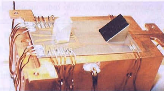
Figure 2-3: A photo image of the 5 cm by 2 cm atom chip glued onto a copper holder. The two cubes on top on the chip surface are the prism mirrors [27].
