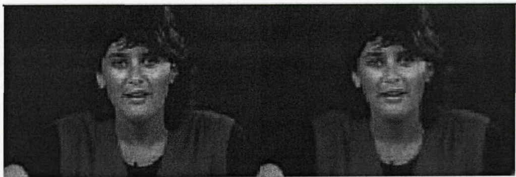
Figure 2.14: Subjective video quality of frame 4 at 2279 bits/frame encoded by the Dirac video codec using the (144x176)-pixel QCIF “Miss_America” sequence.
