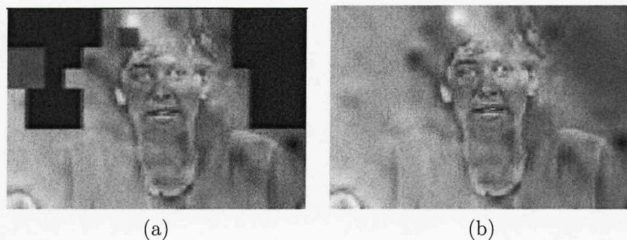
Figure 3.9: Image quality degradation due to the corruption of the Y component's first bit in the lowest LL subband (a) and the resultant motion-predicted second frame (b) for the "Miss_America" QCIF video sequence encoded at 30 frame/s and 60kbit/s using 2181 bits for this frame.
