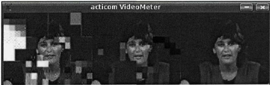
Figure 4.11: Subjective video quality of the systems summarized in Table 4.5 for transmission over the uncorrelated Rayleigh fading channel at E_b/N_0 = 4.5dB : the second video frame of the “Miss_America” sequence extracted from System 1 (left); System 2 (middle); System 3 (right).
