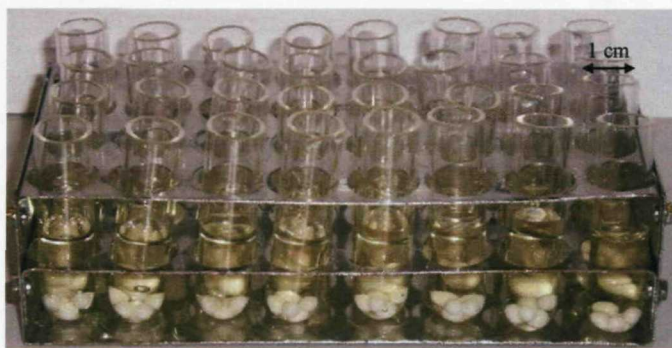
Figure 3-7 Photo of one of the two stainless steel racks used to contain the quartz tubes of the array during heat treatment.
