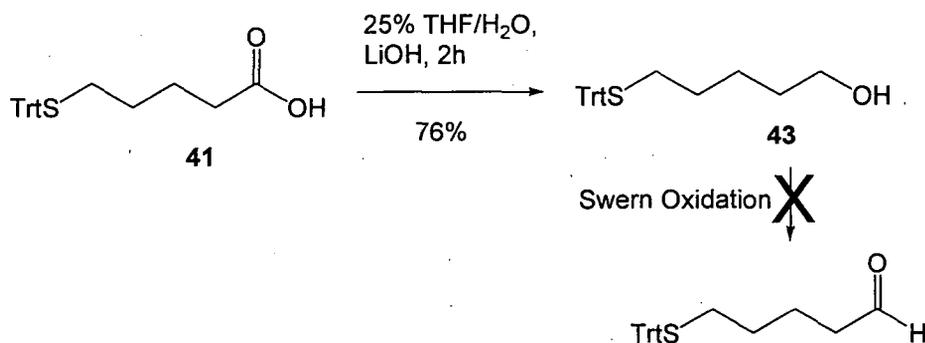
**Scheme 25:** Reaction scheme showing the attempt to synthesise the saturated linker by over reduction and oxidation.
