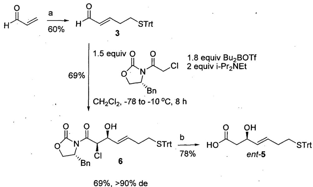
**Scheme 3:** The Wentworth-Janda route to the  $\beta$ -hydroxy acid. Reagents and conditions: a) i. 0.7 equiv TrtSH, 0.7 equiv  $\text{Et}_3\text{N}$ ,  $\text{CH}_2\text{Cl}_2$ , 1 h; ii.  $\text{Ph}_3\text{P}=\text{CH}-\text{CHO}$ , benzene, reflux 7 h. b) i. Al amalgam, aq THF, 0 °C, 2 h; ii. aq  $\text{LiOH}/\text{H}_2\text{O}_2$  in THF, 1 h.
