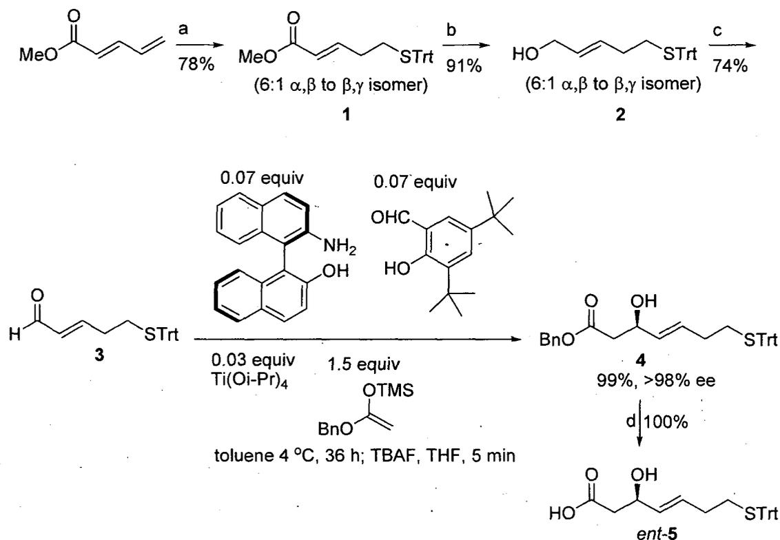
**Scheme 2:** Simon's route to the  $\beta$ -hydroxy acid. Reagents and conditions: a) 1.2 equiv TrtSH, 1.2 equiv  $\text{Cs}_2\text{CO}_3$ , THF, 20 h. b) 2 equiv DIBAL,  $\text{CH}_2\text{Cl}_2$ ,  $-78\text{ }^\circ\text{C}$ , 3 h. c) 1.2 equiv  $(\text{COCl})_2$ , 2.4 equiv DMSO,  $\text{CH}_2\text{Cl}_2$ ,  $-78\text{ }^\circ\text{C}$ , 30 min; 2.4 equiv  $\text{Et}_3\text{N}$ ,  $-30\text{ }^\circ\text{C}$ , 4 h. d) 10 equiv LiOH, MeOH, 3 h.
