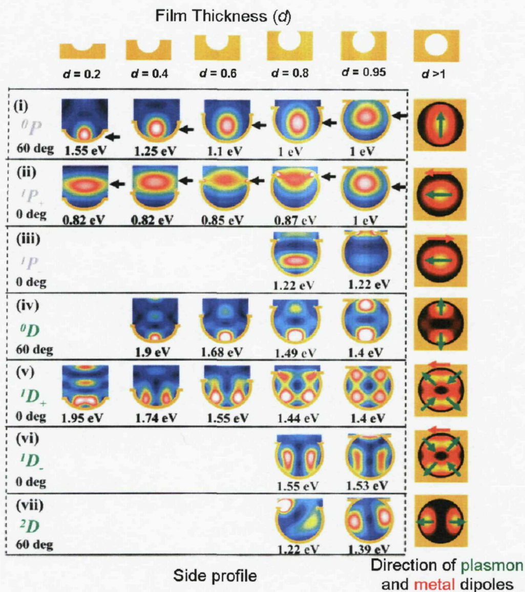
Figure 19 Theoretical plasmon modes within a 500 nm sample. The film thickness ( d ) is indicated at the top of each column, and the theoretical molecular orbital is given for each row. The column for film thickness d > 1 shows the overall direction of the dipole within the metal (red arrows) and the void itself (green arrows). [14]
