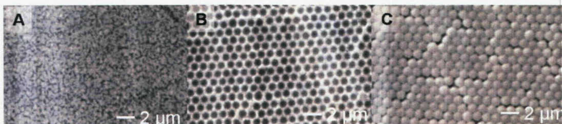
Figure 11 Scanning electron microscope images of an electrochemically roughened surface (A), an anti-dot ( 600 \text{ nm } \frac{3}{4} d ) (B) and a dot MFON type substrate (C) (prepared using a 600 nm polystyrene sphere template with a 150 nm layer of silver evaporated over the surface.) The images were obtained using a Philips XL30 ESEM, with an accelerating voltage of 30 kV and a magnification of 10,000.
