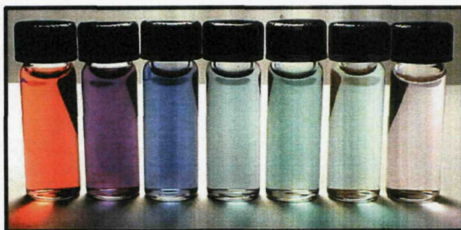
Figure 8 Solution of Ag nano-shell particles from [21], increasing the shell thickness (left to right) alters the surface plasmon energy to longer wavelengths and changes the scattering efficiency.
