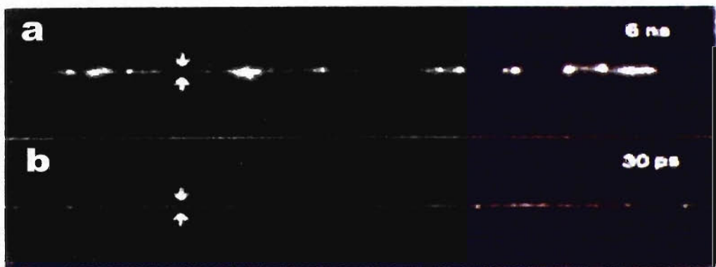
Figure 1.2 Formation of multiple small plasmas (seen as bright spots) at small focussing angles for 6 ns pulse (a) and 30 ps pulse (b). For the 6 ns pulse the focussing angle was 1.8^\circ and for the 30 ps pulse 1.7^\circ . The focal spot is indicated by arrows [35].
