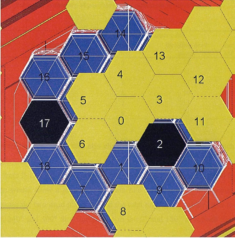
Figure 4.16: Position of the SPI mask with respect to the SPI detector plane at an off axis angle consistent with that of GRB041219a. The black pixels are the two pixels that have failed in SPI.
