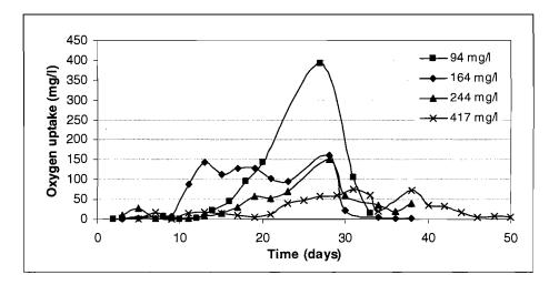
Figure 5.59 Oxygen uptake curves for different initial substrate concentrations
