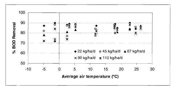
Figure 5.61 BOD<sub>5</sub> removal as a function of temperature in Fayette ponds (Neel *et al.*, 1961)
