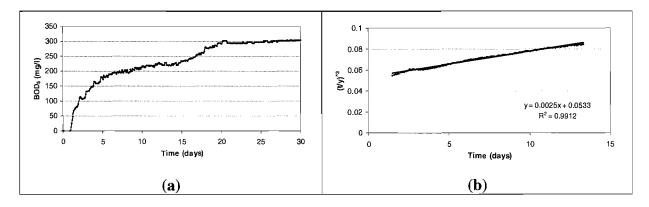
**Figure 4.3** (a) OECD BOD curve and (b) determination of the BOD constant and ultimate BOD using the Thomas graphical method
