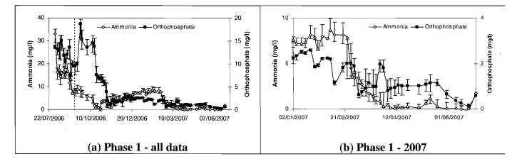
**Figure 7.22** Ammonia and orthophosphate concentration during Phase 1 (NB. different y-axis to highlight changes in nutrients in spring) (---) represents end of filling period
