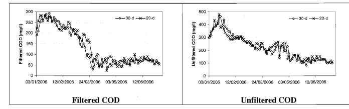
Figure 6.25 Change in mean filtered and unfiltered COD concentration for 20- and 30-d HRT (NB. different y-axis)
