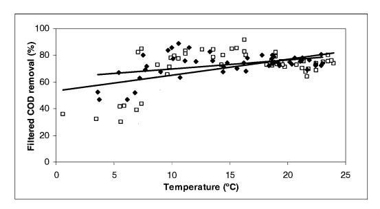
Figure 6.27 Relationship between filtered COD removal and water temperature in facultative tanks with 20- and 30-d HRT (♦) 30-d HRT (R<sup>2</sup> = 0.19); (□) 20-d HRT (R<sup>2</sup> = 0.25)
