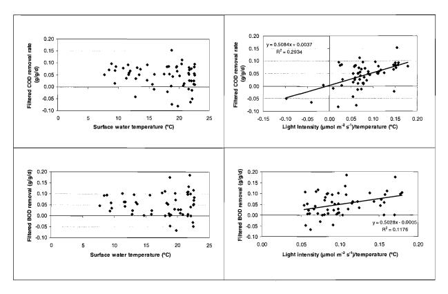
Figure 5.46 COD and BOD<sub>5</sub> removal rate and temperature and temperature with light intensity during tank experiments
