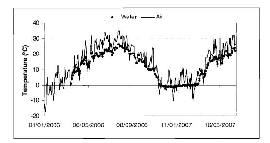
Figure 6.5 Air and average surface water temperature in the 780 l tanks
