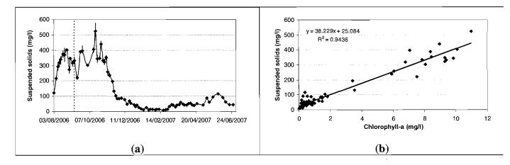
**Figure 7.20** (a) Suspended solids and (b) relationship between chlorophyll-a and suspended solids concentration during Phase 1 (Filling period not included) (---) represents end of filling period
