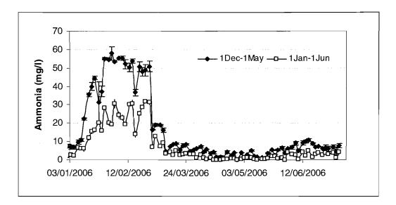
Figure 6.42 Ammonia concentration in storage maturation tanks with different storage periods and discharge dates
