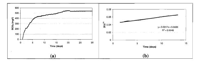
**Figure 4.1** (a) Synthetic BOD curve and (b) determination of the BOD constant and ultimate BOD using the Thomas graphical method
