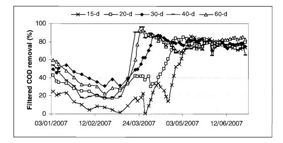
Figure 6.33 Change in filtered COD removal efficiency over time in facultative tanks with different HRT
