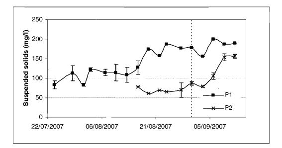
Figure 7.33 Suspended solids concentration in both ponds during Phase 2
