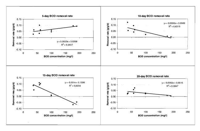
Figure 5.42 5, 10, 15 and 20-day filtered BOD<sub>5</sub> removal rates for initial BOD<sub>5</sub> concentration
