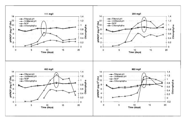
Figure 5.23 Changes in filtered and unfiltered pH in response to rises in chlorophyll-a and net oxygen production  $\bigcirc = \text{ where unfiltered pH became higher than filtered pH}$
