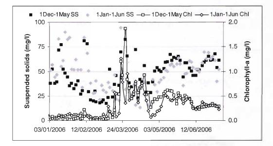
Figure 6.41 Chlorophyll-a and suspended solids concentration in storage maturation tanks with different storage periods and discharge dates
