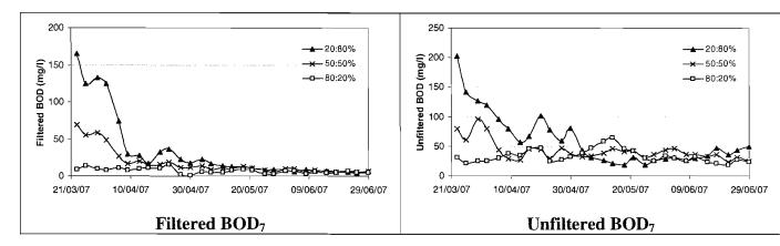
Figure 6.16 Change in mean filtered and unfiltered BOD<sub>7</sub> concentration over time for each dilution (NB. different y-axis)
