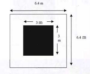
Figure 7.2 Dimensions of Pond 1
