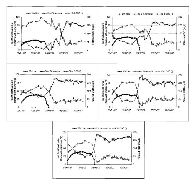
remaining COD continued in the period immediately after ice melt, making it difficult to distinguish between the periods of partial ice cover and completely open water.
