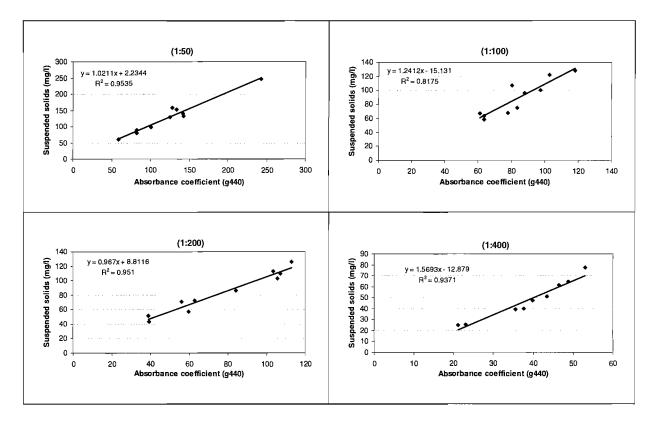
Figure 5.18 Relationship between unfiltered absorbance at 440 nm and suspended solids for each initial COD concentration
