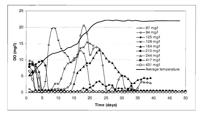
Figure 5.54 Change in surface dissolved oxygen levels for each initial COD concentration (same symbols represent the same run; open symbols represent tank 1; closed symbols tank 2)
