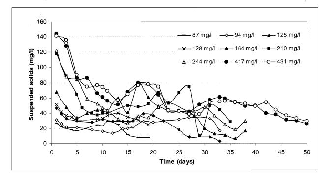
**Figure 5.50** Change in suspended solids concentrations over time for each initial substrate concentration (same symbols represent the same run; open symbols represent tank 1; closed symbols tank 2)
