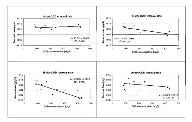
Figure 5.40 5, 10, 15 and 20-day filtered COD removal rates for each initial COD concentration
