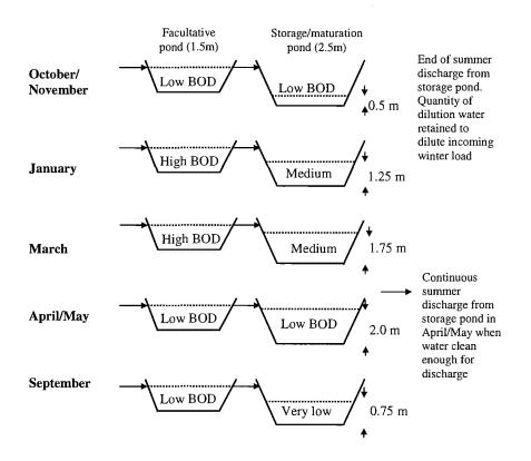
Figure 8.1 Schematic of the proposed operational design for WSP in cold regions (adapted from Heaven and Banks (2005))
