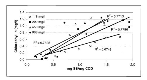
**Figure 5.17** Relationship between mean chlorophyll-a levels and ratio of suspended solids to COD concentration
