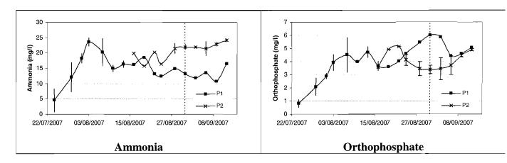
Figure 7.35 Ammonia and orthophosphate concentration in each pond during Phase 2 (NB. different y-axis)
