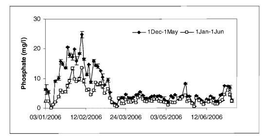
Figure 6.43 Phosphate concentration in storage maturation tanks with different storage periods and discharge dates
