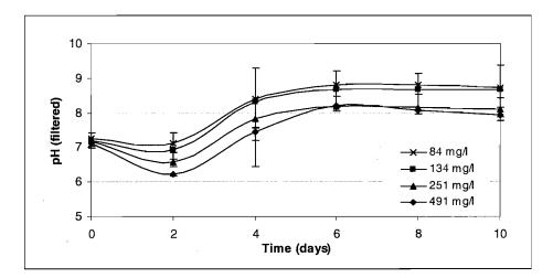
Figure 5.5 Change in mean filtered pH values over time for each initial COD concentration
