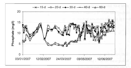
Figure 6.39 Change in phosphate concentration over time in facultative tanks with different HRT
