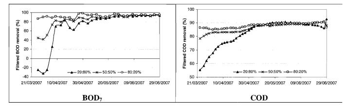
Figure 6.17 Filtered BOD<sub>7</sub> and COD removal efficiency for each dilution (NB. different y-axis)
