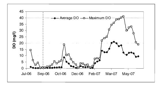
Figure 7.24 Weekly average and maximum dissolved oxygen levels during Phase 1 (---) represents end of filling period
