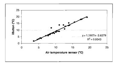
Figure 7.9 Relationship between the air temperature sensor and iButton readings (weekly average readings November-June)
