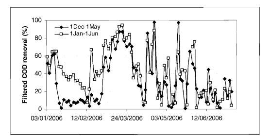
**Figure 6.40** Change in filtered COD removal efficiency in storage maturation tanks with different storage periods and discharge dates
