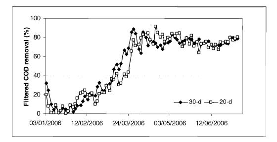
Figure 6.26 Filtered COD removal in facultative tanks with 20- and 30-d HRT
