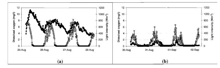
Figure 7.39 Relationship between light intensity and dissolved oxygen levels in Pond 2 (♦) dissolved oxygen; (□) light intensity
