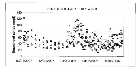
Figure 6.37 Change in suspended solids concentration over time in facultative tanks with different HRT
