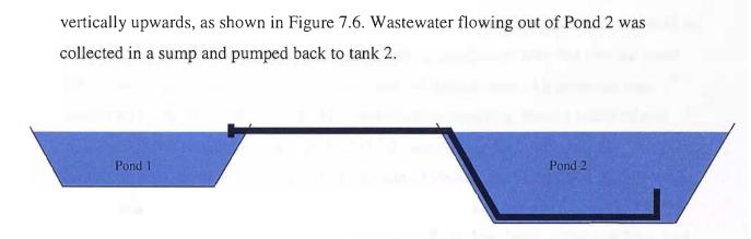
Figure 7.6 Pipework connecting Pond 1 and Pond 2
