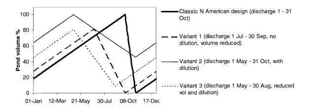
Figure 6.1 Simplified flow balance model with alternative time-dependent discharge and effluent retention scenarios
