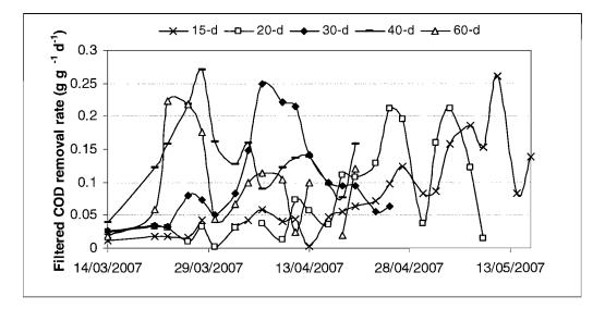
Figure 6.34 Change in filtered COD removal rate over time in facultative tanks with different HRT
