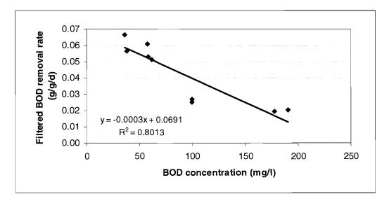
Figure 5.43 Overall BOD<sub>5</sub> removal rate for each initial BOD<sub>5</sub> concentration
