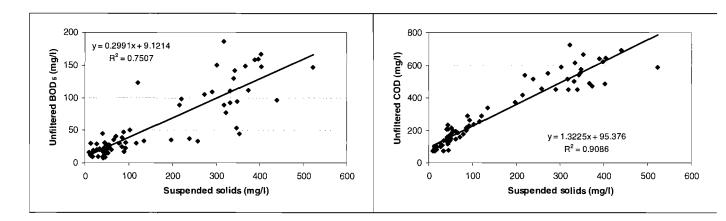
Figure 7.21 Relationship between suspended solids and BOD<sub>5</sub>/COD concentration during Phase 1 (NB. different unit of measurement)
