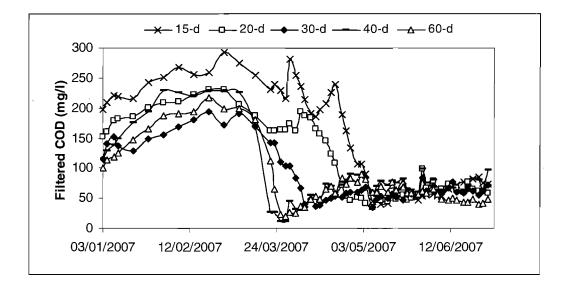
Figure 6.32 Change in filtered COD concentration over time in facultative tanks with different HRT
