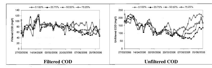
**Figure 6.6** Mean changes in filtered and unfiltered COD concentration over time for each dilution (NB. different y-axis)
