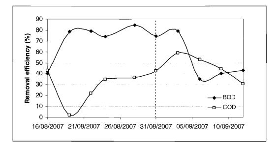
Figure 7.31 Average filtered BOD<sub>5</sub> and COD removal efficiencies in Pond 2 during Phase 2
