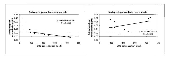
Figure 5.53 5 and 10-day orthophosphate removal rate for each initial COD concentration
