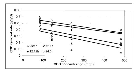
Figure 5.30 COD removal rate at different initial COD concentrations for each daylength on day 2 (with regression lines)
