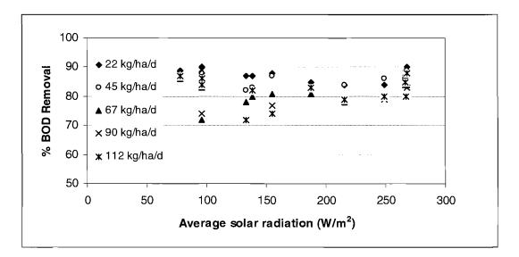
Figure 5.60 BOD<sub>5</sub> removal as a function of light intensity in Fayette ponds (Neel *et al.*, 1961)
