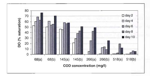
Figure 5.10 Change in dissolved oxygen levels for different initial COD concentrations in the dark variant bottles ( $^{a}15 \ \mu mol \ m^{-2} \ s^{-1}$ ;  $^{b}5 \ \mu mol \ m^{-2} \ s^{-1}$ )
