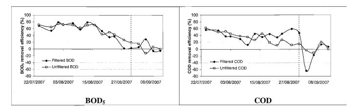
Figure 7.30 Average filtered and unfiltered BOD<sub>5</sub> and COD removal efficiencies in Pond 1 during Phase 2
