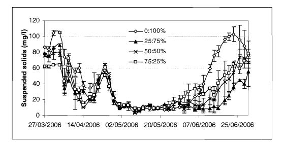
Figure 6.9 Change in suspended solids concentrations over time for each dilution
