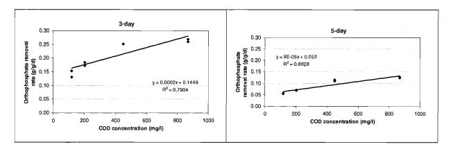
Figure 5.25 3 and 5-day orthophosphate removal rate
