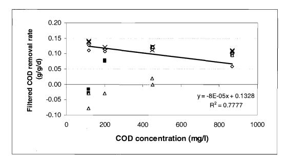
Figure 5.12 5-d (×), 10-d ( $\blacksquare$ ), 15-d ( $\triangle$ ) and overall ( $\Diamond$ ) COD removal rate (with regression line)
