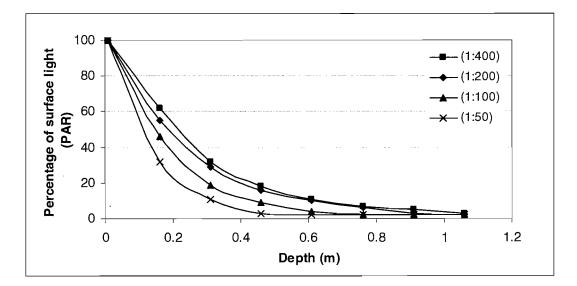
Figure 5.44 Percentage transmission of incident light with depth in the tanks in relation to dilution
