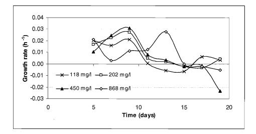
Figure 5.14 Effect of mean initial concentration on algal growth rate
