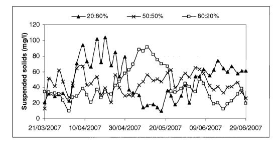
Figure 6.19 Change in suspended solids concentration over time for each dilution
