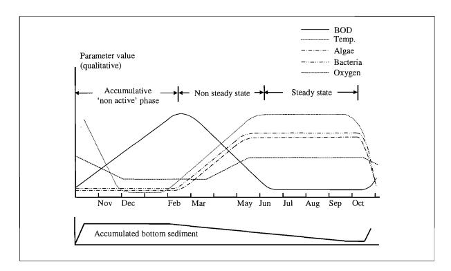
**Figure 2.1** Seasonal fluctuations in key parameters in a variable climate pond in the northern hemisphere working in batch mode with a once-yearly discharge (Heaven and Banks, 2005)
