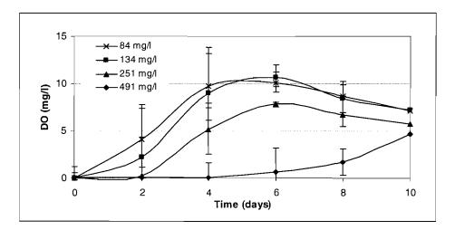
Figure 5.6 Change in mean dissolved oxygen levels over time for each initial COD concentration (with range bars)
