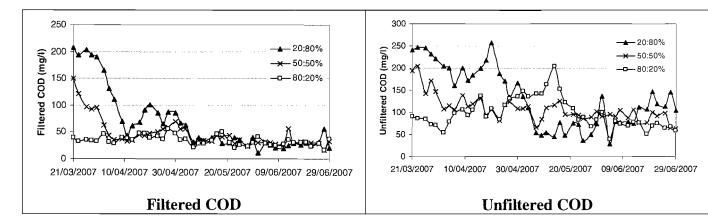
Figure 6.15 Change in mean filtered and unfiltered COD concentration over time for each dilution (NB. different y-axis)
