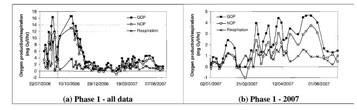
**Figure 7.27** Average gross and net oxygen production and respiration rate during Phase 1 (NB. different y-axis to highlight changes in oxygen production) (---) end of filling period
