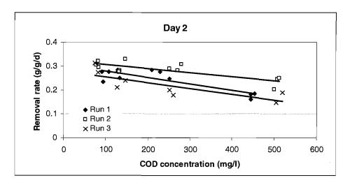
**Figure 5.3** COD removal rate in all bottles on day 2 for each run (with regression lines)
