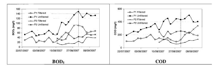
**Figure 7.29** Average filtered and unfiltered BOD<sub>5</sub> and COD concentration in both ponds during Phase 2 (using both composite and grab samples) (---) represents end of filling period
