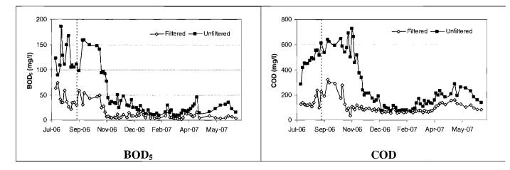
Figure 7.18 Monthly average filtered and unfiltered BOD<sub>5</sub> and COD concentration during Phase 1 (---) represents end of filling period
