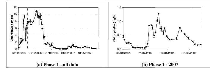
**Figure 7.19** Chlorophyll-a concentration during Phase 1 (2007 graph shows spring algal bloom) (NB. different y-axis to highlight changes in chlorophyll-a concentration) (---) represents end of filling period
