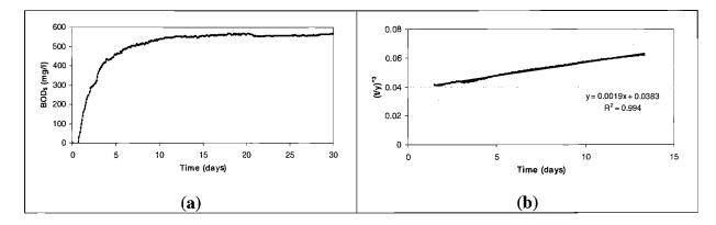
**Figure 4.2** (a) SYNTHES BOD curve and (b) determination of the BOD constant and ultimate BOD using the Thomas graphical method
