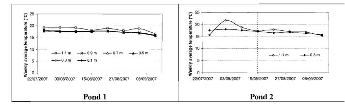
**Figure 7.15** Weekly average water temperature for both ponds during Phase 2 (---) represents pond at maximum volume
