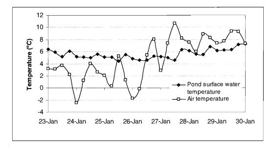
Figure 7.14 Air temperature and surface water temperature readings during one week in January in 2007 (average taken over six-hour period)
