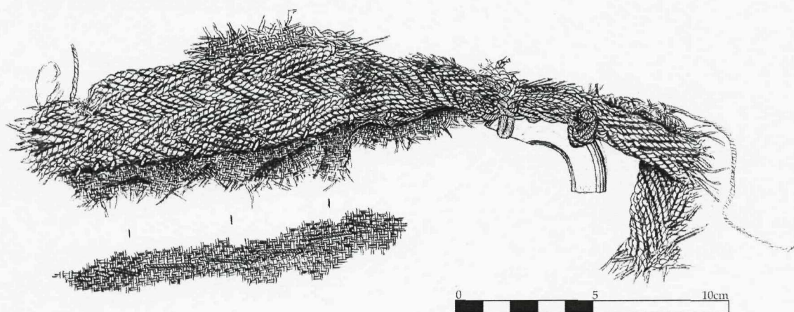
Fragment of cotton sailcloth, horizontal reinforcement strip and attached wooden brail ring from the Red Sea port of Myos Hormos (J. Whitewright).
