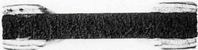
Figure 5- 1 Tapered wooden end tabs shown adhered to an unaged C70.130
