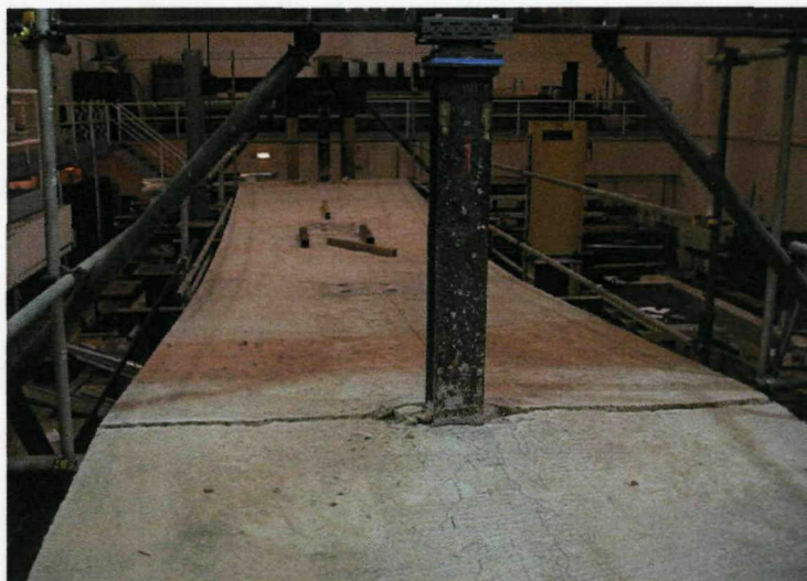
Fig. 3. 24 Crack in composite slab that led to fracture of mesh reinforcement (Byfield, 2004)
