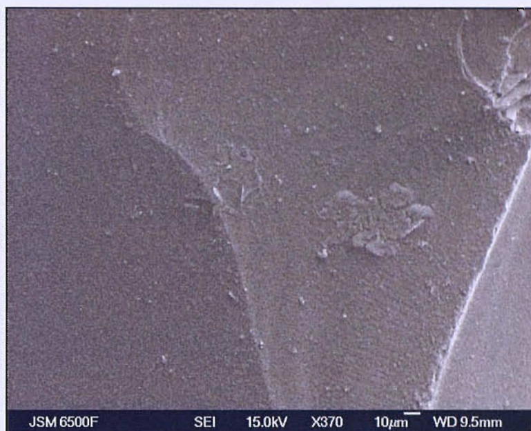
Figure 5.7: SEM image confirming the coating of the substrate via the presence of imperfections in the film (see centre of image).
