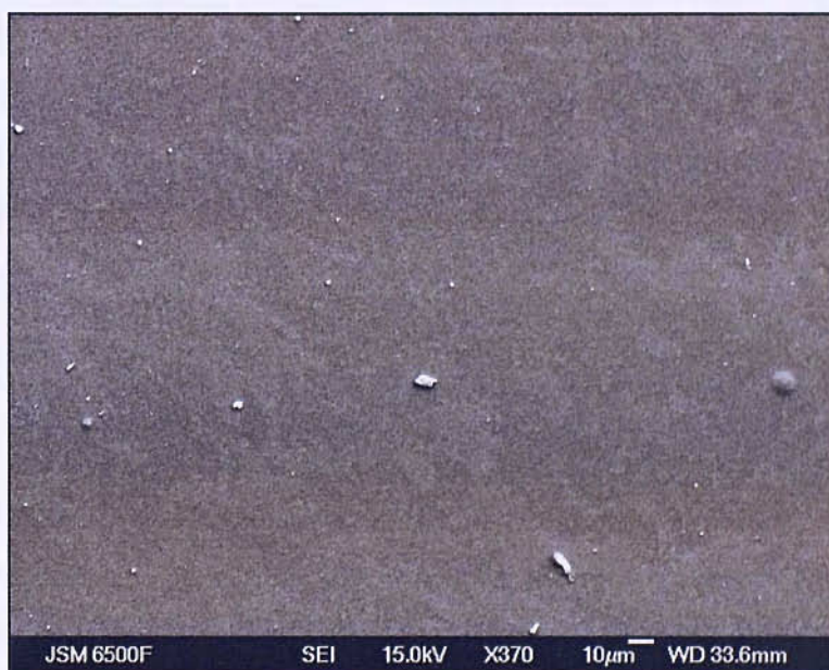
Figure 5.6: Ammonolytic coating, on silica, with no cracks but some solid fragments.
