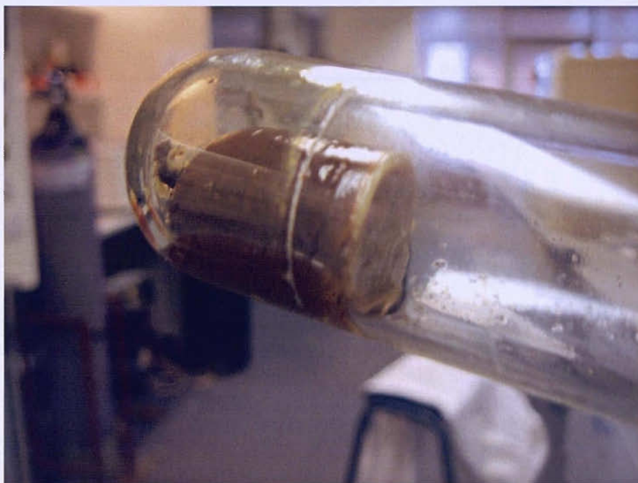
Figure 6.2: Image of TiN precursor gel after solvent removal, clearly displaying the same shape as the containing vessel.
