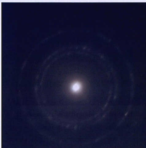
Figure 3.20: A diffuse electron diffraction pattern of the TiN precursor after annealing at 450 °C under N 2 .
