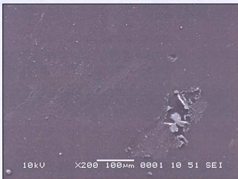
Figure 5.11: The occasional presence of imperfection confirmed that a coating was present.
