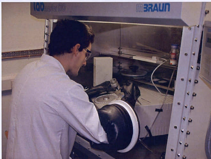
Figure 2.11: Mettler Toledo TGA851e being used inside a nitrogen-filled glovebox.
