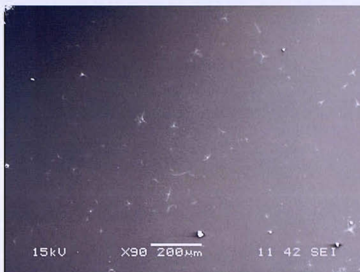
Figure 4.5: SEM images of films produced with \text{PrNH}_2 and \text{Ti}(\text{NMe}_2)_4 solutions, made with 20 \text{ cm}^3 (Top), 10 \text{ cm}^3 (Middle) or 5 \text{ cm}^3 (Bottom) THF and then pyrolysed in \text{N}_2 at 800 \text{ }^\circ\text{C} .
