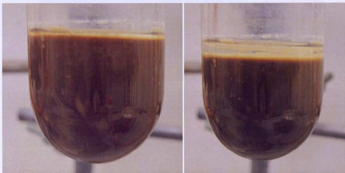
Figure 6.1: Images displaying the process of syneresis in the tin precursor gel after 24 hours (left) and 48 hours (right).
