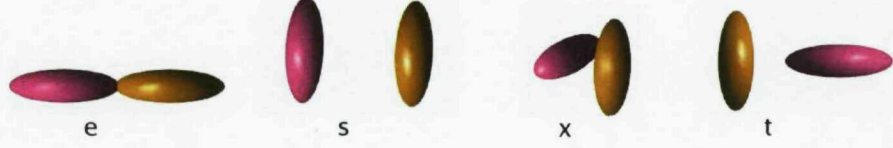
Figure 5.3: Representative configurations of a pair of Gay-Berne particles. From left to right: end-to-end e , side-by-side s , cross x and tee t .
