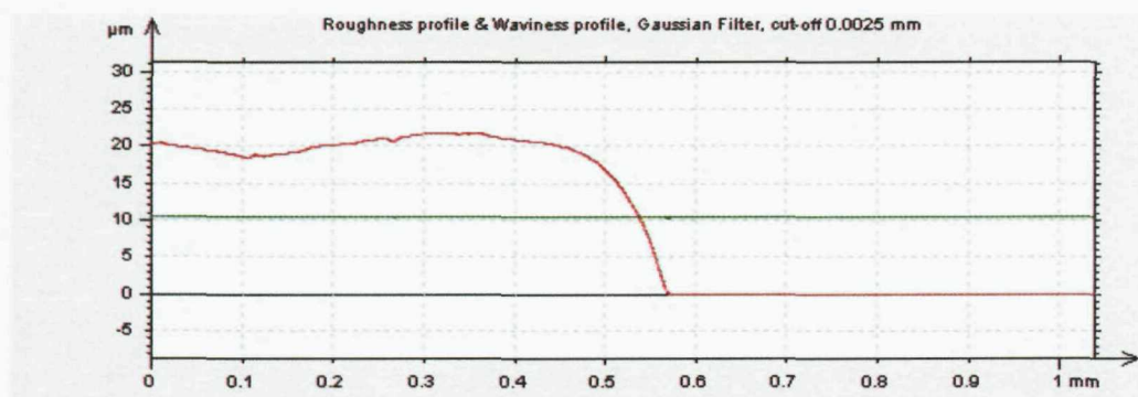
Figure 12: The TiO 2 film profile ( red trace ) at its edge with the TCO substrate measured for a film prepared using Paste 2 and a 43 thread/cm screen.
