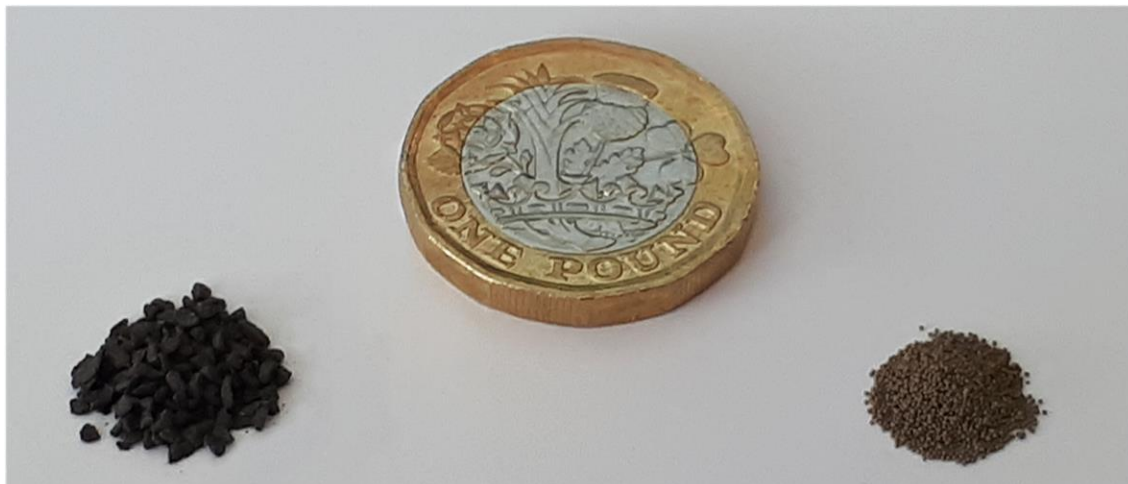
Figure 6.13 – A photograph for comparison of the variant (left) and baseline (right) catalysts.
