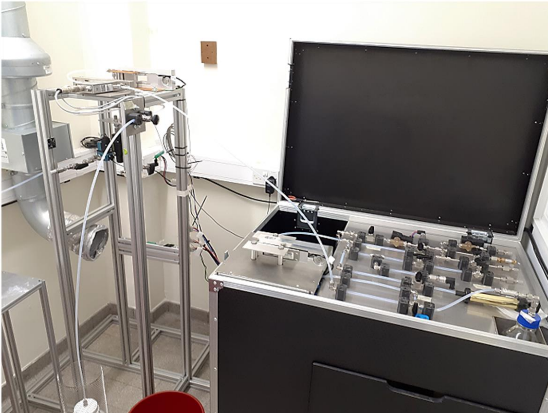
Figure 3.1 – A photograph of the chemical micropropulsion laboratory fluidic system, showing the thrust stand (downstream of MV5) on the left and the rest of the system on the right.
