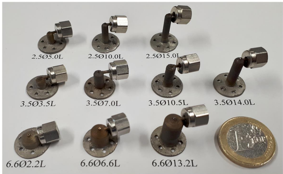
Figure 6.1 – A photograph of all of the manufactured thruster variations, labelled with their corresponding notation. A 1 EUR coin is included for scale.
