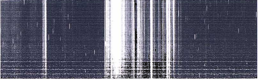
Figure 3.2: An example keogram, for the period 15 UT - 21 UT (l - r) on 26 January 2006. This shows data from the O^+ 7320/30 Å doublet mosaic panel. The bright areas mainly in the centre of the keogram are aurora, and the shorter bright vertical lines are stars.
