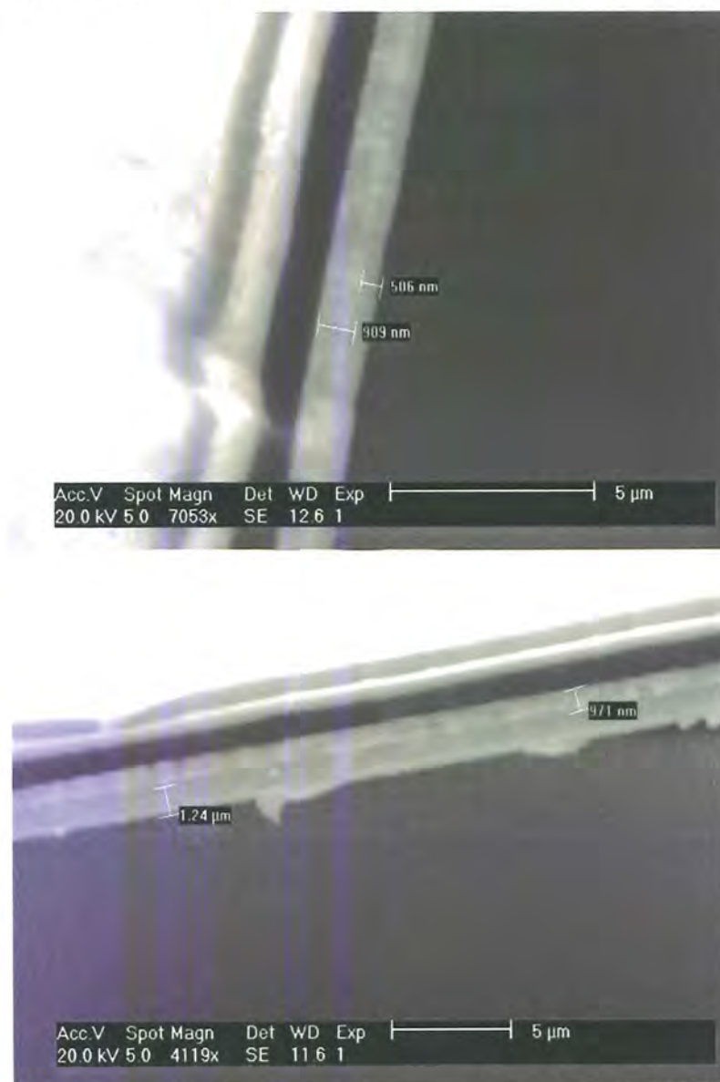
Figure 3.2.1: SEM micrographs of the 1 dip (top) and 4 dip (bottom) TiO 2 films coated on FTO glass.
