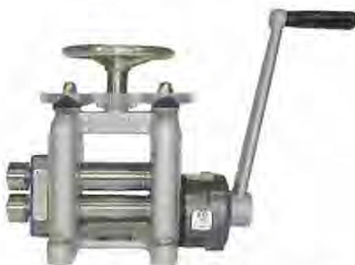
Figure 5.3.1: A Durston Minimill, as used for milling composite electrode films.[123]
