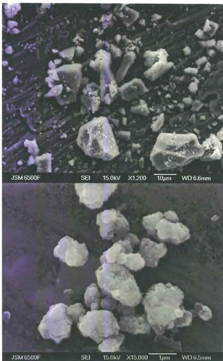
Figure 3.2.7 SEM micrograph for Titania powder prepared with I 1 F127 (Top) and commercial 12 nm anatase particles (bottom).
