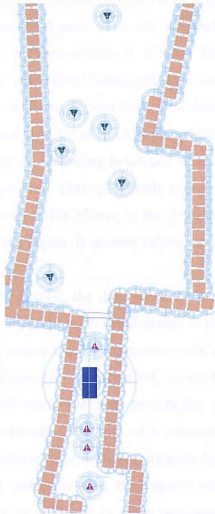
Figure 6-9: The ABM environment: agents moving towards the south are indicated in green and those heading towards the north in red. The blue object stands for group of pedestrians, pack or ridden animals. Forces of avoidance (hard and repel radii) are indicated with light blue.
