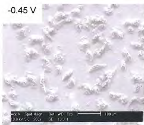
Fig. 3.10 SEM micrograph of the film deposited at -0.45 V vs. SCE. Scale bar is 100 \mu\text{m}
