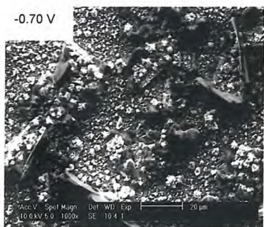
Fig. 3.33 SEM micrograph of the film deposited at -0.70 V vs. SCE. Scale bar is 20 \mu\text{m} .
