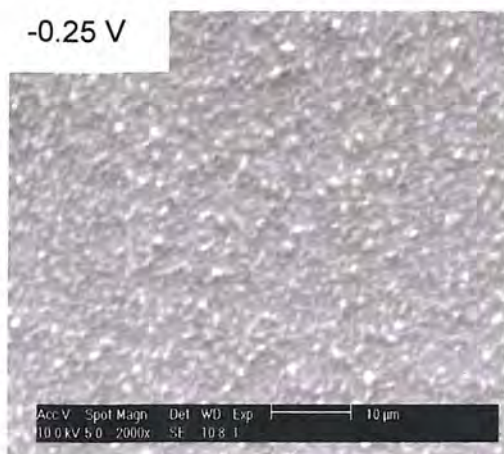
Fig. 3.8 SEM micrograph of the film deposited at -0.25 V vs. SCE. Scale bar is 10 \mu\text{m}
