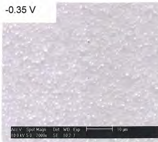
Fig. 3.9 SEM micrograph of the film deposited at -0.35 V vs. SCE. Scale bar is 10 \mu\text{m}
