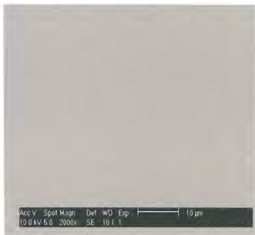
Fig. 4.22 SEM micrograph of the second H_1 -PbTe film using a nucleation pulse. Scale bar is 10 \mu\text{m}
