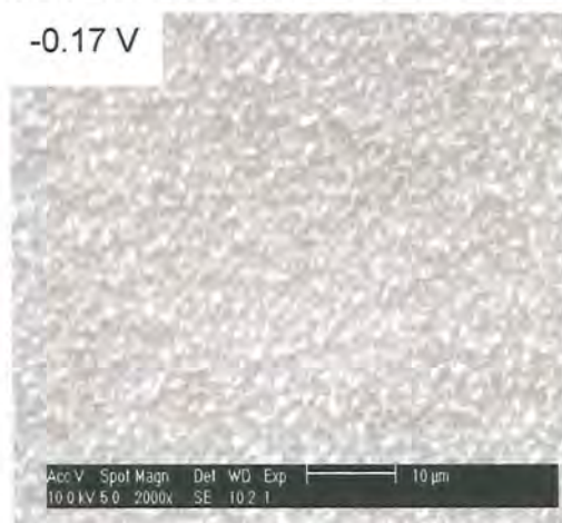
Fig. 3.6 SEM micrograph of the film deposited At -0.17 V vs. SCE. Scale bar is 10\text{ }\mu\text{m}
