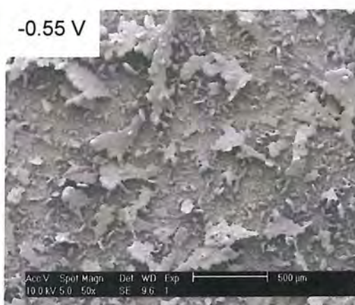
Fig. 3.11 SEM micrograph of the film deposited at -0.55 V vs. SCE. Scale bar is 500 \mu\text{m}
