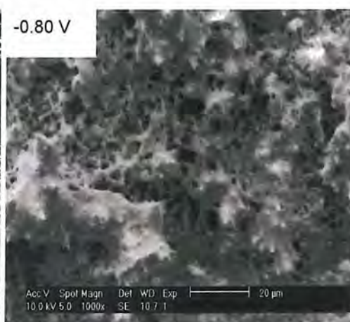
Fig. 3.34 SEM micrograph of the film deposited at -0.80 V vs. SCE. Scale bar is 20 \mu\text{m} .
