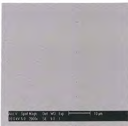
Fig. 3.63 SEM of film deposited after 1 s at -0.60V then deposition at -0.43V for 1 hour.
