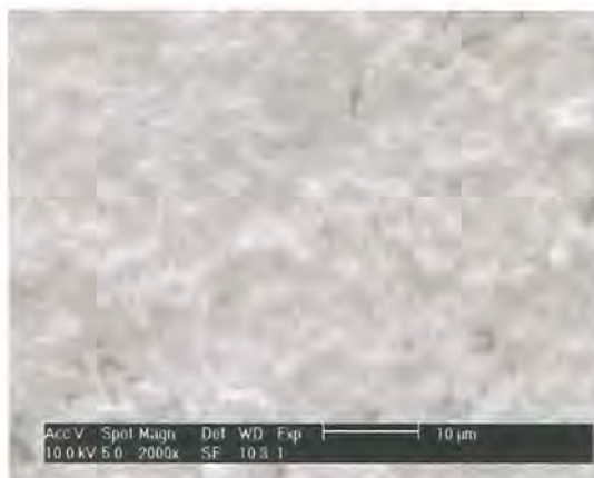
Fig. 4.13 SEM micrograph of the first mesoporous film deposited onto modified silicon substrate. Scale bar is 10 \mu\text{m} .
