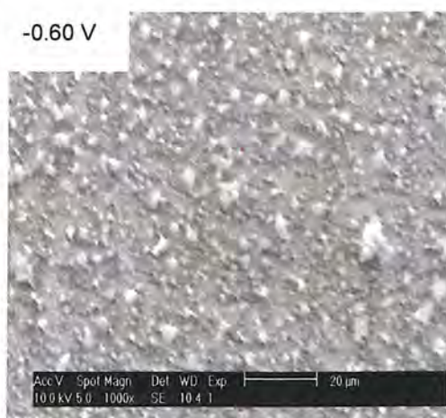
Fig. 3.32 SEM micrograph of the film deposited at -0.60 V vs. SCE. Scale bar is 20 \mu\text{m}
