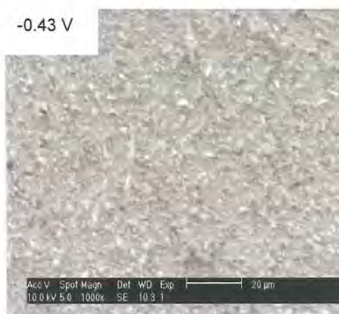
Fig. 3.30 SEM micrograph of the film deposited at -0.43 V vs. SCE. Scale bar is 20 μm
