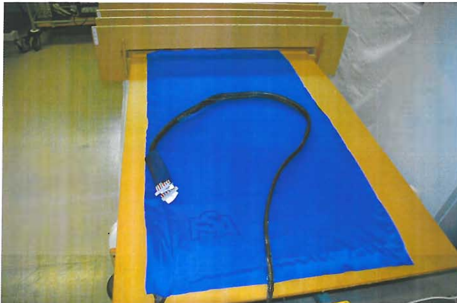
Figure 3.1b Force sensing mat positioned on lower calibration jig platen
