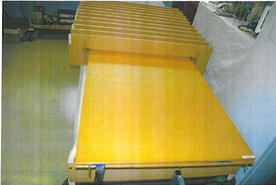
Figure 3.1d Calibration jig showing upper platen in position
