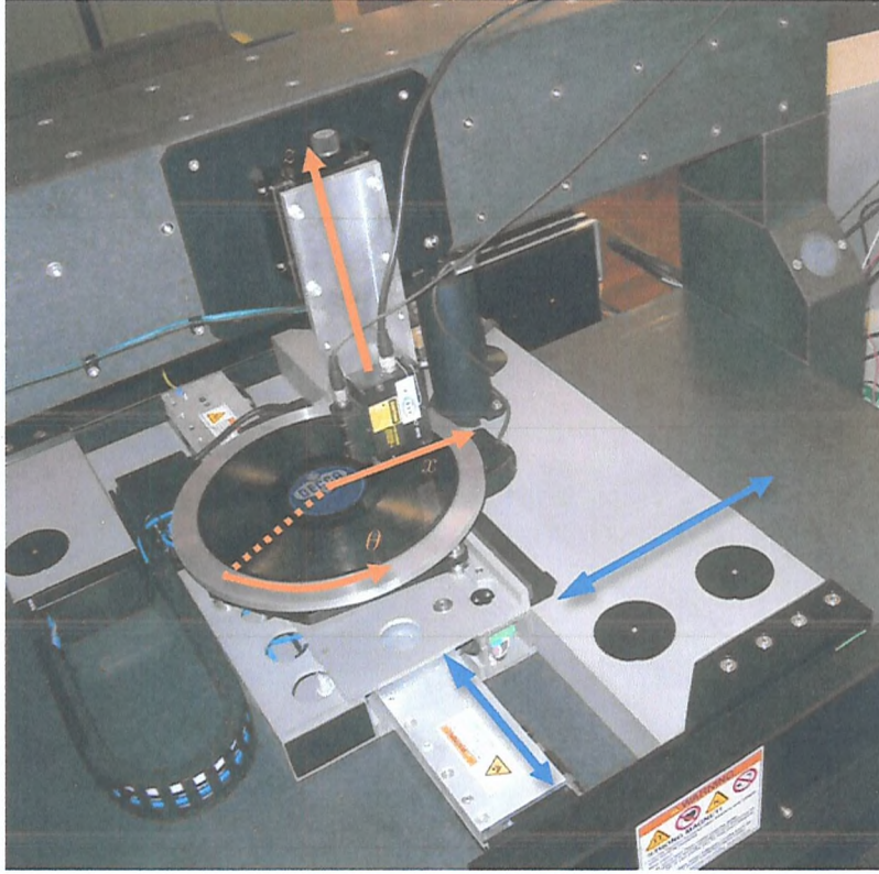
Figure 3.10: Air-bearing system shown here measuring a 78 rpm disc.
