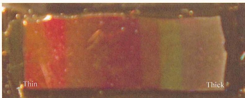
Figure 2.8 A photograph of gold graded substrate with the sphere template still embedded in the structure. The template consists of 600 nm diameter ( D ) spheres. The gradation is from 0.1 to 1 D from left to right in 10 steps of 1 mm each.
