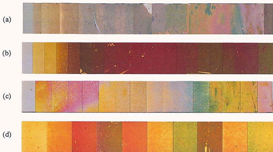
Figure 4.2 Optical images of (a) D400, (b) D800, (c) D900 and (d) D1000 SSV gold substrates. The images show the variation in colour with the thickness of the electrodeposited film. The film thickness increase from 0 to 1 D for (a), 0 to 0.8 D for (b) and (c) and 0.1 to 1 D for (d) in equally spaced steps from left to right. The area of each image is 700 \mu\text{m} x 500 \mu\text{m} .
