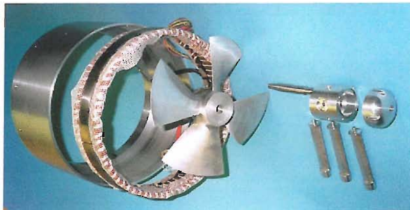
Figure A3.8 – Components used in the prototype TDP. From left to right: Aluminium shroud, stator, propeller, propeller shaft, bearing casing and supports.
