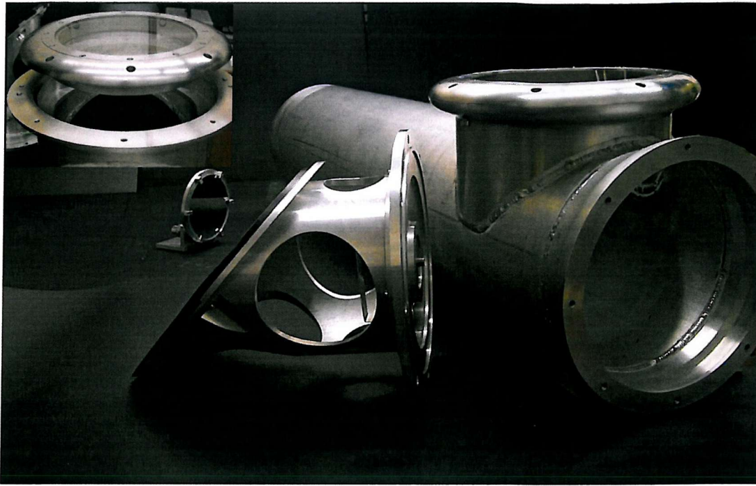
Figure 7. 6. The Laser Scanning Unit submersible housing, showing torpedo structure ( right ), 45° mirror ( foreground left ), plane adjustable mirror ( background ) and glass window and lens assembly ( insert ).
