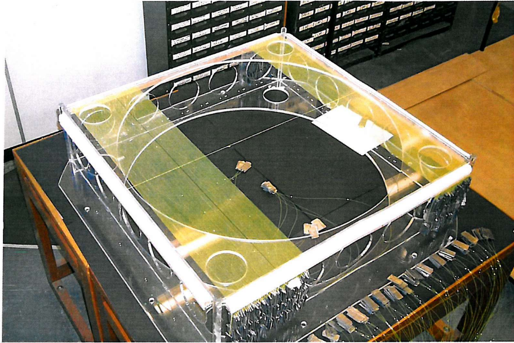
Figure 7.3. A single layer of the detector frame. The fibres are being mounted, using lead to tension them.
