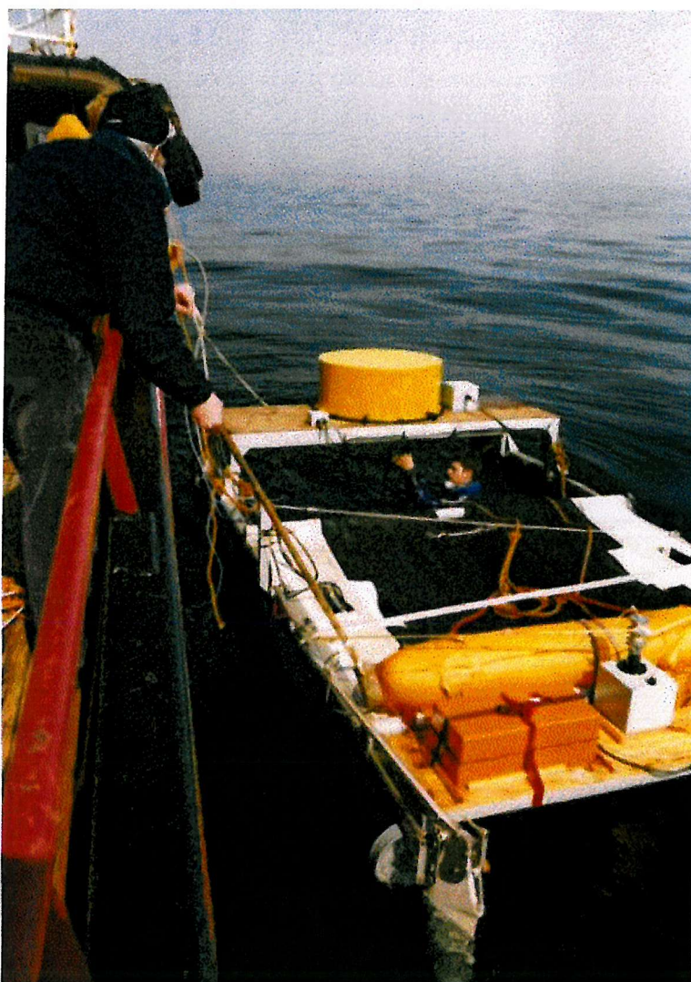
Figure 3. 10. The attachment of the optical fibre, data link cable and the wiping of the detector screen by a diver.
