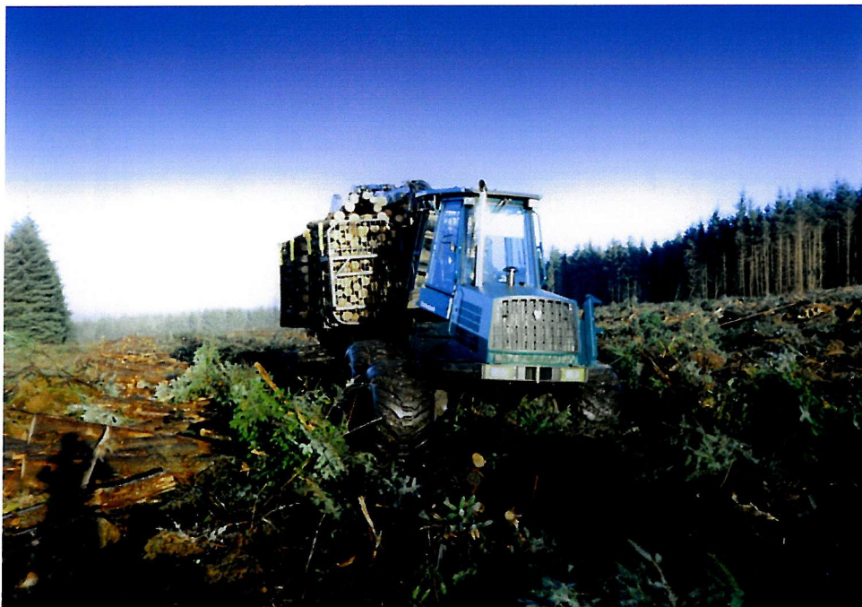
Plate 1.2. Extraction of sawn timber by a forwarder (Kielder Forest, UK) travelling along a brash mat. (Photograph: John Walton).
