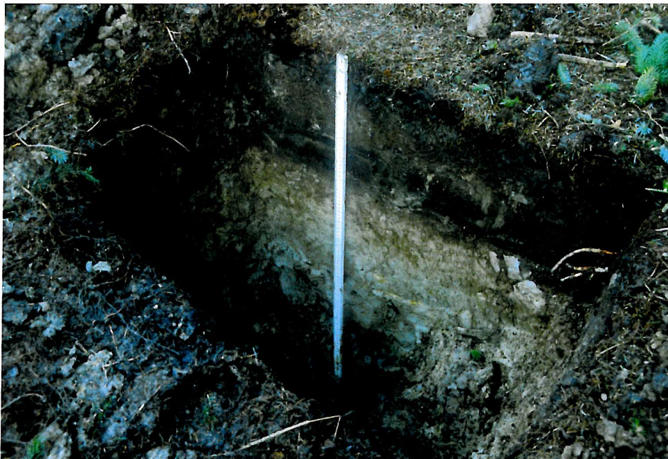
Plate 2.2. Soil profile typical of a peaty gley soil (site 01K). See Box 2.1 (p. 30) for profile description.
