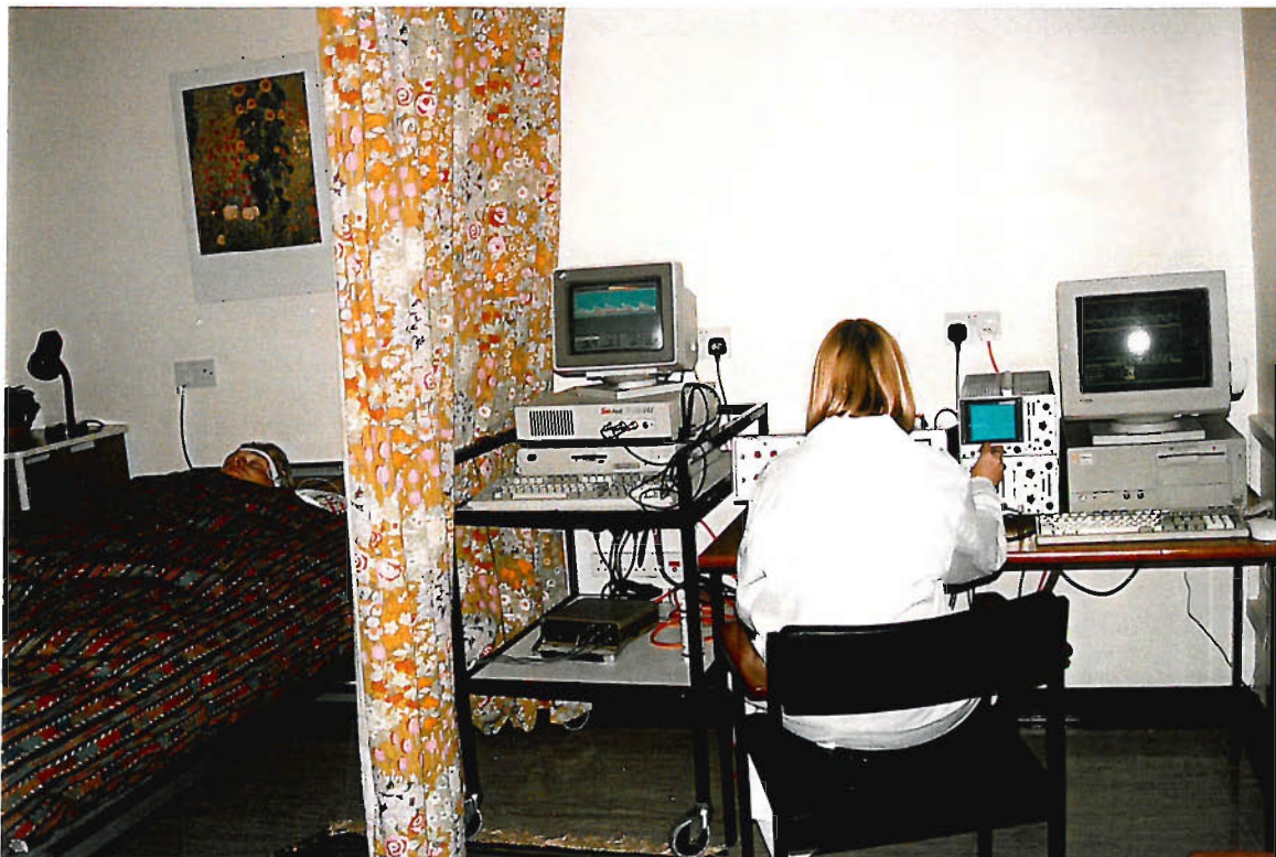
Figure 3: The TCD machine, EEG amplifier, oscilloscope and computer for data acquisition as set-up in the sleep laboratory
