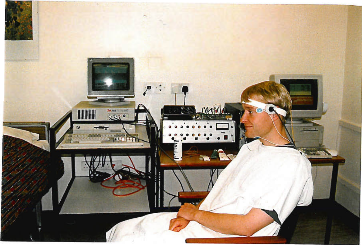
Figure 2: A volunteer with the TCD probe held in position with an elasticated headband and EEG electrodes connected to the junction box
