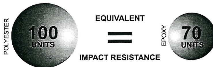
Figure 5.3 Polyester and epoxy resin; E-glass mass requirement for equal impact performance.
