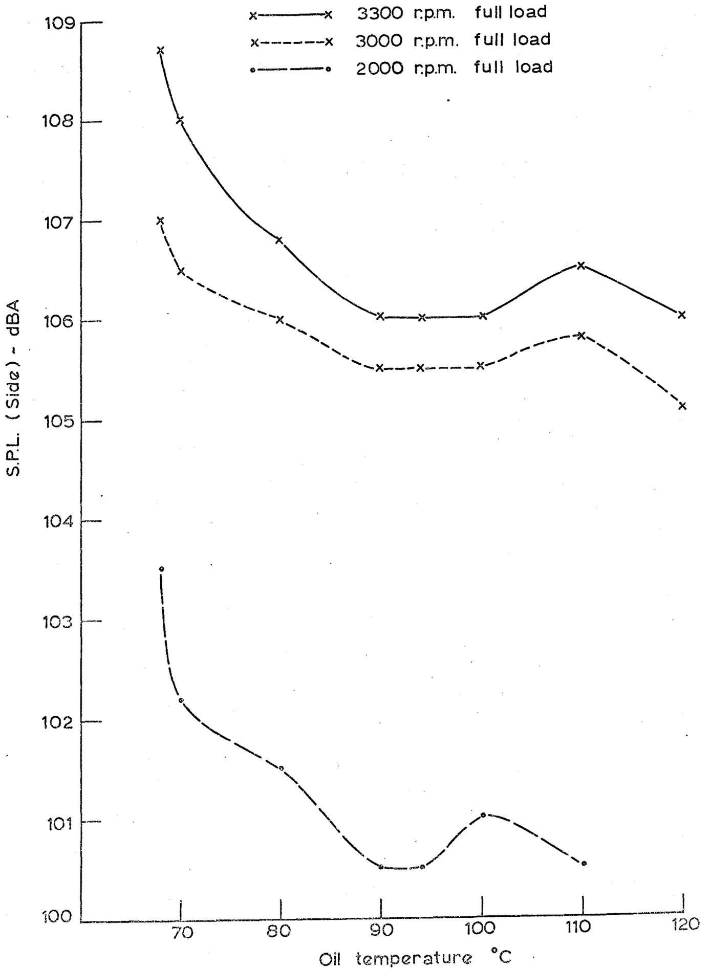
Fig. 3.4 Variation of overall noise levels with oil temperature for the SA engine.
