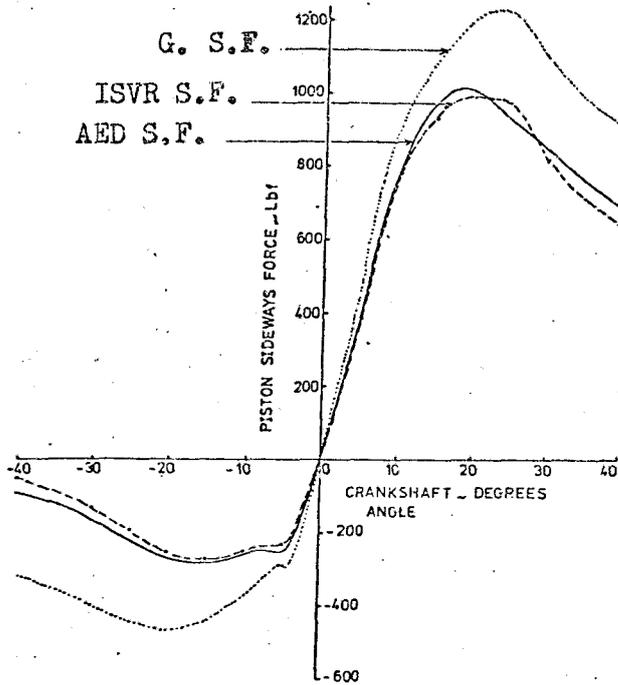
COMPARISON OF COMPUTED PISTON SIDE FORCES AROUND T.D.C. USING ISVR and AED PROGRAMMES AT 3600RPM FULL LOAD (ENGINE SA G.P.OFFSET=0)
