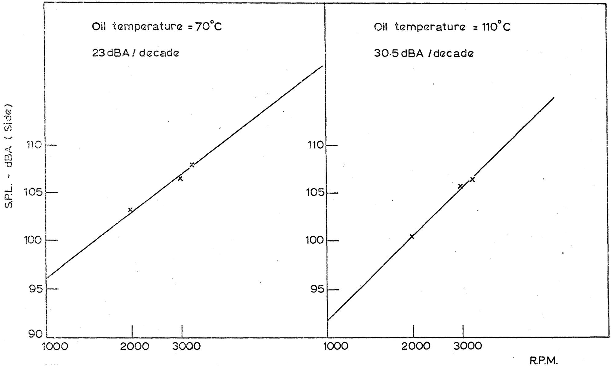
Fig. 3.5 Variation of overall noise levels with speed of the SA engine at full load for 70 and 110°C oil temperature
