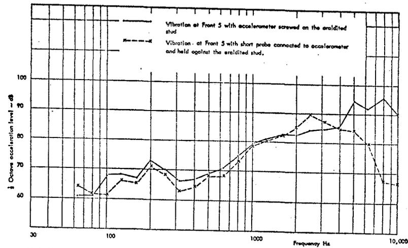
FIG. 3.11b REFERENCE CORRECTION LEVELS FOR SHORT PROBE.
