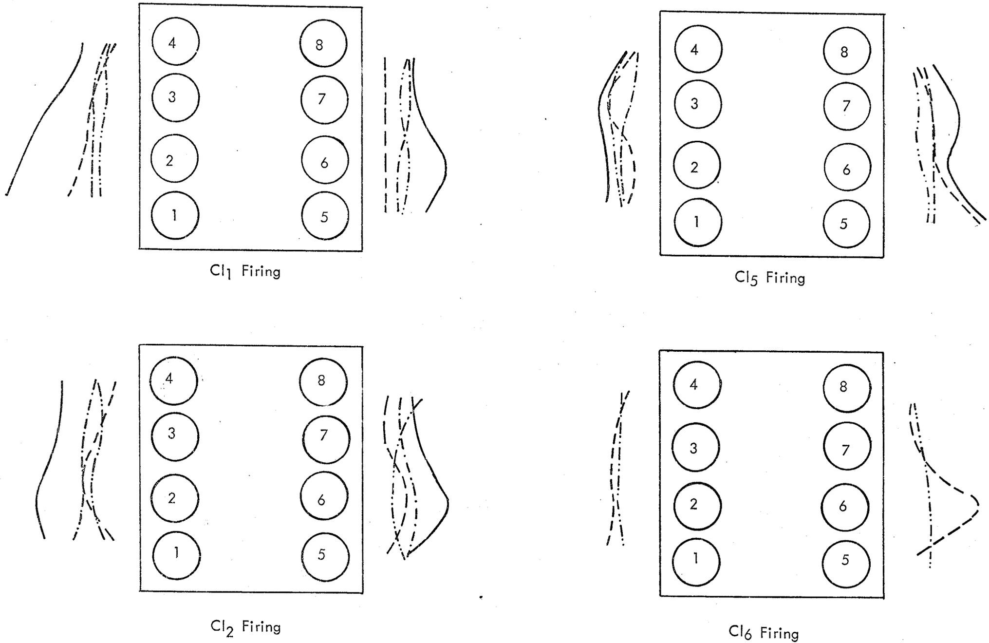
FIG. 4.19 MAXIMUM VIBRATION AMPLITUDES FOR SA ENGINE MAHLE @ 3000 r.p.m.
