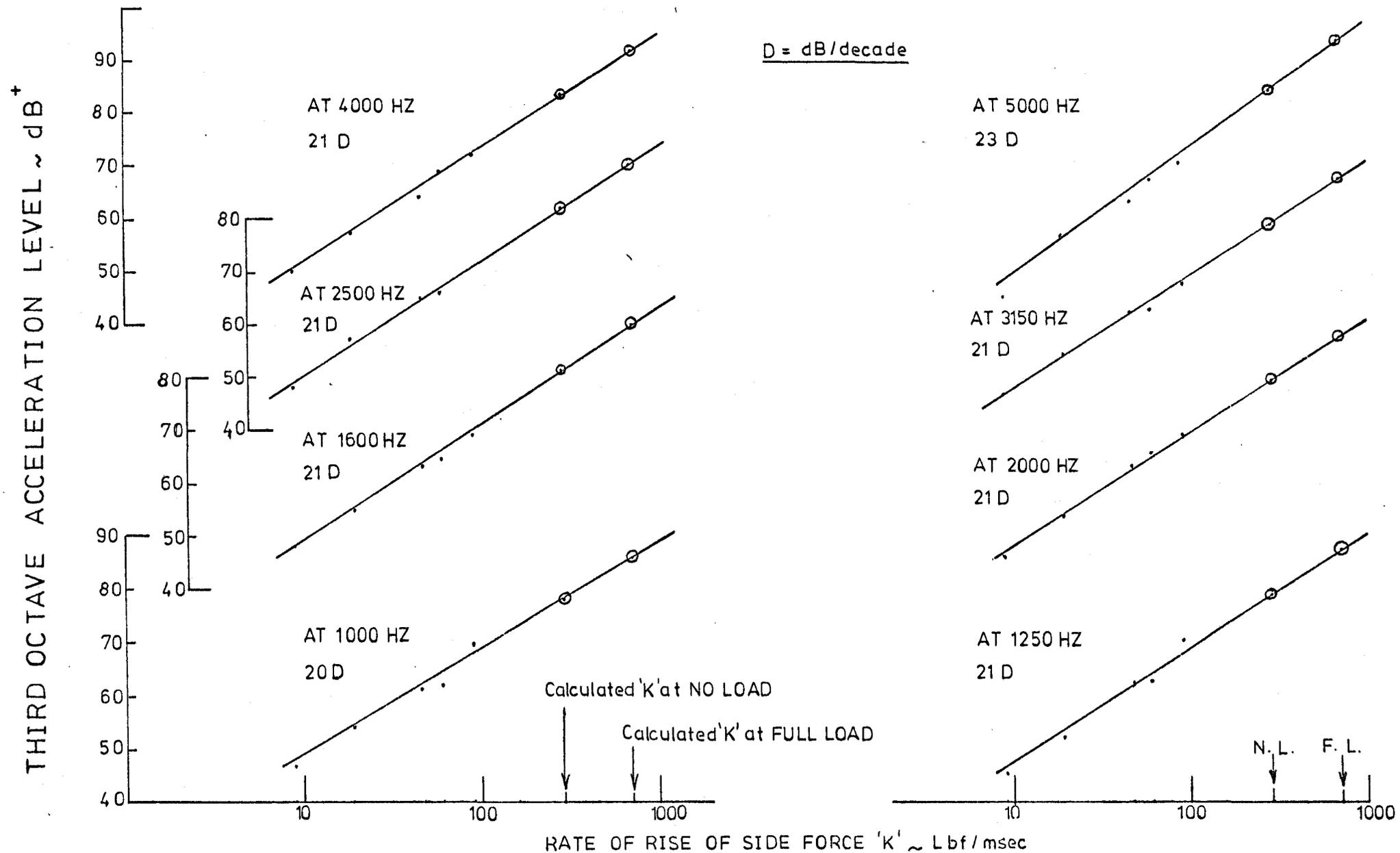
FIG. 5.21 RELATION BETWEEN VIBRATION RESPONSE AT  $Cl_3$  AND 'k' FACTOR AT REPETITION RATE 25 per sec.  $\approx$  1500 RPM ENGINE SPEED (SA)
