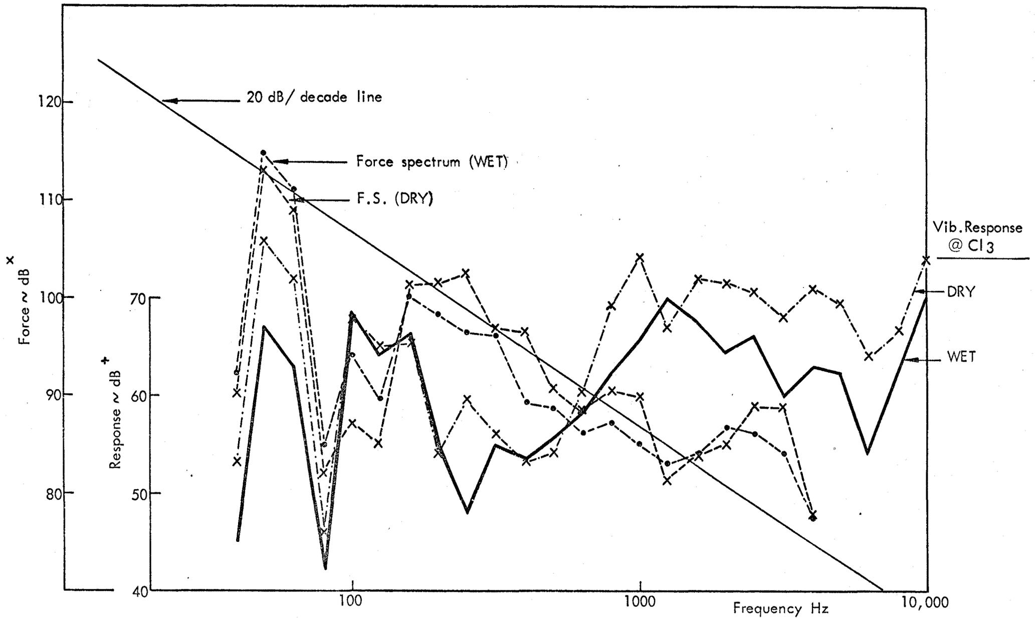
FIG. 5.30f TYPICAL EFFECT OF OIL FILM ON THE VEE RIG AT REPETITION RATE 55 per sec. — STANDARD PISTONS OF SA
