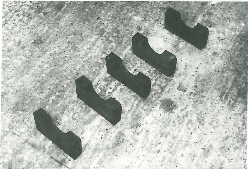
FIG. 3.24b THE SEPARATE BEARING CAPS (  $\delta$  )
