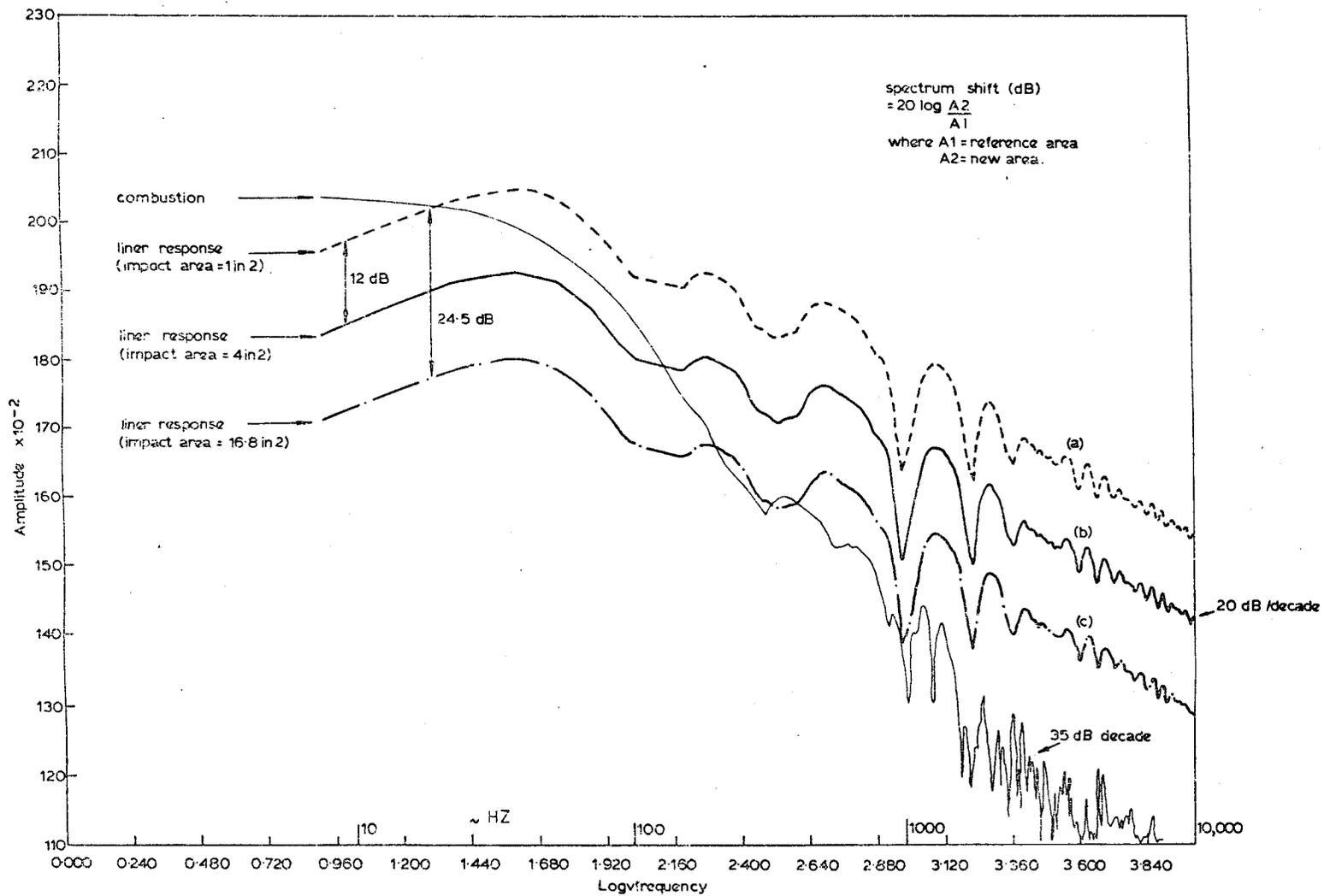
FIG. 3H RELATIONSHIP BETWEEN COMBUSTION AND ENGINE LINER RESPONSE AT 1000 revs/min NO LOAD FOR A V8 7.7 LITRE DIESEL ENGINE.
