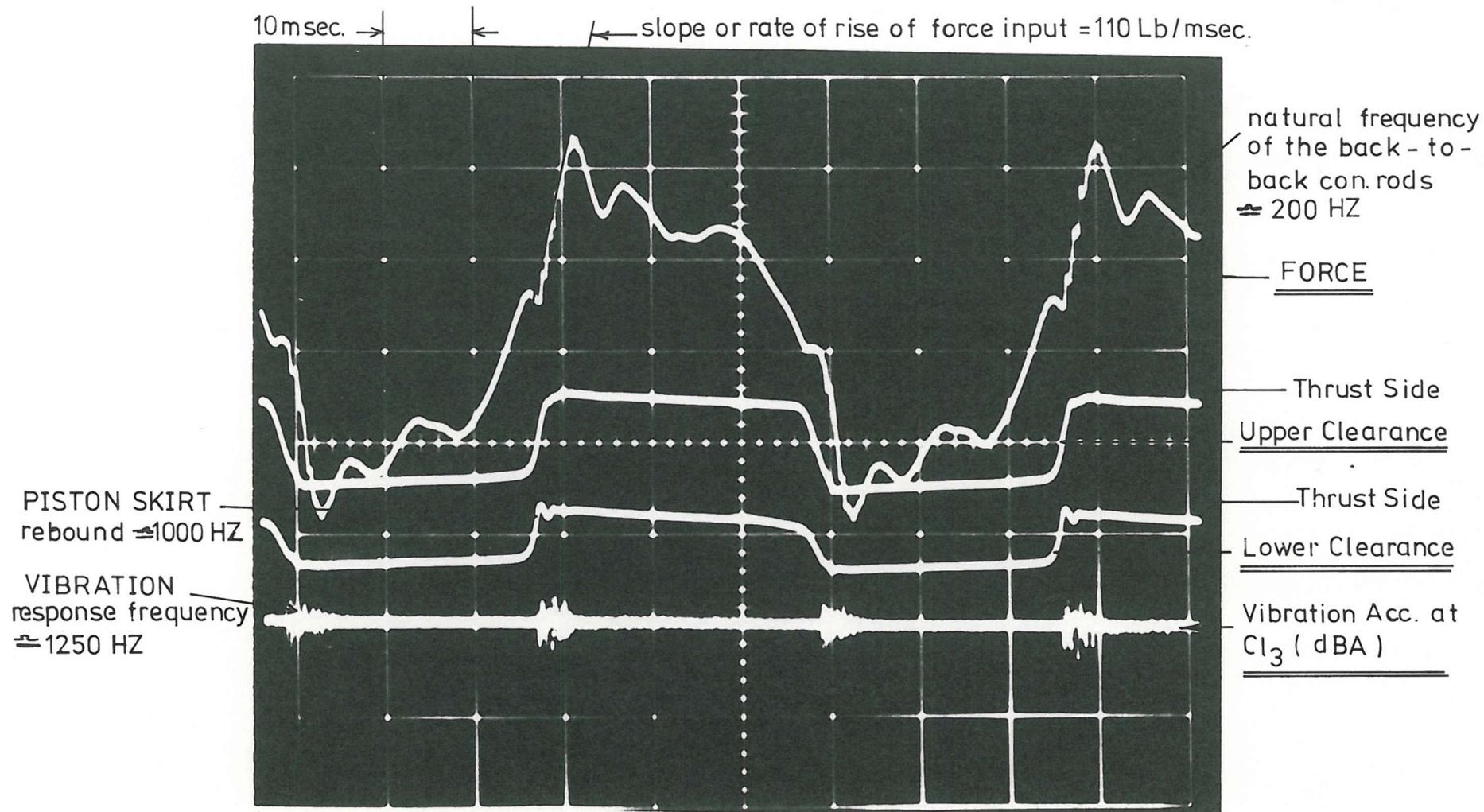
FIG. 5.15 TYPICAL OSCILLOGRAPH FOR THE VEE PISTON SLAP RIG AT REPETITION RATE 16.7 per sec.  $\approx 1000$  RPM ( DRY CASE )
