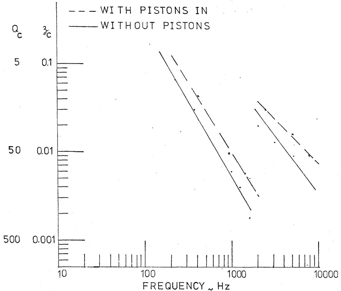
FIG. 4E. MODAL DAMPING RATIOS BETWEEN THE LINER AND ENGINE BLOCK OF V8 SA DIESEL ENGINE
