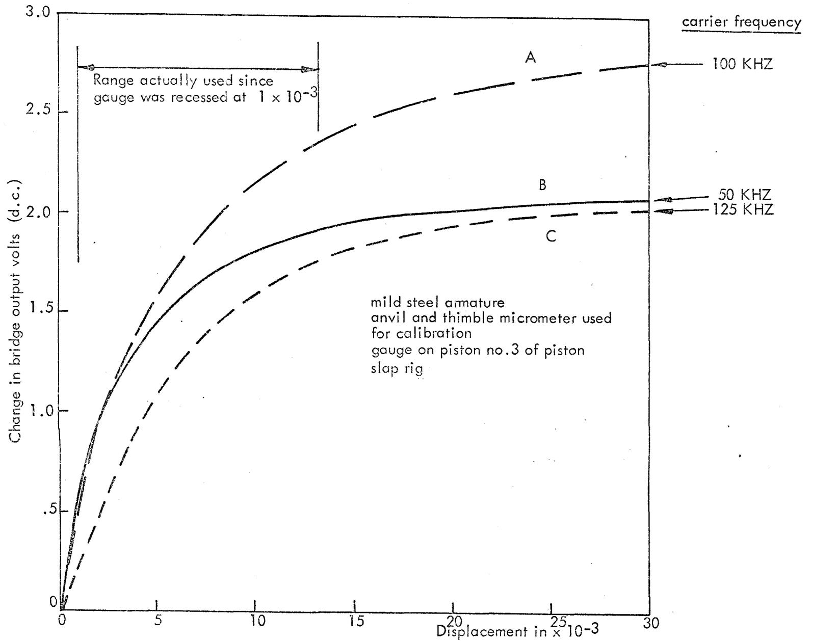
FIG.1F CALIBRATION OF UPPER CLEARANCE AET 4 INDUCTIVE GAUGE
