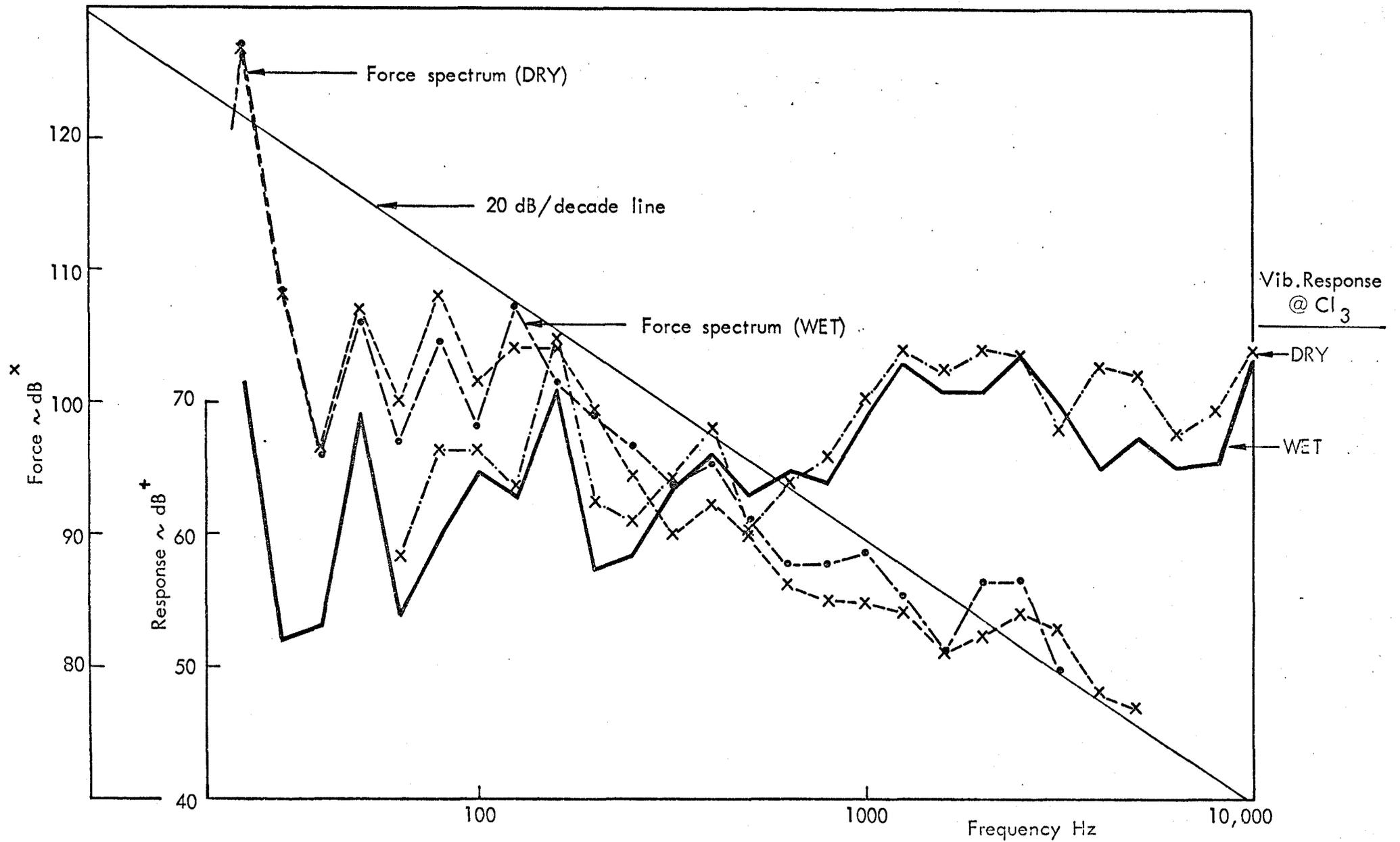
FIG. 5.30 b TYPICAL EFFECT OF OIL FILM ON THE VEE RIG AT REPETITION RATE 25 per sec.— STANDARD PISTONS OF SA
