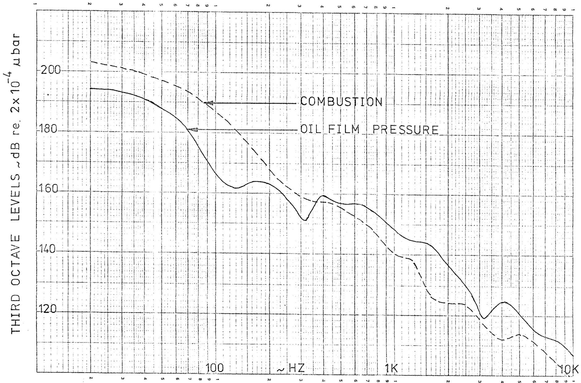
FIG. 7.20 SPECTRA OF PISTON TO BORE OIL FILM PRESSURE AND COMBUSTION FOR SA ENGINE AT 1000 RPM NO LOAD
