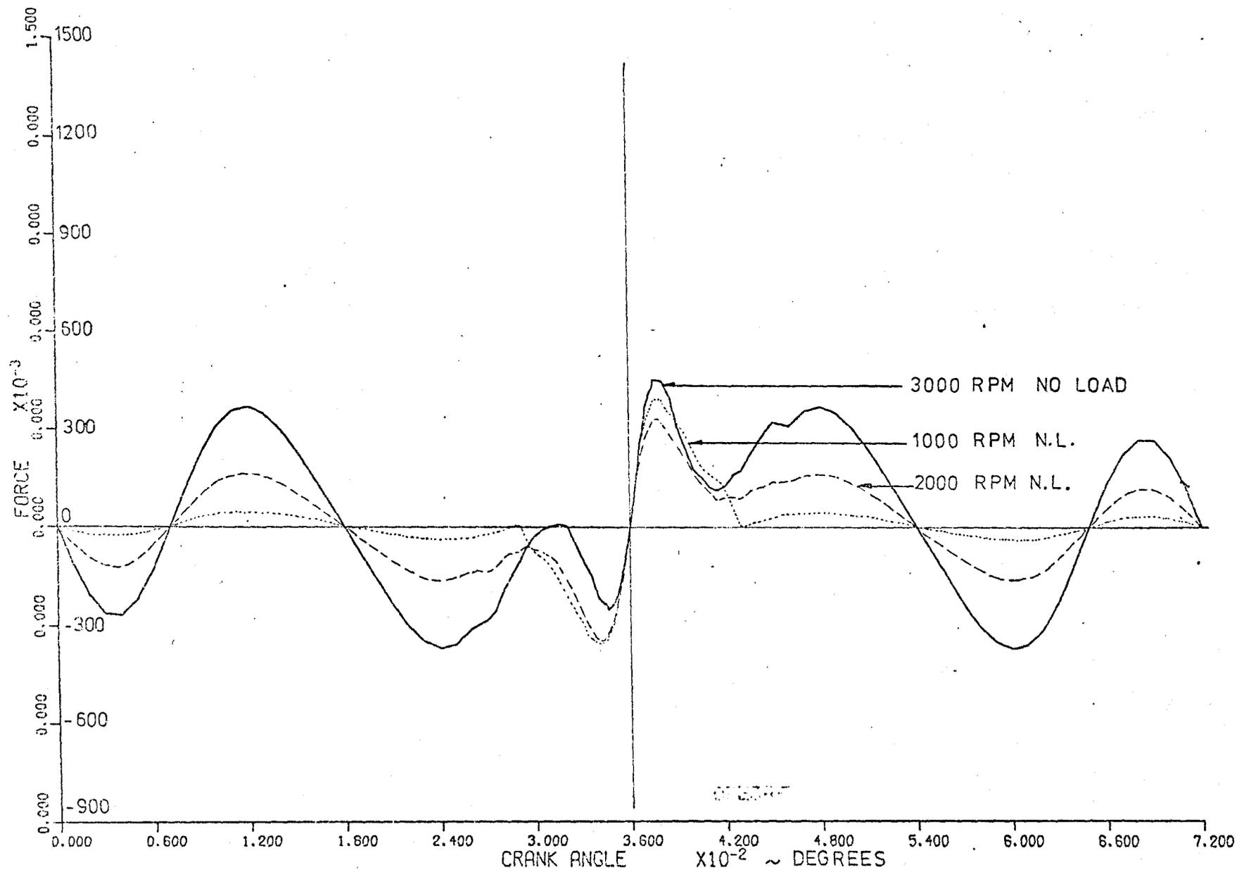
FIG. 7.16 PISTON SIDEWAYS FORCES FOR ENGINE SA
