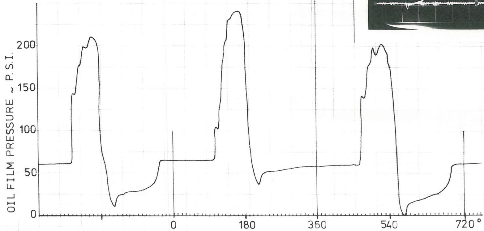
FIG. 7.8 CYLINDER PRESSURE AND PISTON TO BORE OIL FILM PRESSURE ( T.S. )
