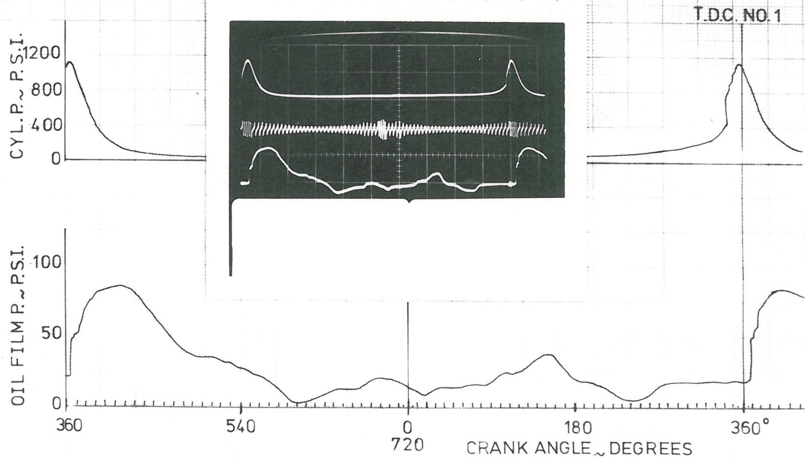
FIG. 7.9 CYLINDER PRESSURE AND PISTON TO BORE OIL FILM PRESSURE (T.S.) AT 1000 RPM FULL LOAD - SA ENGINE
