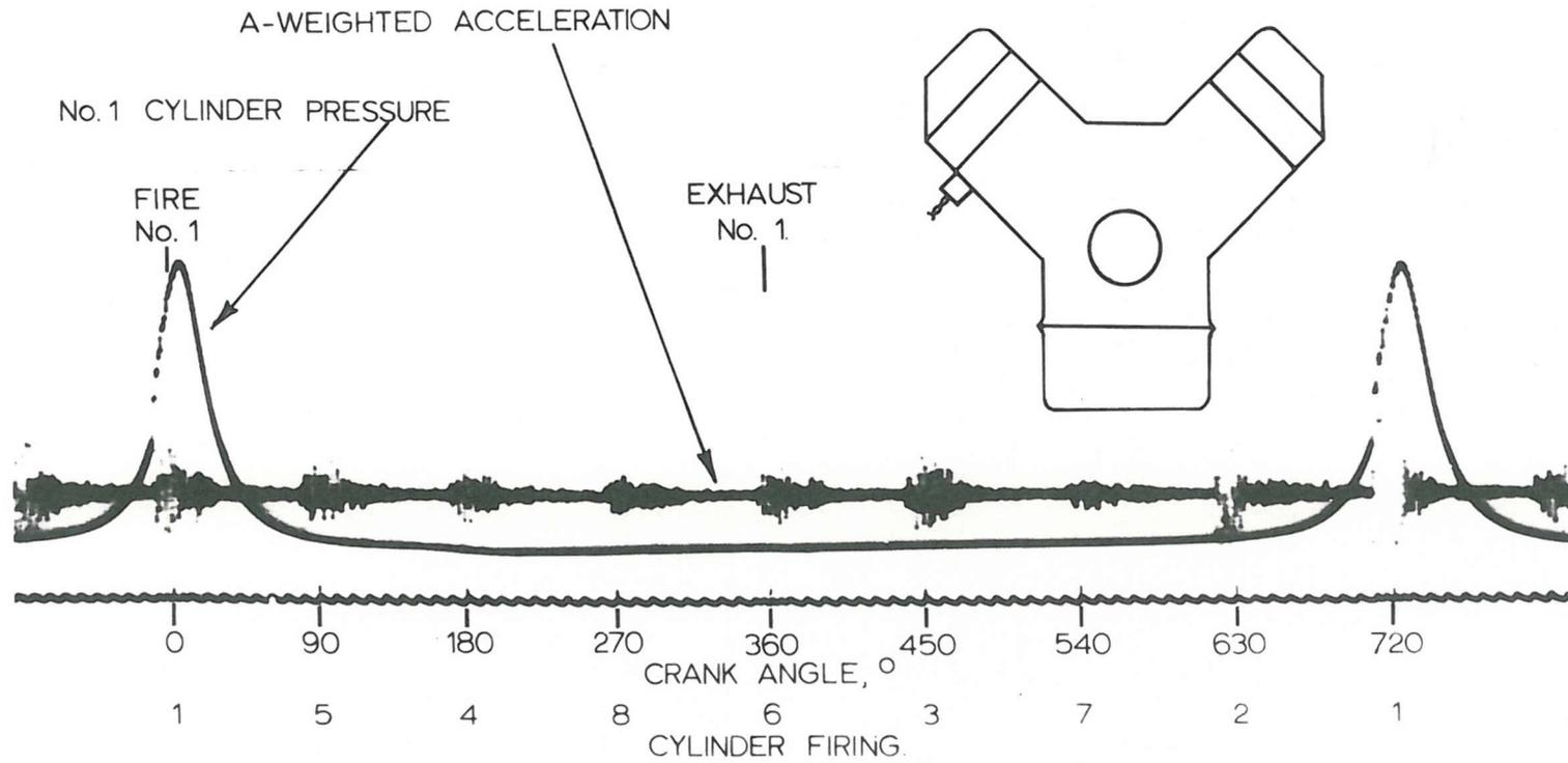
FIG. 4.10 Piston Slap Contribution to Cylinder Block Vibration in a Running Engine
