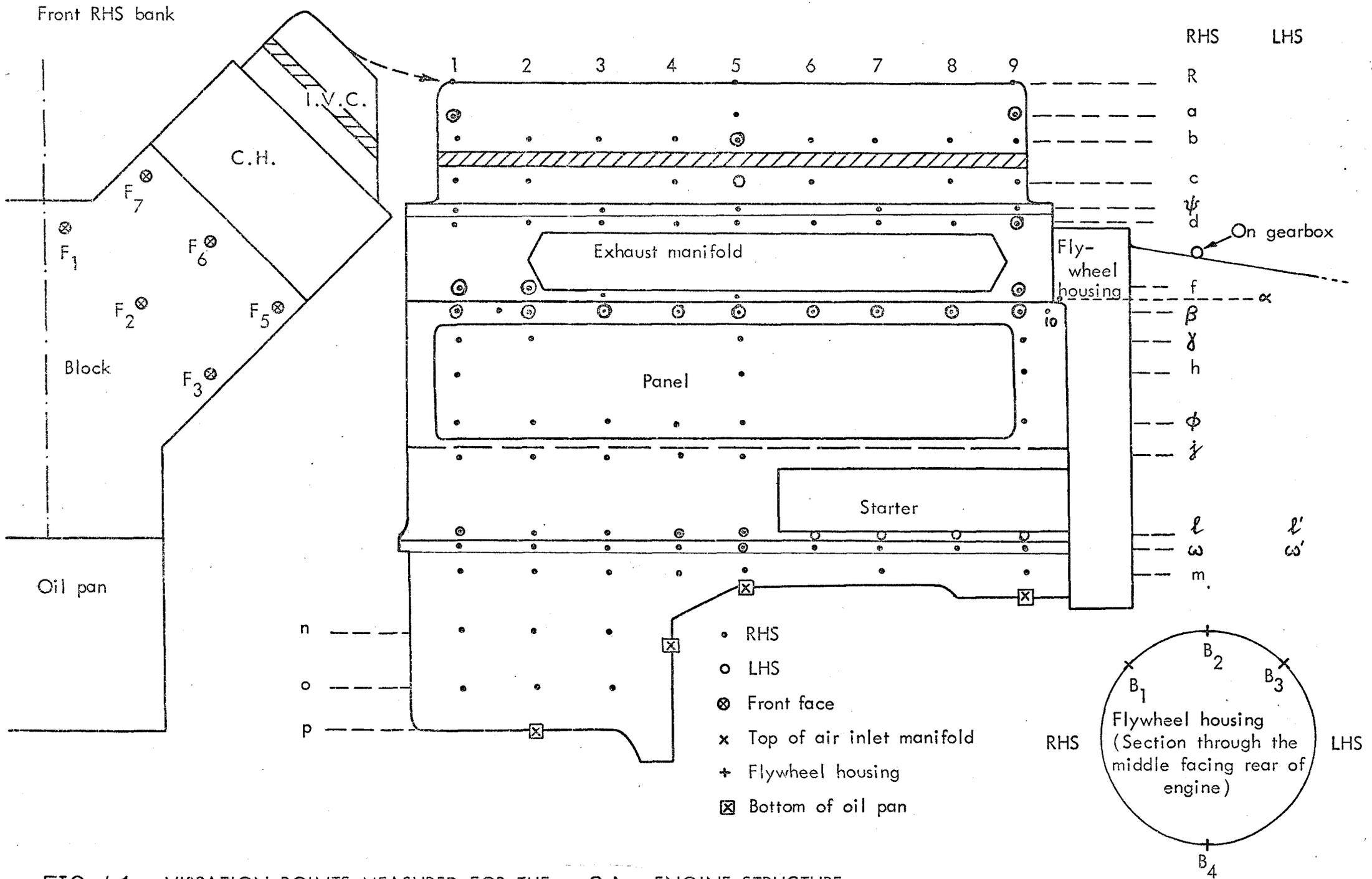
FIG. 4.1 VIBRATION POINTS MEASURED FOR THE SA ENGINE STRUCTURE.
