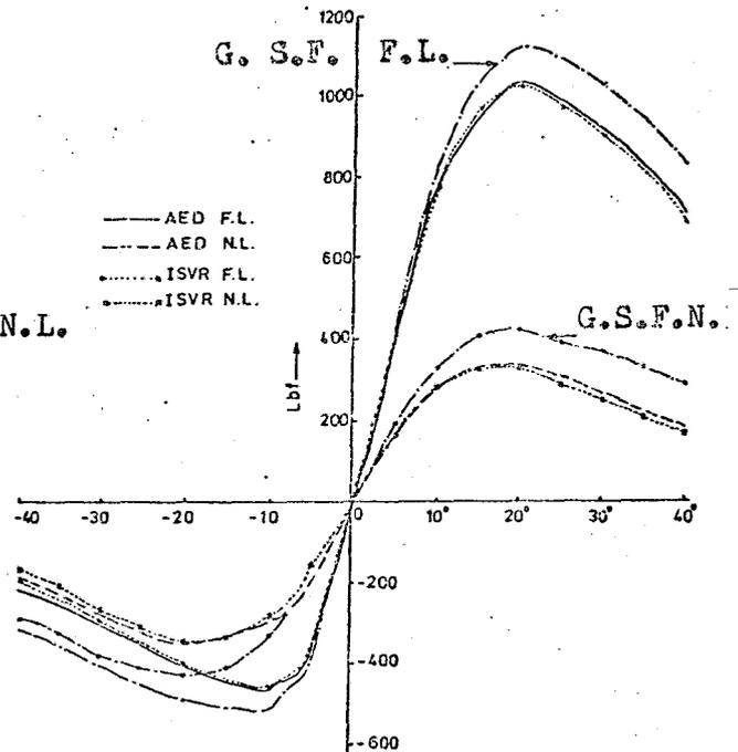
COMPARISON OF COMPUTED PISTON SIDE FORCES AROUND T.D.C. USING ISVR and AED PROGRAMMES AT 2000 RPM FULL AND NO LOAD (ENGINE SA G.P.O.=0)
