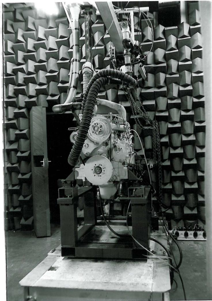
FIG. 3.1 TYPICAL INSTALLATION OF DIESEL ENGINE
