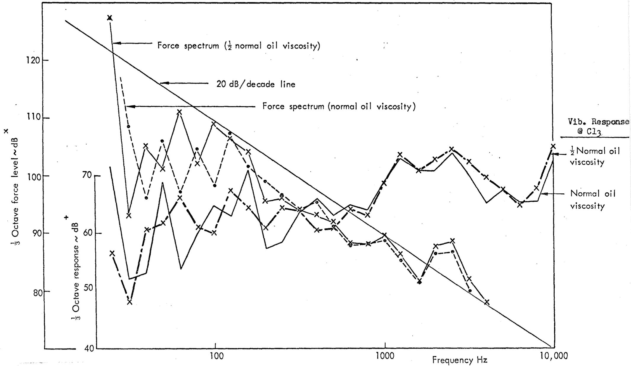
FIG. 5.34 b FORCE RESPONSE SPECTRA SHOWING EFFECT OF VARYING OIL FILM VISCOSITY ON THE V8 PISTON SLAP RIG FOR THE STANDARD PISTONS AT  $25 \text{ Hz} \cong 1500 \text{ R.P.M.}$
