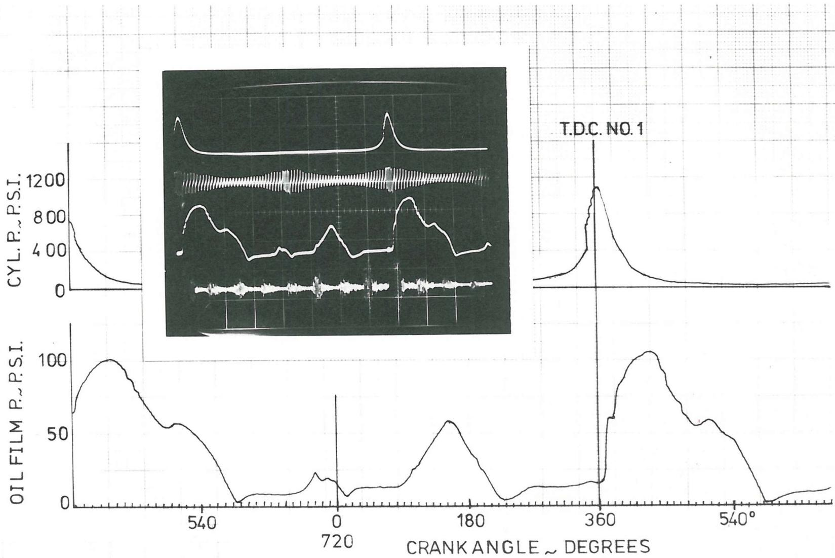
FIG. 7.10 CYLINDER PRESSURE AND PISTON TO BORE OIL FILM PRESSURE ( T.S. )
