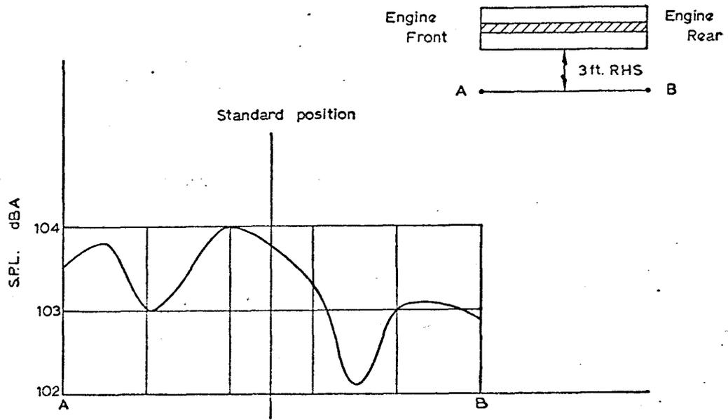
FIG. 3.3 a Overall SPL variation when moving microphone across line AB for standard valve at 3300 full load.
