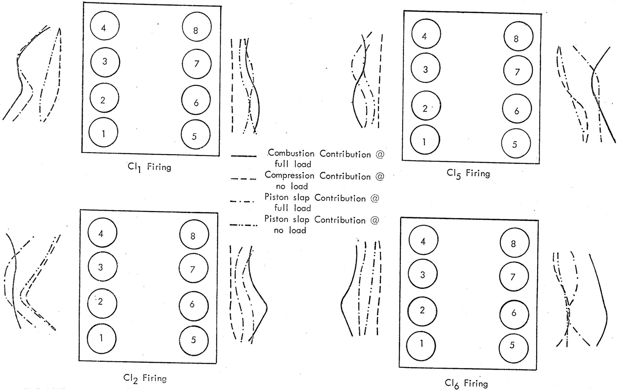
FIG. 4.13 MAXIMUM VIBRATION AMPLITUDES FOR SA ENGINE STANDARD @ 1500 r.p.m.
