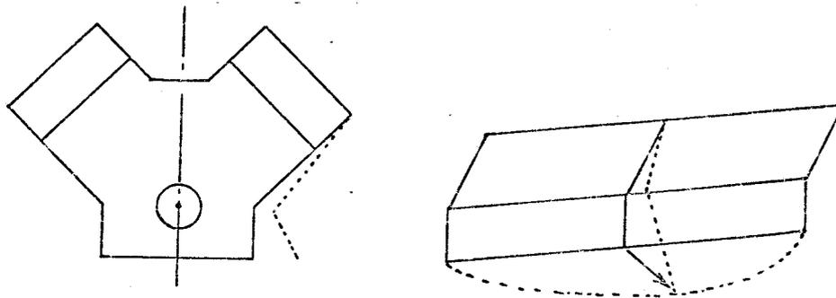
Fig. 3.18. Idealised displacement of the conical mode on one side of a V8 engine ( $\approx 2500$  Hz for SA).
