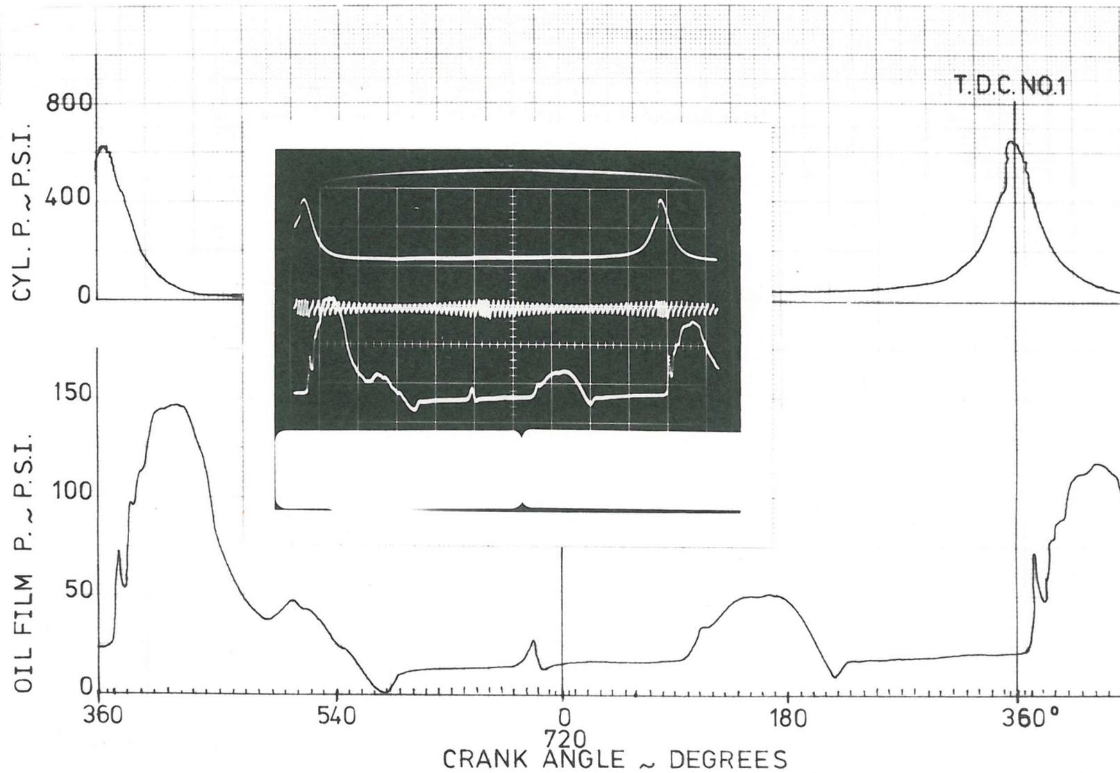
FIG. 7.4 CYLINDER PRESSURE AND PISTON TO BORE OIL FILM PRESSURE ( THRUST SIDE )
