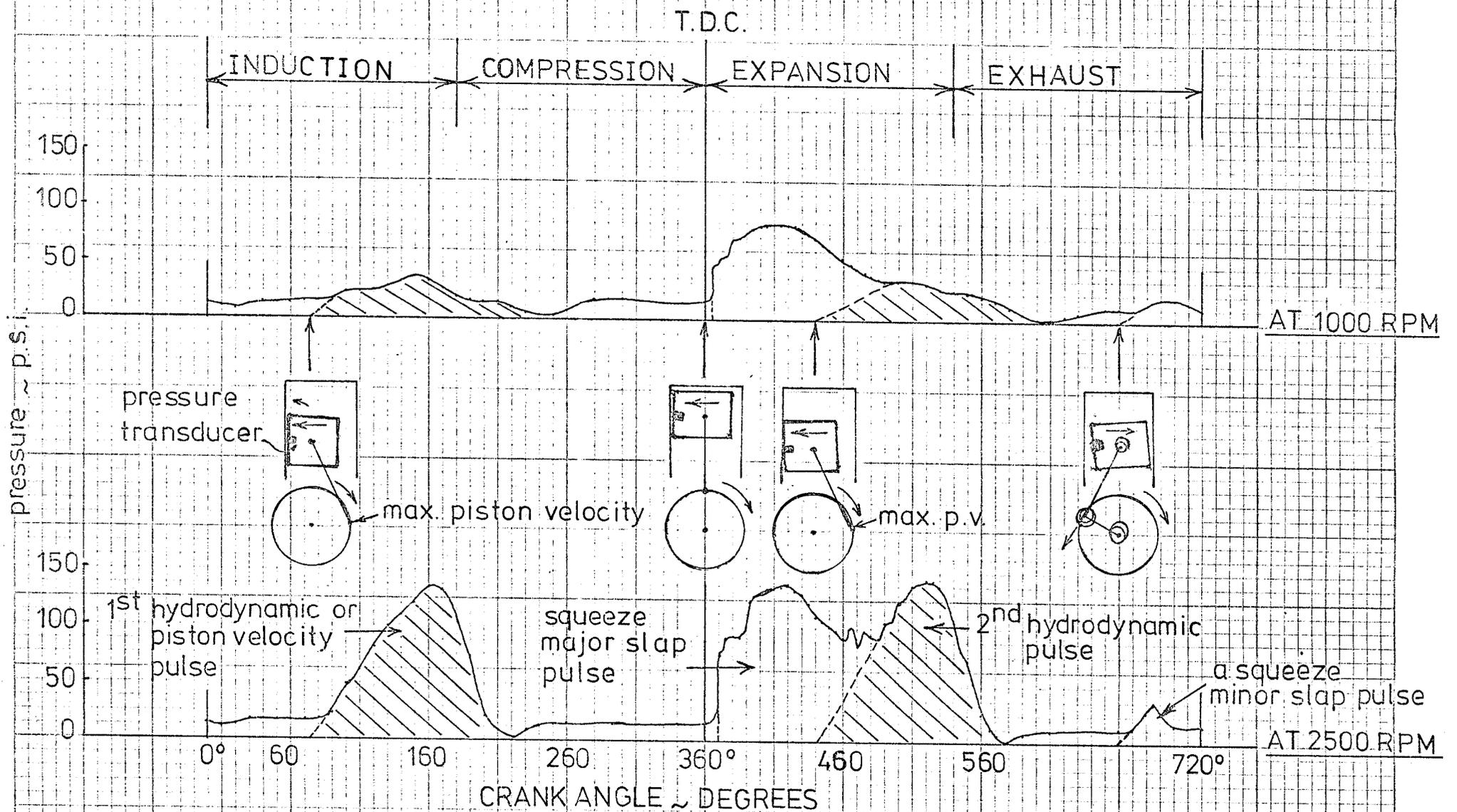
FIG. 7.15 VARIATION OF PISTON TO BORE OIL FILM PRESSURE (THRUST SIDE) WITH ENGINE SPEED AT FULL LOAD FOR THE RUNNING V8 SA DIESEL ENGINE
