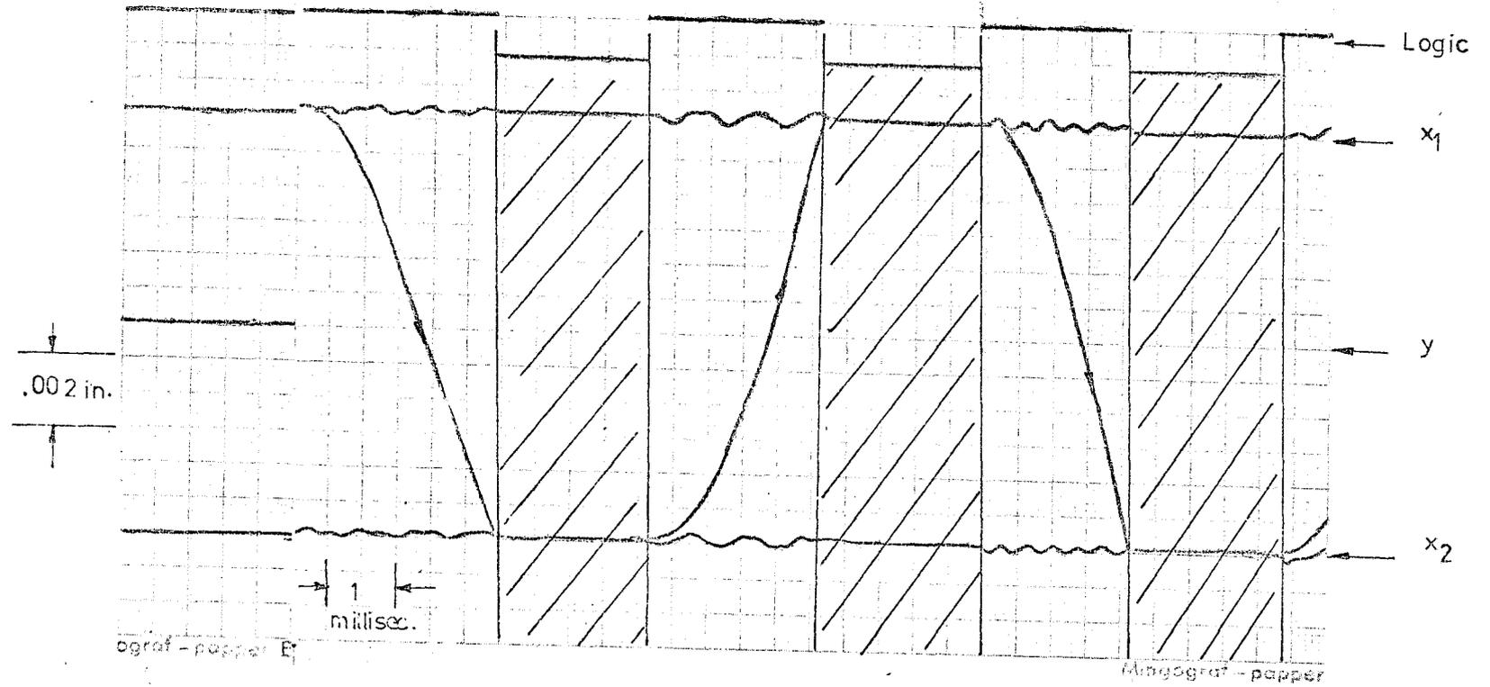
FIG. 6.5 Effect of increased mass of liner ( $m_c > m_p$ )
