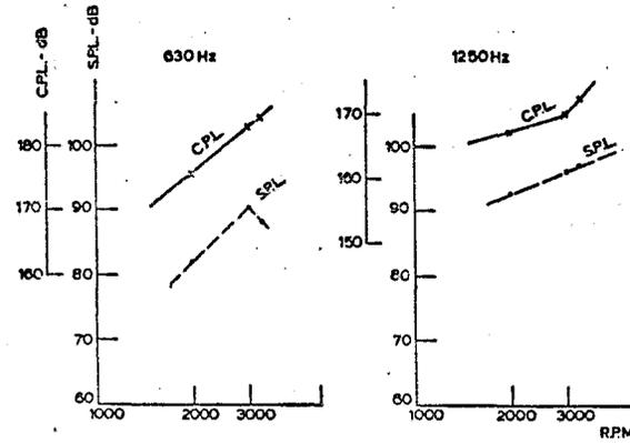
FIG. 3.13 b Variation of cylinder pressure and noise with speed for the standard engine at full load and operating temperatures - 630 and 1250 Hz.
