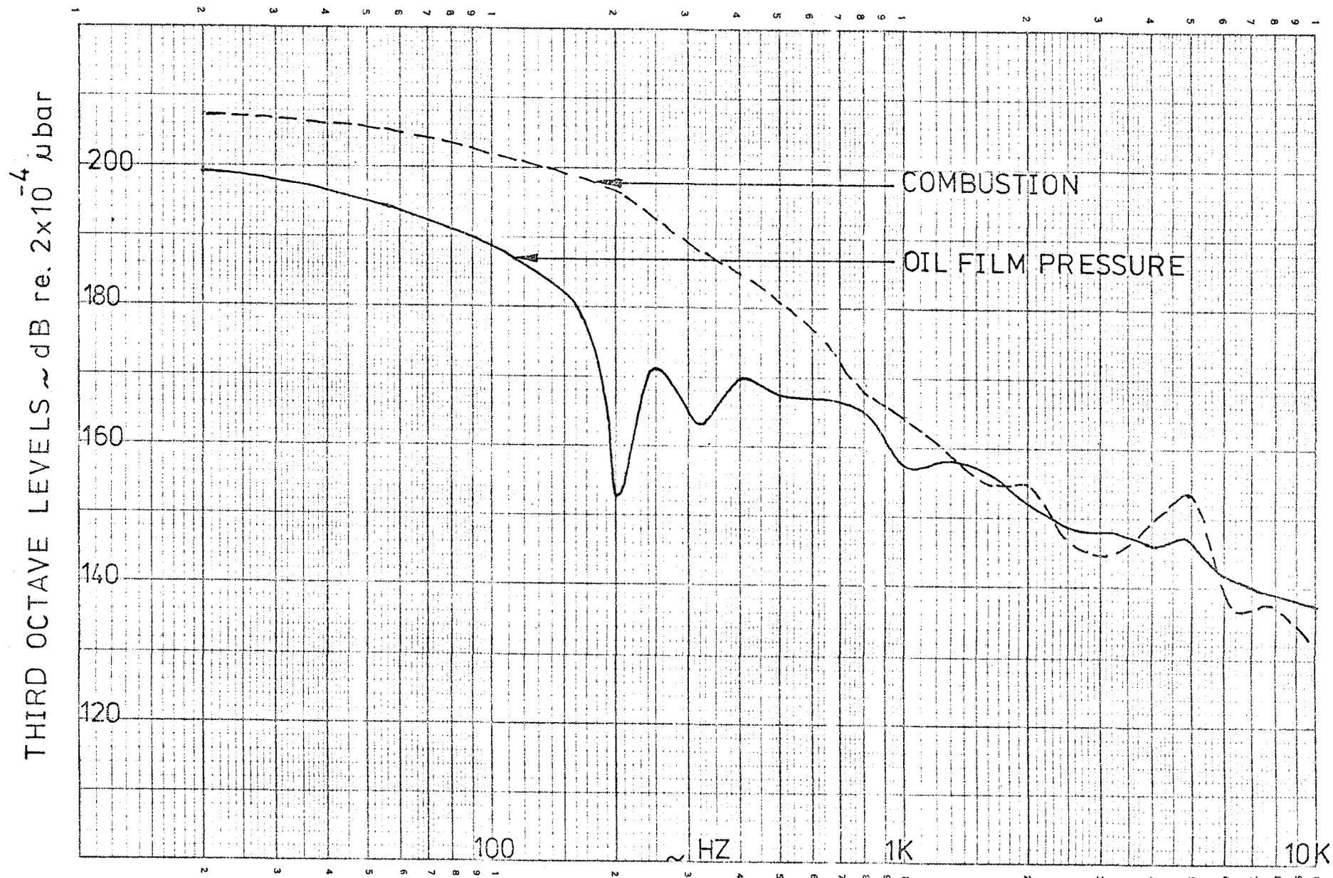
FIG. 7.25 SPECTRA OF PISTON TO BORE OIL FILM PRESSURE AND COMBUSTION FOR THE SA ENGINE AT 2500 RPM FULL LOAD
