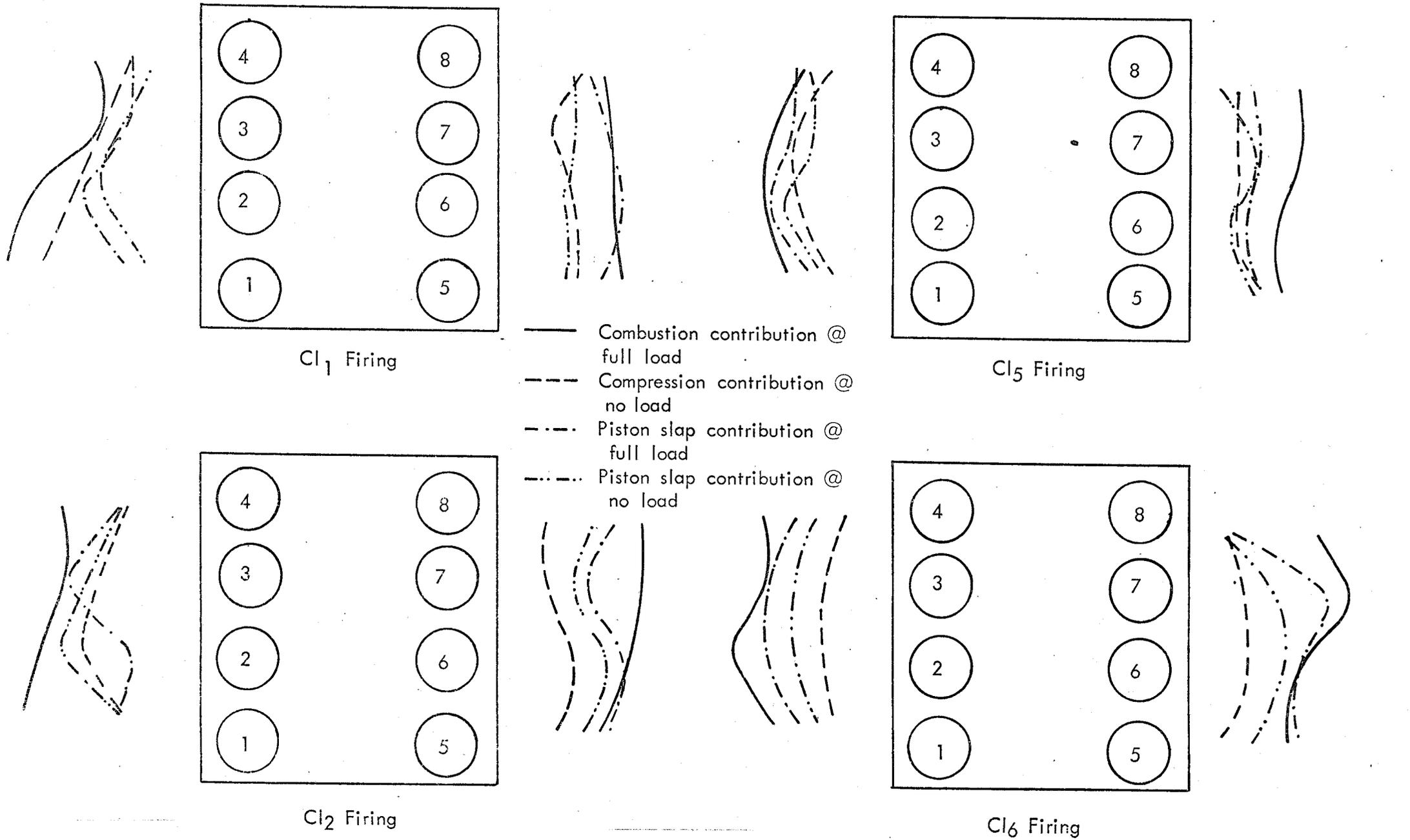
FIG. 4.17 MAXIMUM VIBRATIONS AMPLITUDES FOR SA ENGINE STANDARD @ 3000 r.p.m.
