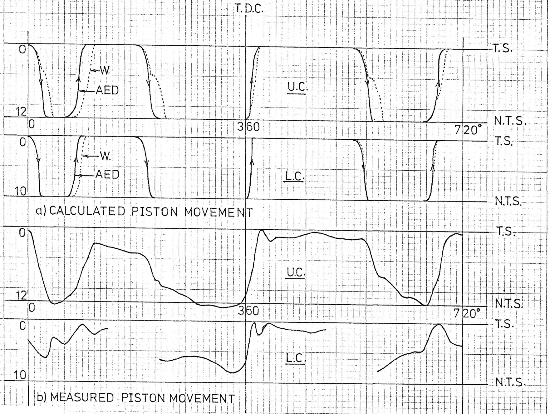
FIG. 7.33 COMPARISON OF CALCULATED AND MEASURED PISTON MOVEMENT PLOTS FOR ENGINE SA at 2000 RPM NO LOAD
