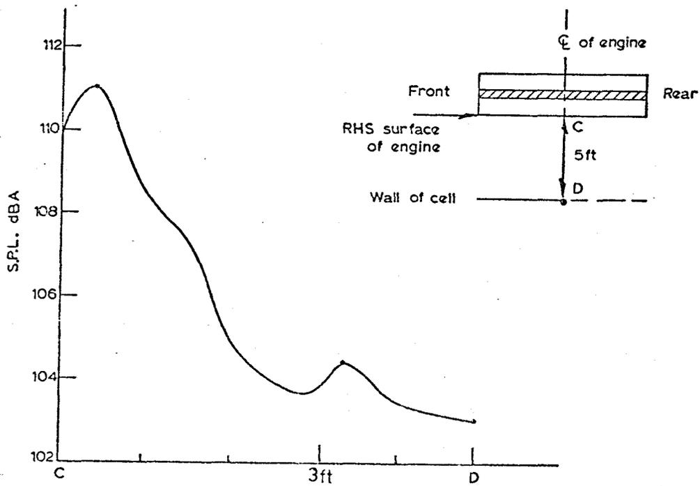
FIG. 3.3 b Overall SPL variation when moving microphone across line CD for standard valve at 3300 full load.
