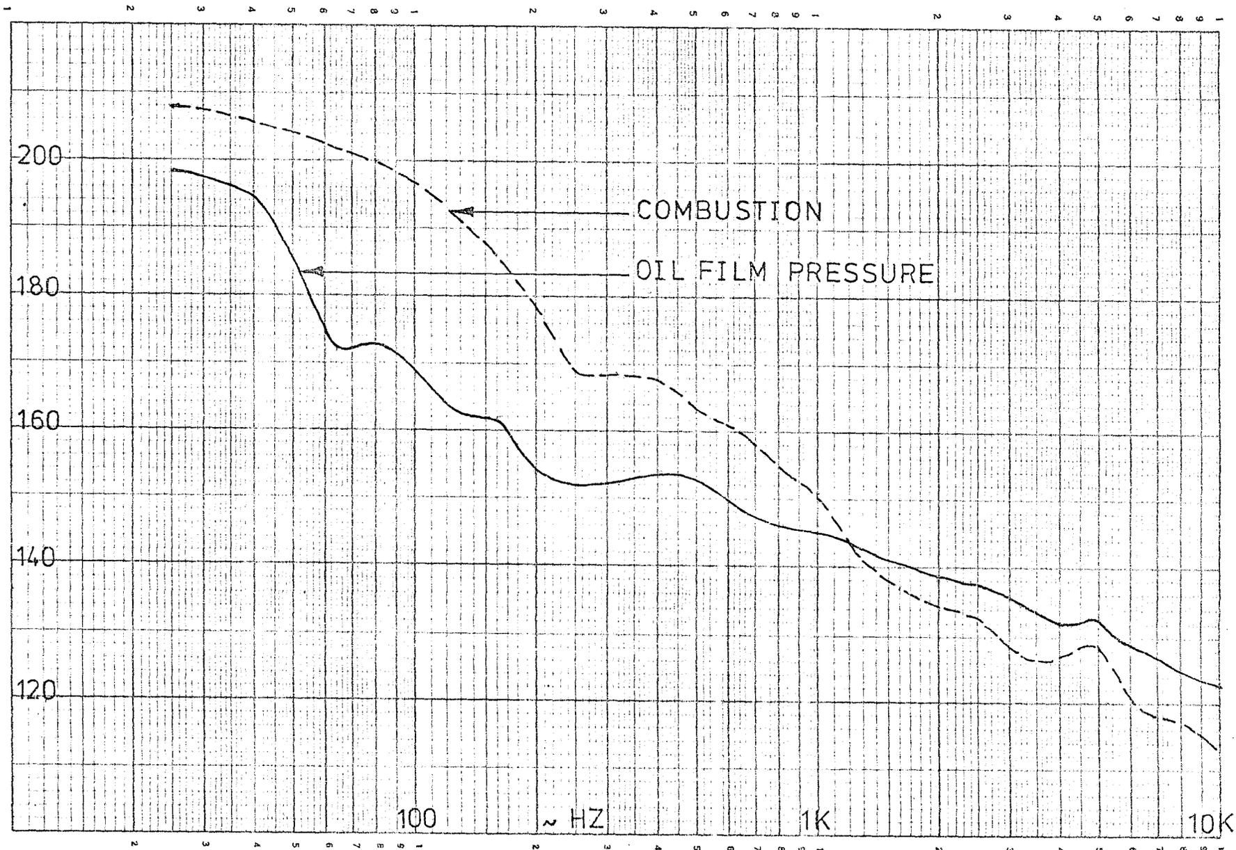
FIG. 7.23 SPECTRA OF PISTON TO BORE OIL FILM PRESSURE AND COMBUSTION FOR SA ENGINE AT 1000 RPM FULL LOAD
