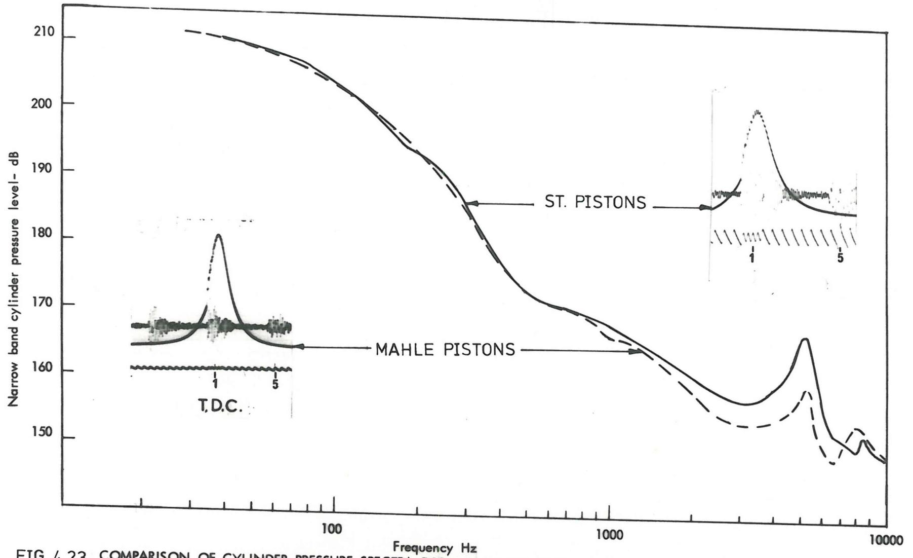
FIG. 4.23 COMPARISON OF CYLINDER PRESSURE SPECTRA FOR THE SA ENGINE FITTED WITH STANDARD AND MAHLE PISTONS @ 1500 r.p.m. FULL LOAD.
