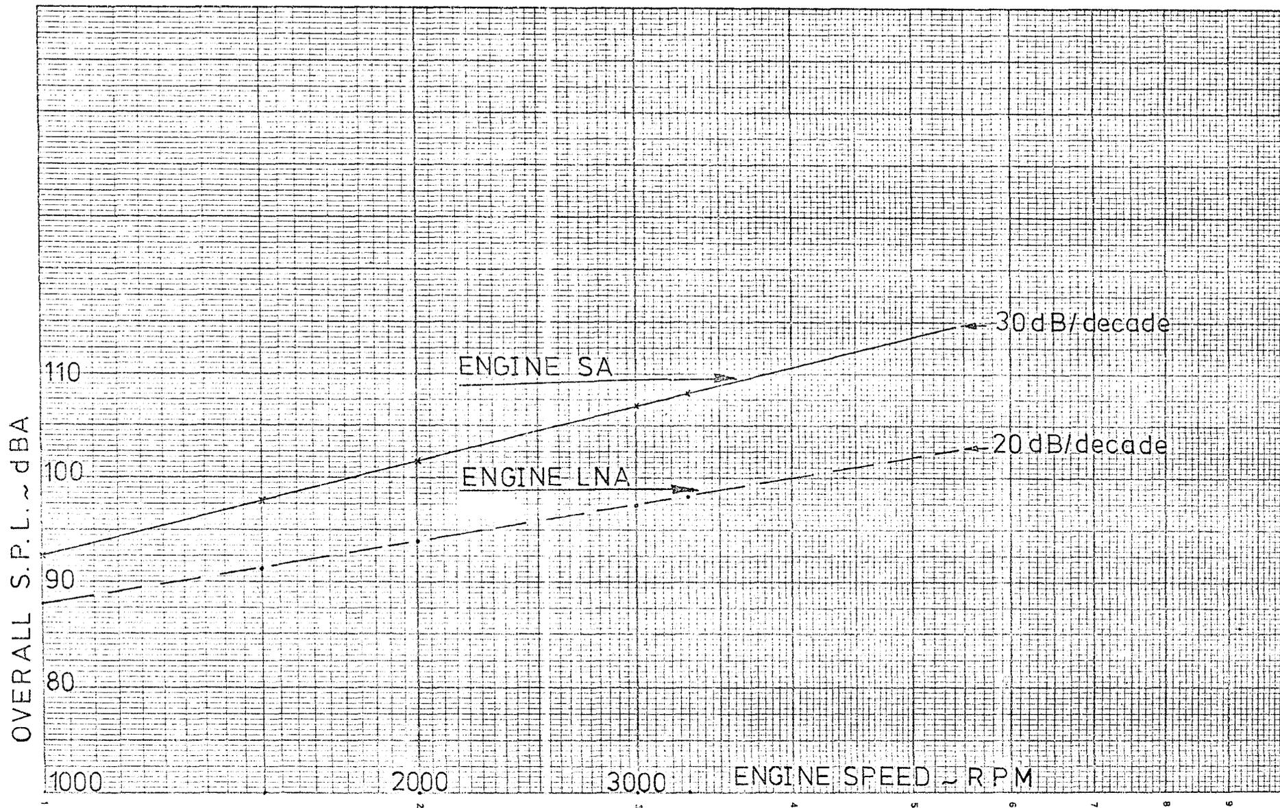
FIG. 3.30 COMPARISON OF STANDARD AND LOW NOISE ENGINE AT FULL LOAD
