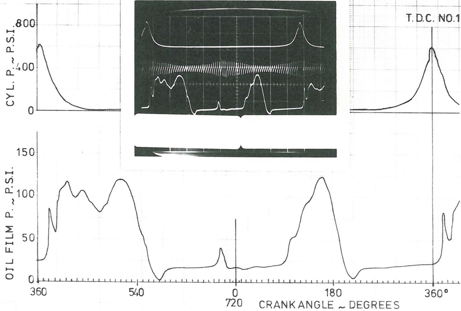
FIG. 7.6 CYLINDER PRESSURE AND PISTON TO BORE OIL FILM PRESSURE (THRUST SIDE) AT 2000 RPM NO LOAD - SA ENGINE
