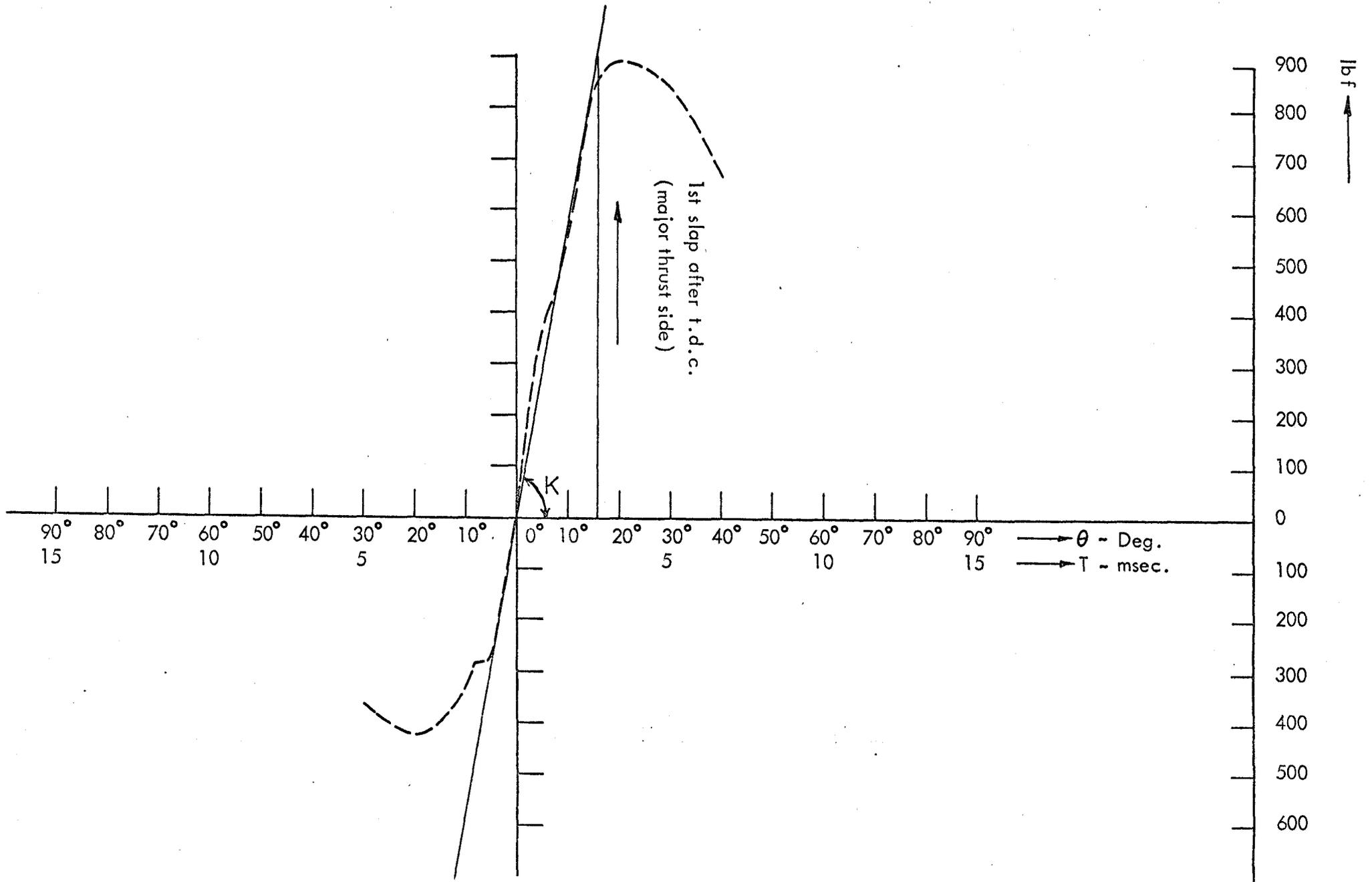
FIG. 5.3 CALCULATED PISTON SIDE FORCE OF ENGINE AT 1000 r.p.m. FULL LOAD
