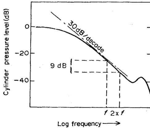
Fig. 3.19. Reduction of excitation by increase in frequency.
