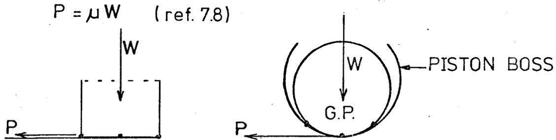
Finally, the strains on the gudgeon pin, piston and connecting rod may be measured and related to the forces in the system with the possibility of giving an accurately measured piston side force (top and bottom) taking into account the effect of all parameters.
