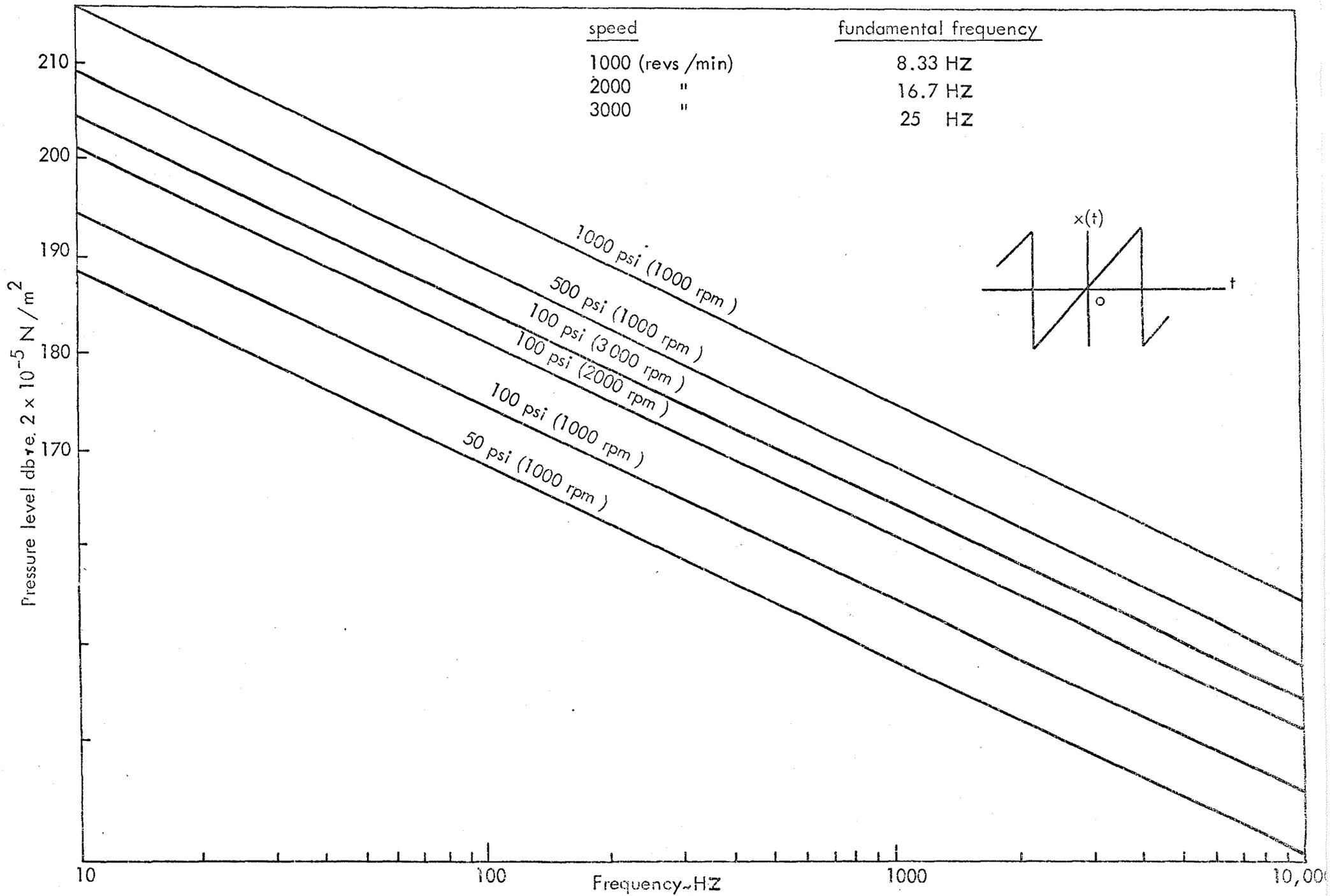
FIG. 1G FOURIER SPECTRA OF SAWTOOTH WAVEFORMS SHOWING THE EFFECT OF VARYING THE AMPLITUDE AND THE FUNDAMENTAL FREQUENCY
