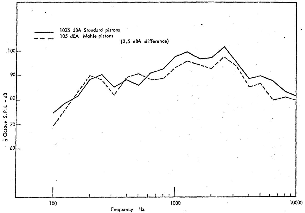
FIG. 4.2 RHS NOISE COMPARISON BETWEEN THE STANDARD AND MAHLE PISTONS FITTED ON THE SA ENGINE @ 3300r.p.m. FULL LOAD.
