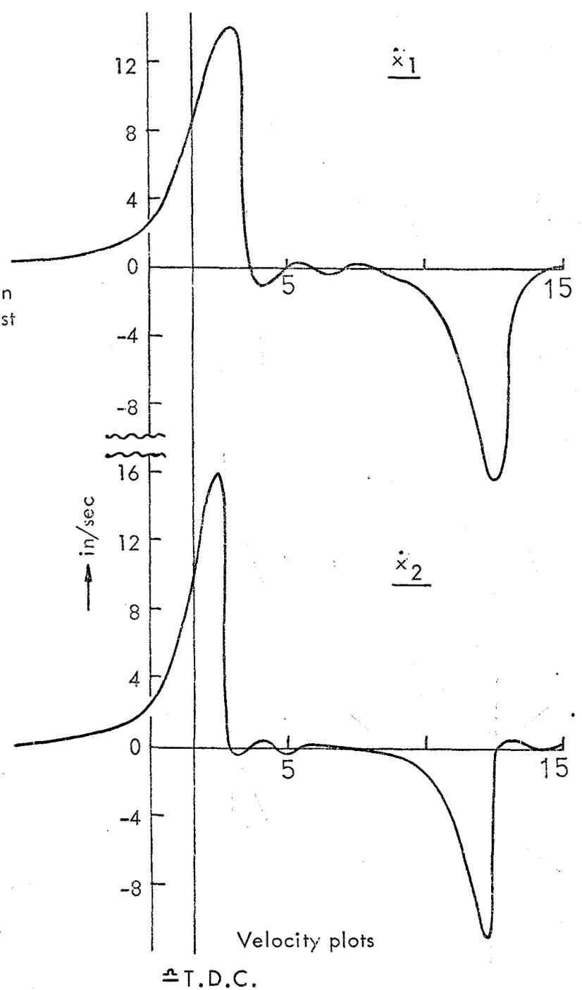
FIG 2A PROXIMITY AND VELOCITY PLOTS OF THE PISTON DUE TO A CERTAIN FORCE AT 50 Hz  $\equiv$  3000 RPM (DRY CASE)
