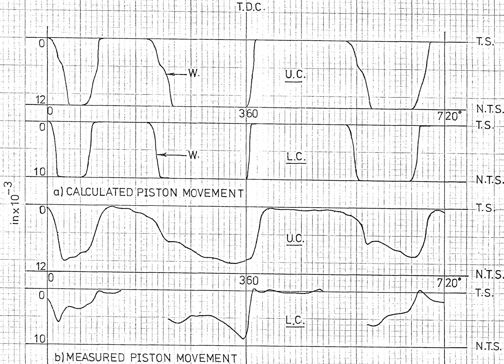
FIG. 7.38 COMPARISON OF CALCULATED AND MEASURED PISTON MOVEMENT PLOTS FOR ENGINE SA at 2500 RPM FULL LOAD
