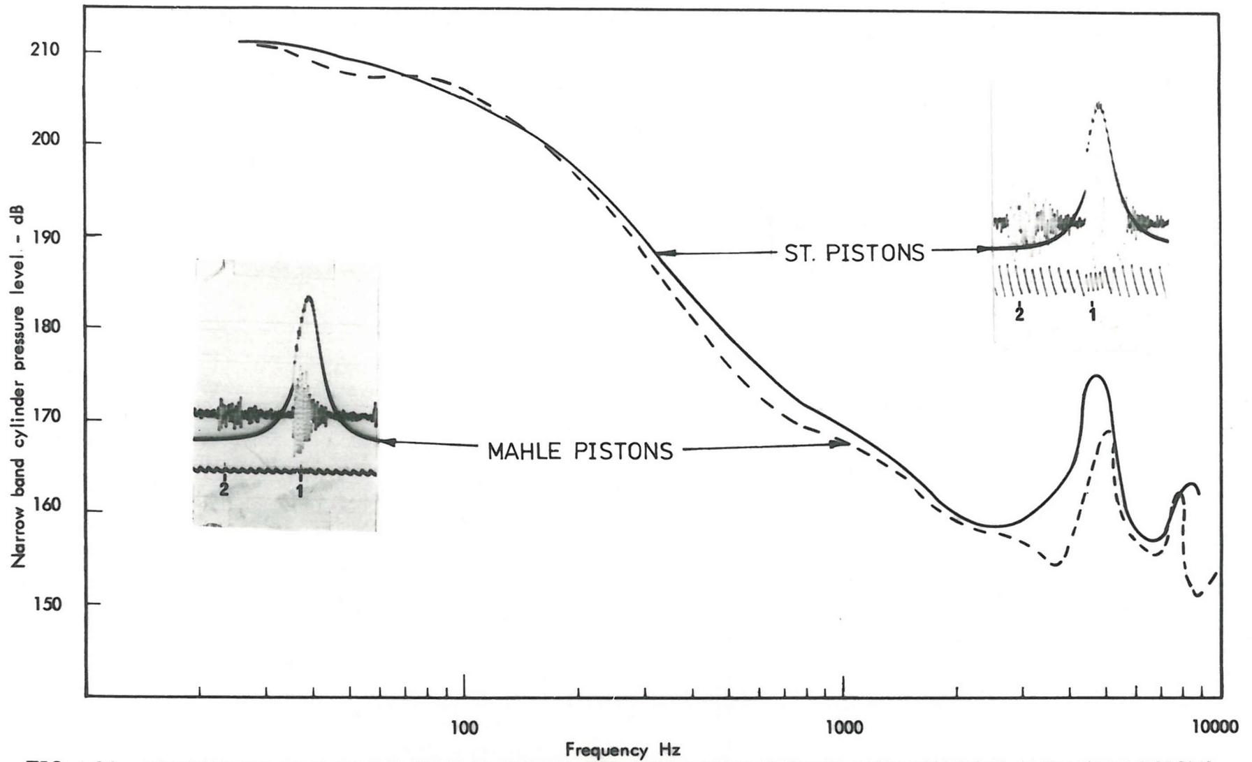
FIG. 4.22 COMPARISON OF CYLINDER PRESSURE SPECTRA FOR THE SA ENGINE FITTED WITH STANDARD AND MAHLE PISTONS @ 2000 r.p.m. FULL LOAD.
