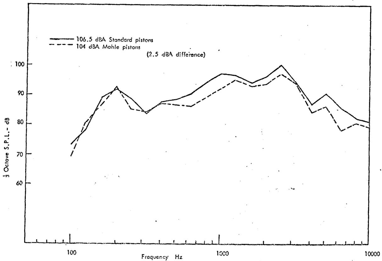
FIG. 4.3 RHS NOISE COMPARISON BETWEEN THE STANDARD AND MAHLE PISTONS FITTED ON THE SA ENGINE @ 3000 r.p.m. FULL LOAD.
