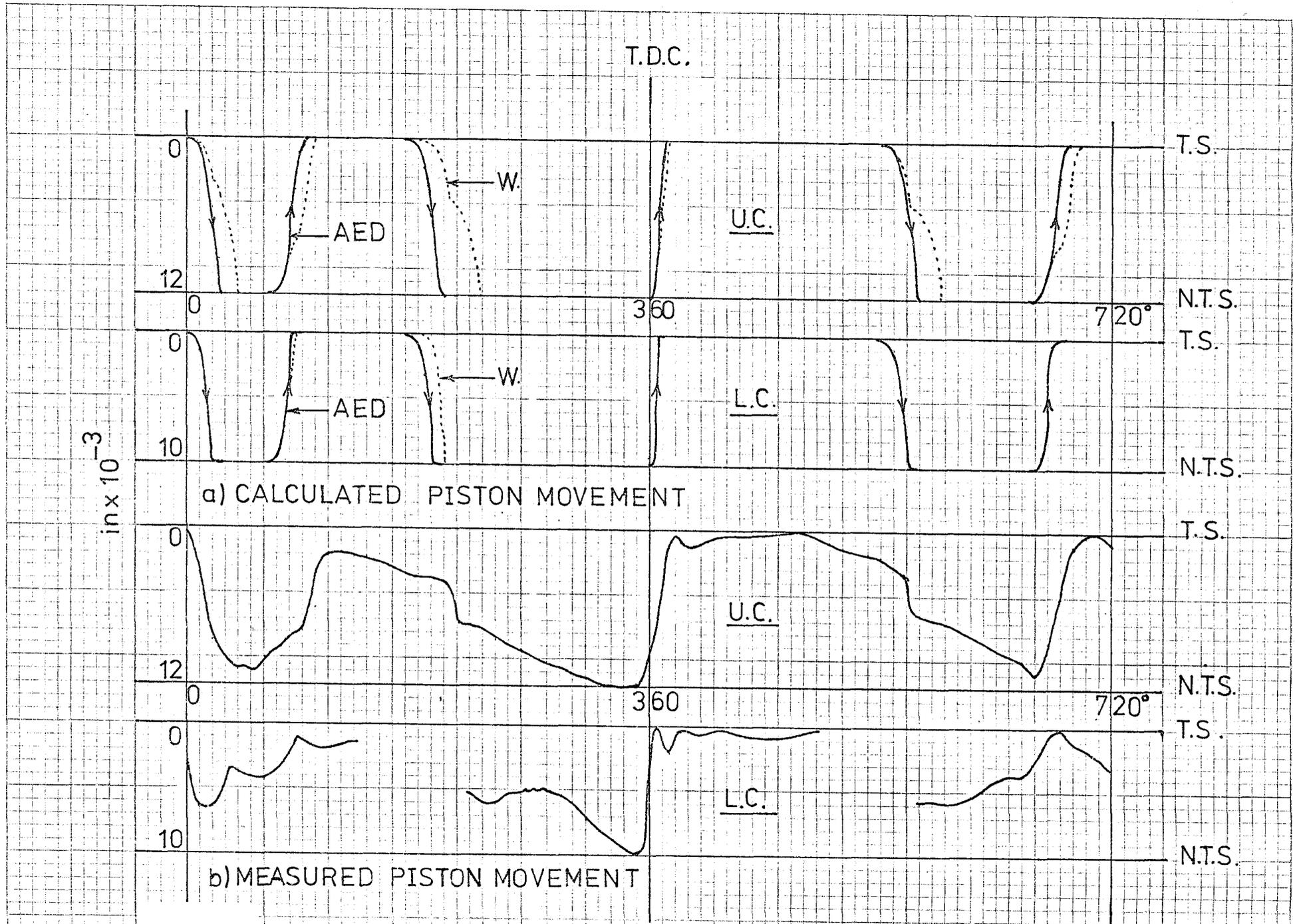
FIG. 7.37 COMPARISON OF CALCULATED AND MEASURED PISTON MOVEMENT PLOTS FOR ENGINE SA at 2000 RPM FULL LOAD
