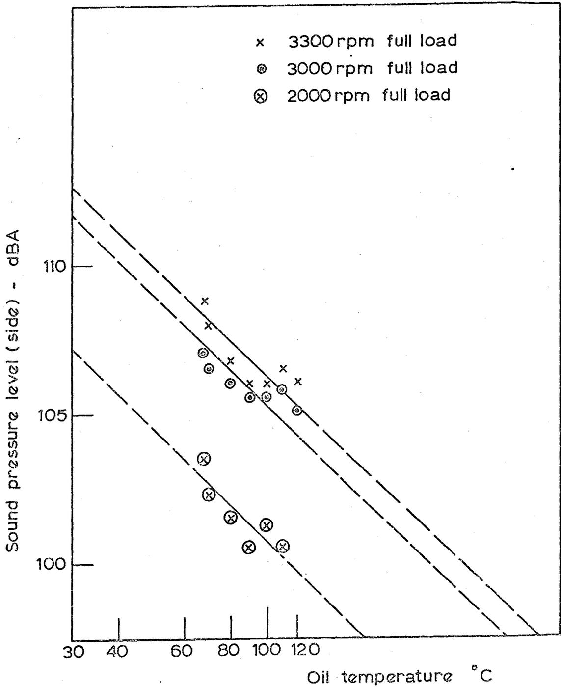
Fig. 3.10 Variation of overall noise level with oil temperature (log scale) for the SA engine - at full load.
