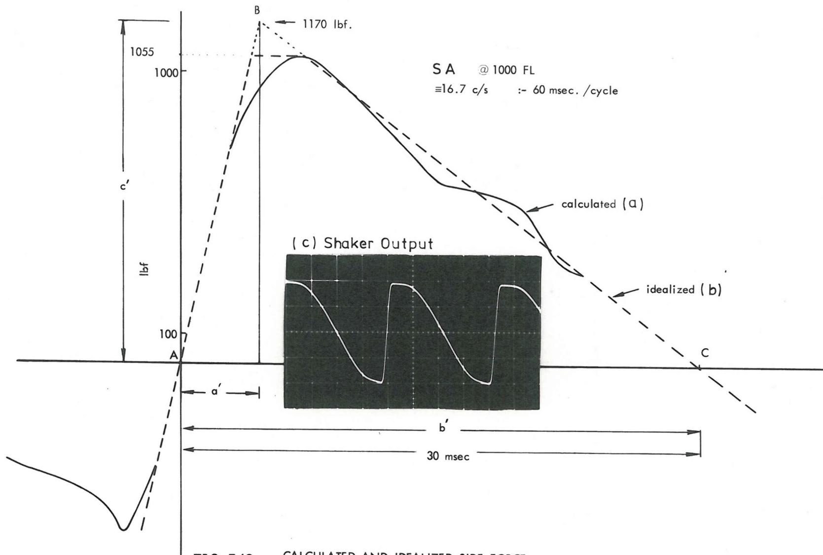
FIG. 5.13 CALCULATED AND IDEALIZED SIDE FORCE.
