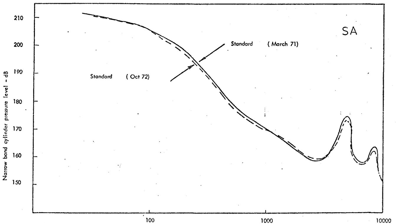
FIG. 4.25 COMPARISON OF CYLINDER PRESSURE SPECTRA FOR THE SAME MAKE AND TYPE OF ENGINE TESTED UNDER NEARLY IDENTICAL CONDITIONS @ 2000 r.p.m. FULL LOAD.
