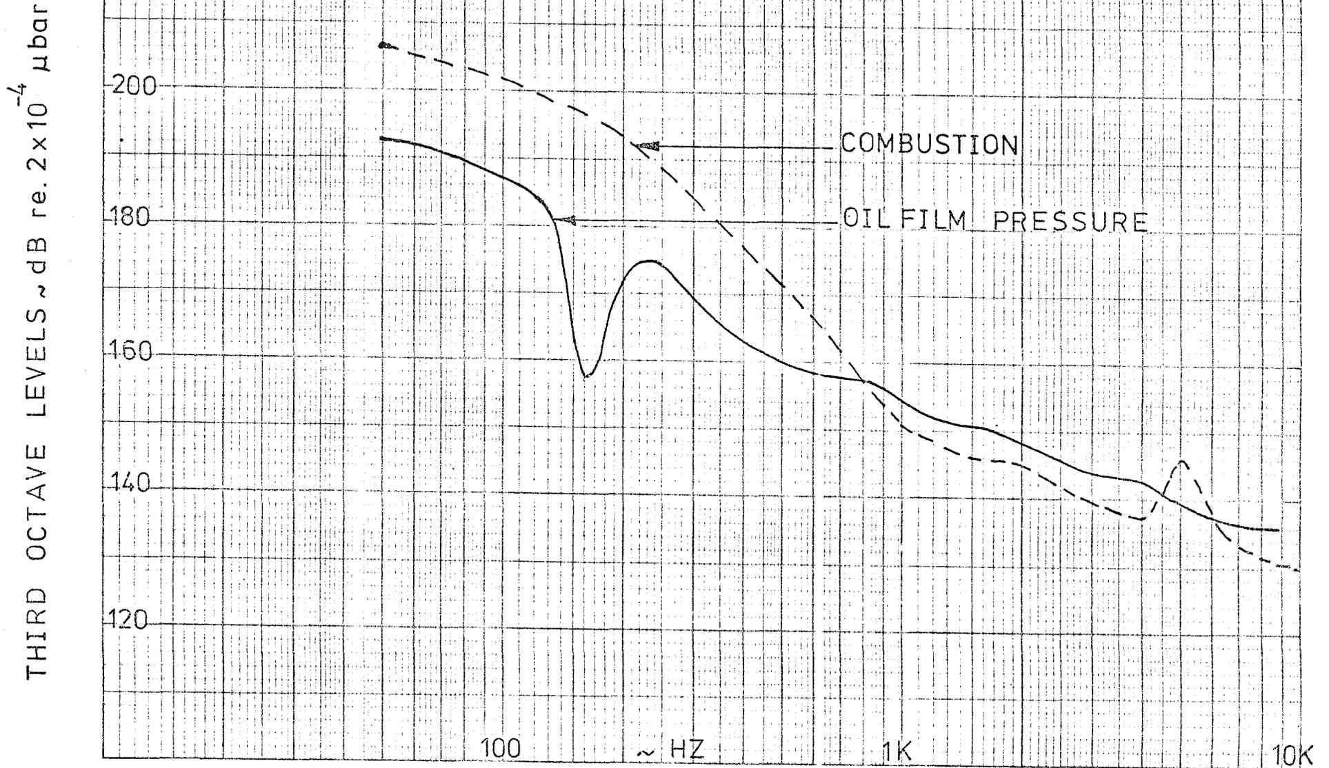
FIG. 7.24 SPECTRA OF PISTON TO BORE OIL FILM PRESSURE AND COMBUSTION FOR SA ENGINE AT 2000 RPM FULL LOAD
