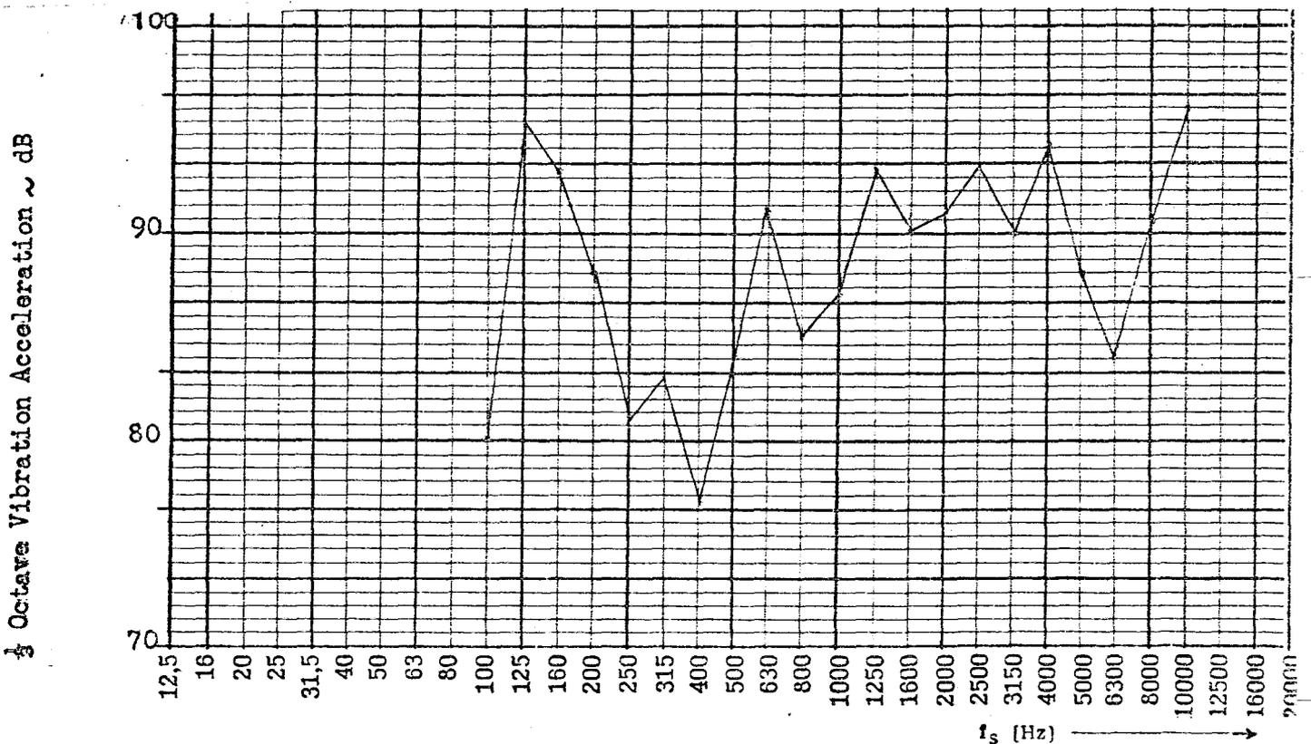
FIG. 3C Simulated Vibration Acceleration Response at  $Cl_3$  obtained on the V8-470 Piston Slap Rig at 2000 r.p.m.  $\equiv$  33.3 Hz for Full Load
