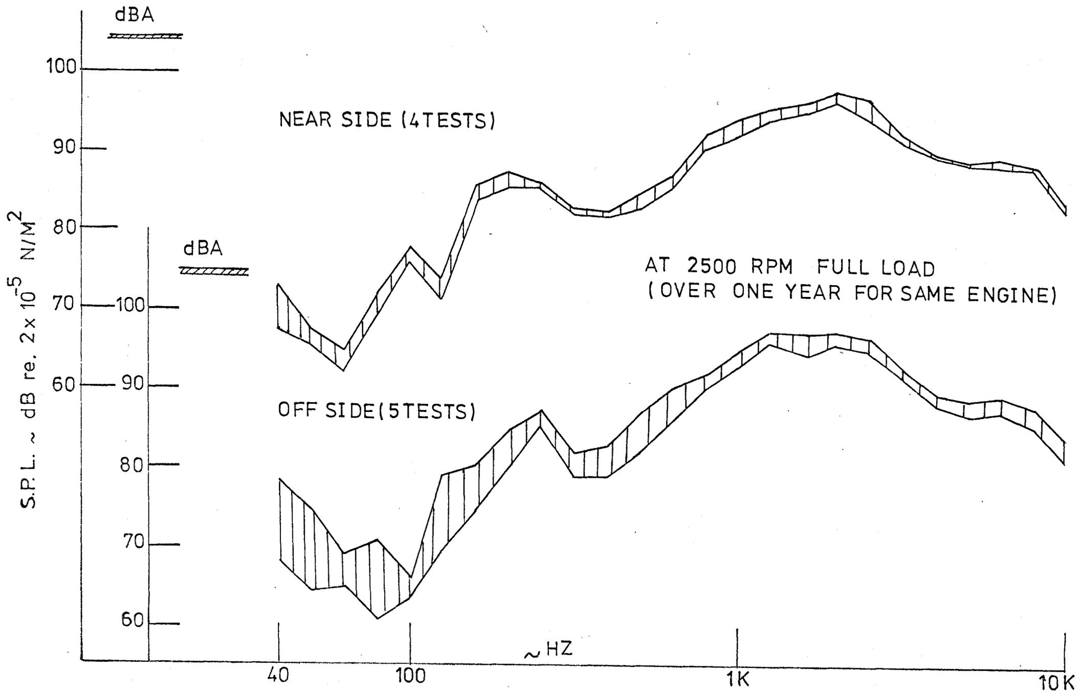
FIG. 3.2 SCATTER OF NOISE MEASUREMENTS
