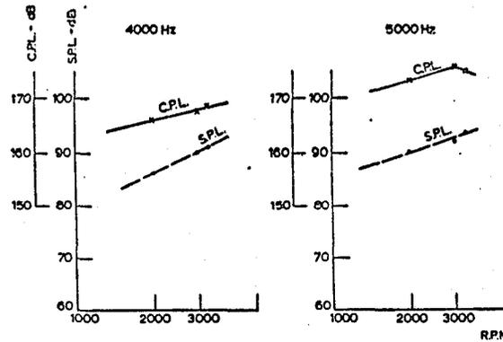
FIG. 3.13 d Variation of cylinder pressure and noise with speed for the standard engine at full load and operating temperatures - 4000 and 5000 Hz.
