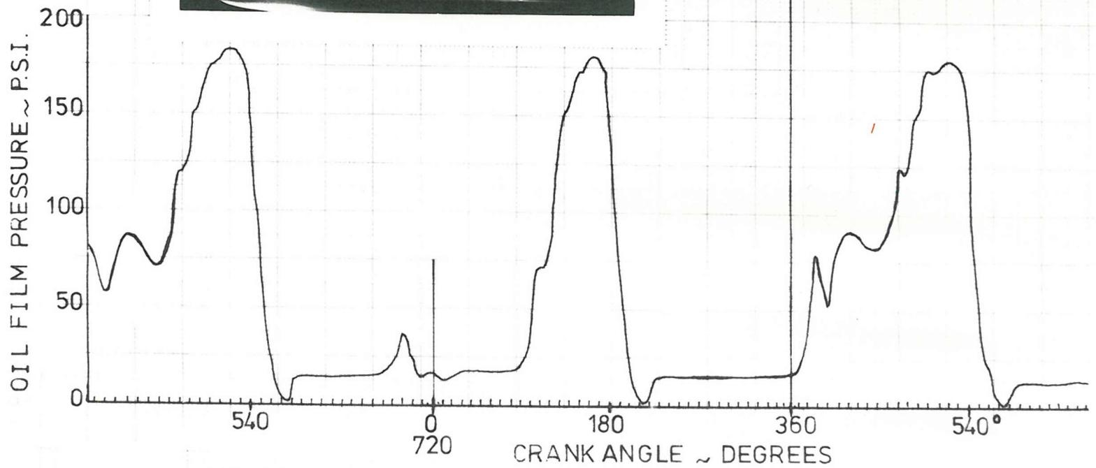
FIG. 7.7 CYLINDER PRESSURE AND PISTON TO BORE OIL FILM PRESSURE ( T.S. ) AT 2500 RPM NO LOAD - SA ENGINE
