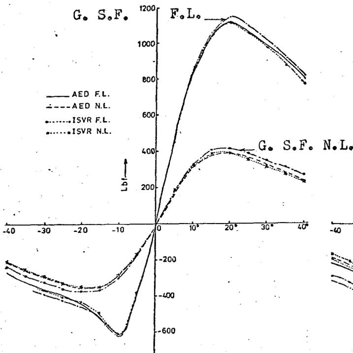
COMPARISON OF COMPUTED PISTON SIDE FORCES AROUND T.D.C. USING ISVR and AED PROGRAMMES AT 1000 RPM FULL AND NO LOAD (SA G.P.O.=0)
