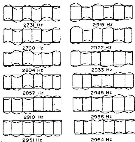
Fig. 3.16. Panel modes of a six-bay crankcase.
