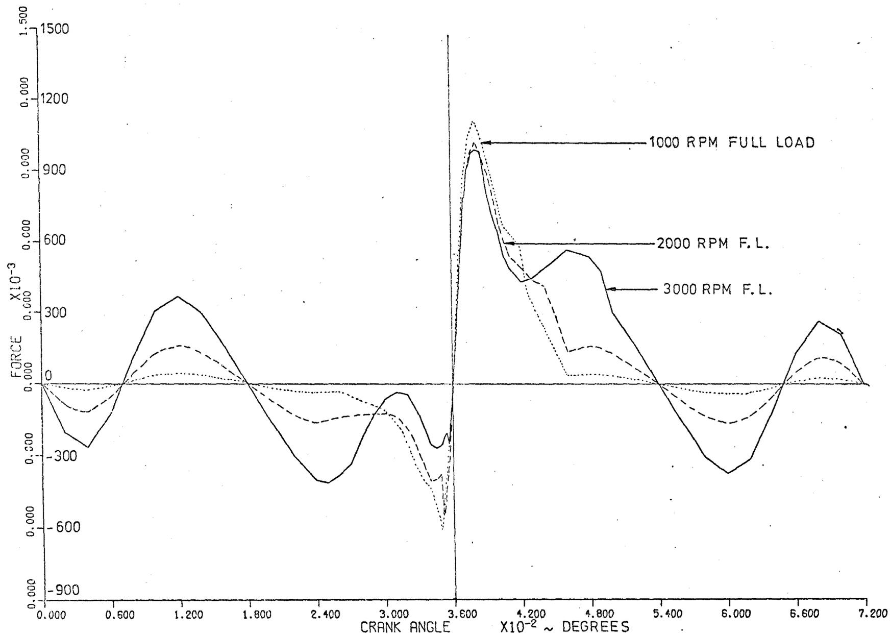
FIG. 7.17 PISTON SIDEWAYS FORCES FOR ENGINE SA
