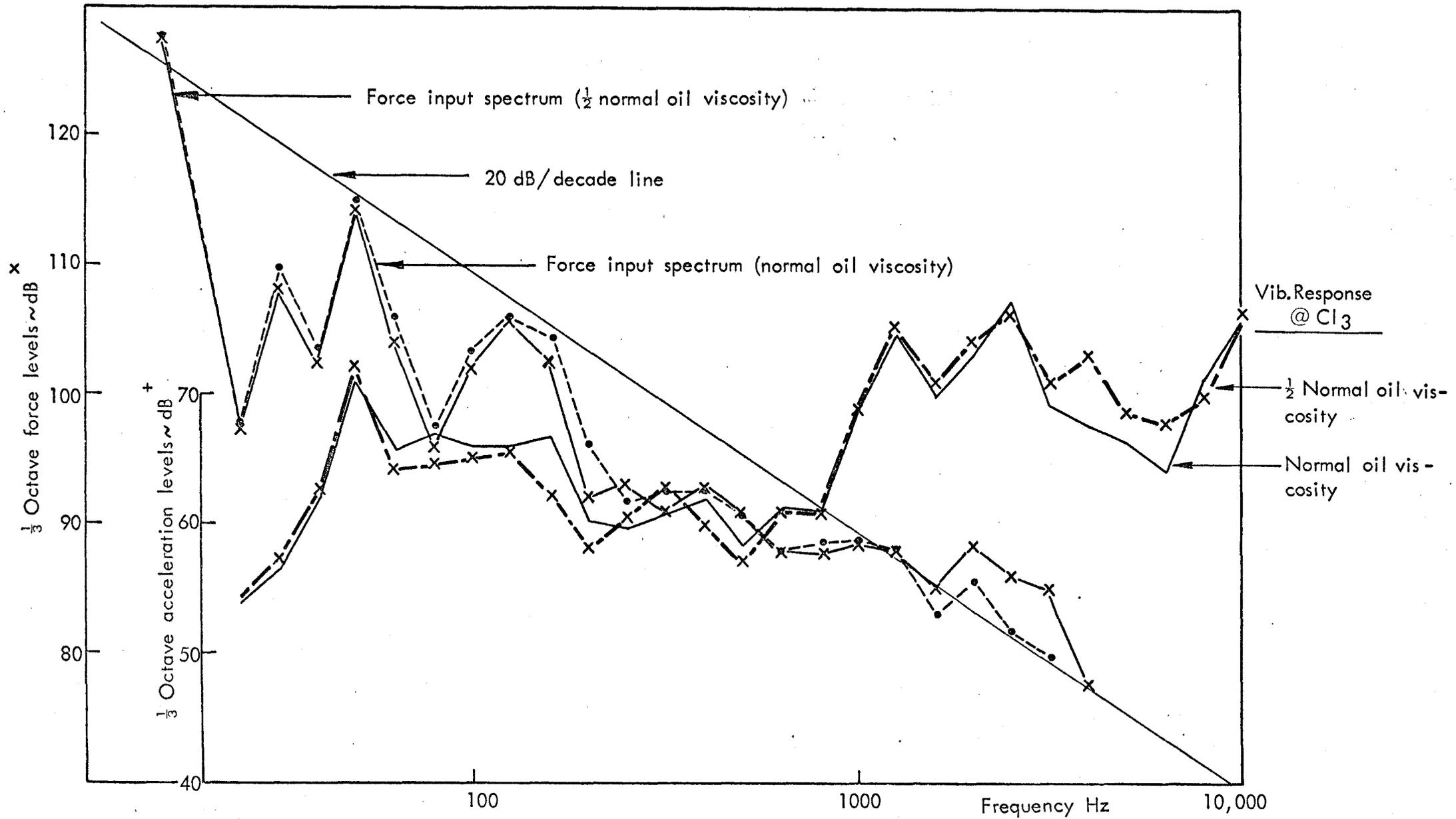
FIG. 5.34a FORCE RESPONSE SPECTRA SHOWING EFFECT OF VARYING OIL FILM VISCOSITY ON THE V8 PISTON SLAP RIG FOR THE STANDARD PISTON AT 16.7 Hz  $\approx$  1000 RPM
