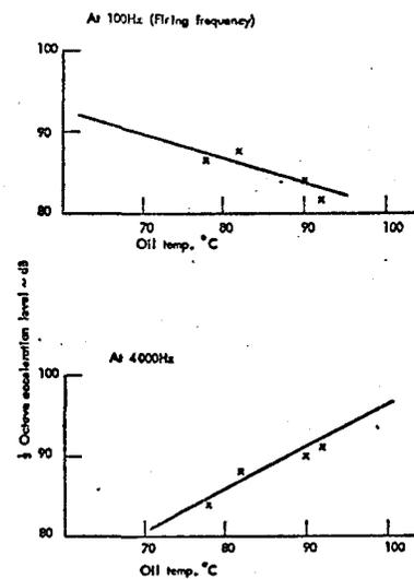
FIG. 3.11d TYPICAL LOW AND HIGH FREQUENCY CRANKSHAFT VIBRATION RESPONSE WITH OIL TEMP. FOR LNA AT 1500 r.p.m. FULL LOAD.
