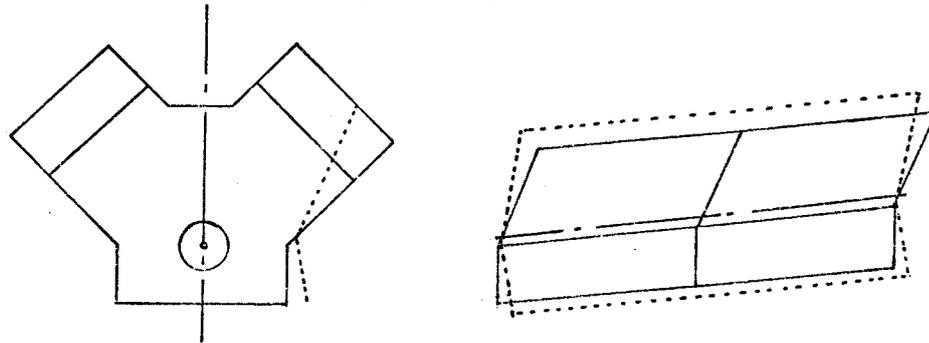
Fig. 3.17. Idealised displacement of the bank-to-bank mode on one side of a V8 engine ( $\approx 1250$  Hz for SA).
