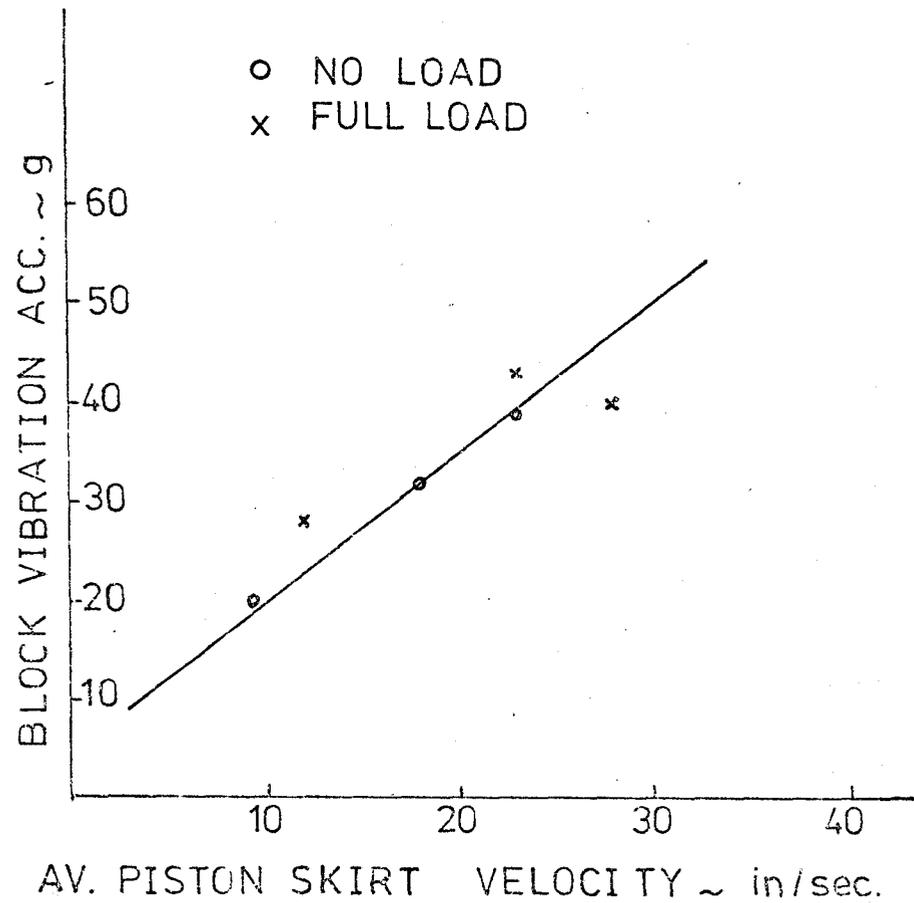
(b) TYPICAL RELATION BETWEEN PISTON IMPACT VELOCITIES AND RESULTANT ENGINE BLOCK VIBRATION - SA
