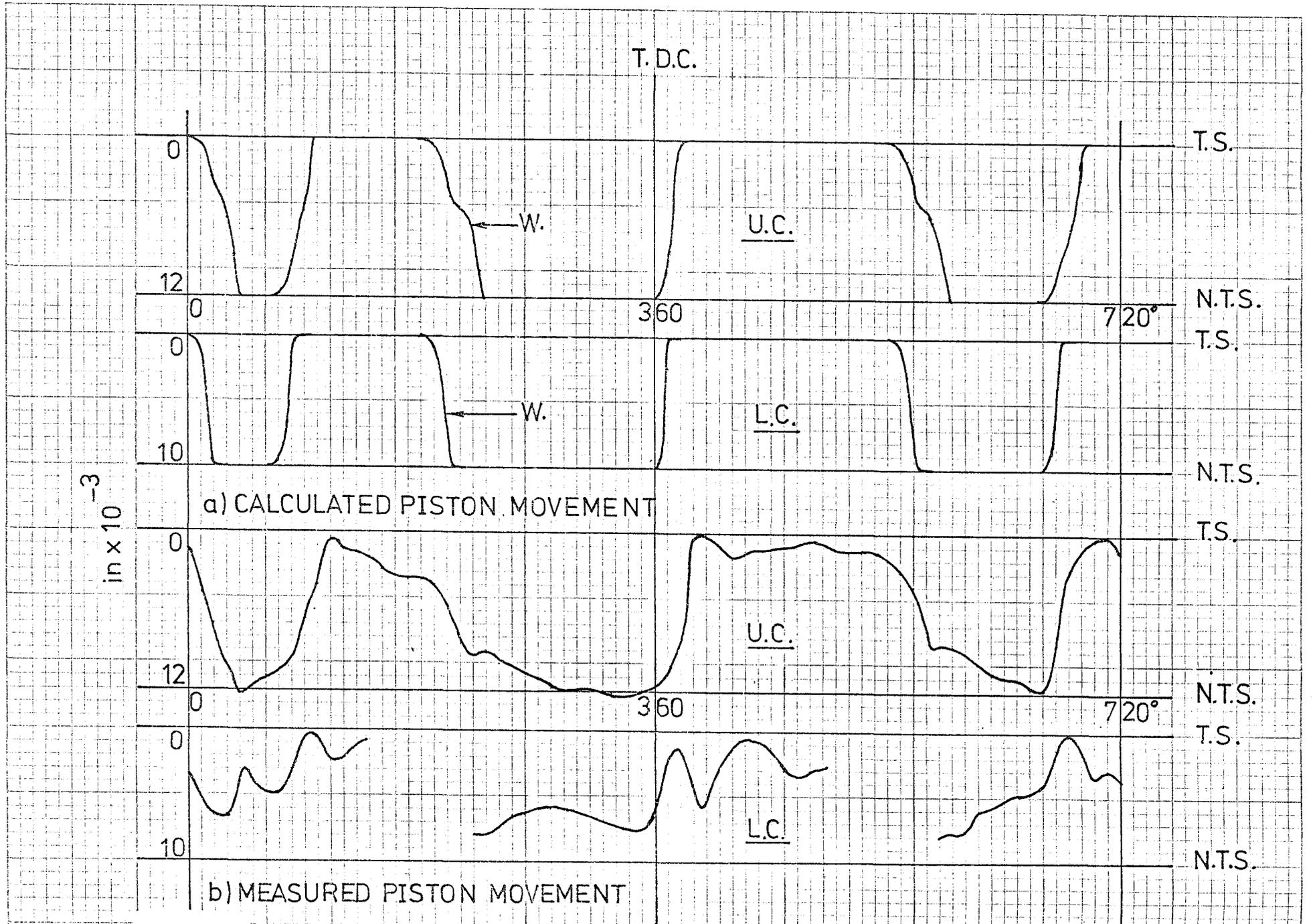
FIG. 7.34 COMPARISON OF CALCULATED AND MEASURED PISTON MOVEMENT PLOTS FOR ENGINE SA at 2500 RPM NO LOAD
