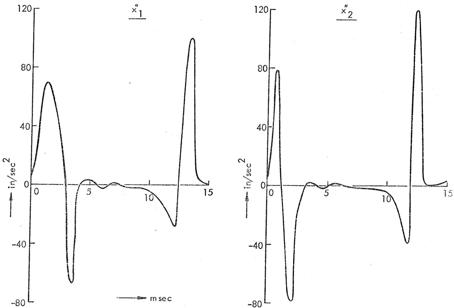
FIG 3A PISTON ACCELERATION PLOTS DERIVED FROM THE PLOTS IN 2A DUE TO A CERTAIN FORCE AT 50 Hz  $\cong$  3000 RPM (DRY CASE)
