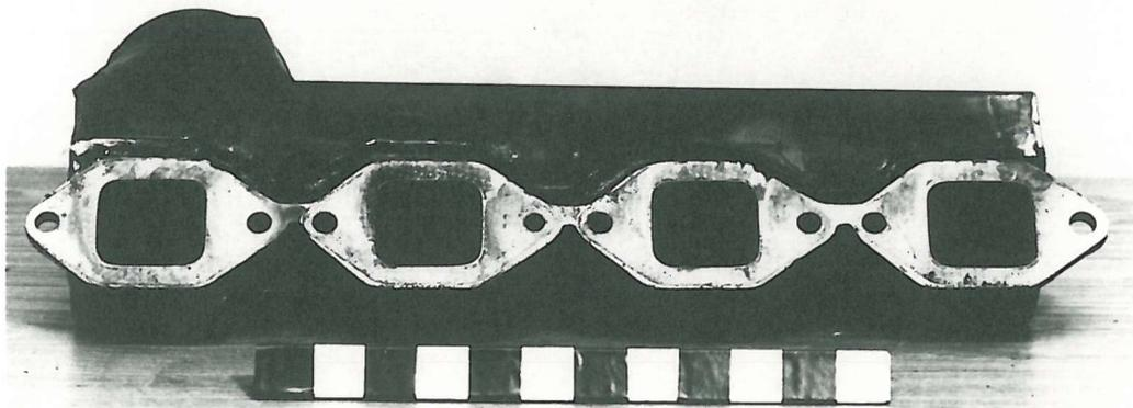
FIG. 3.22 b showing the exhaust manifold steel cover and Kao wool underneath
