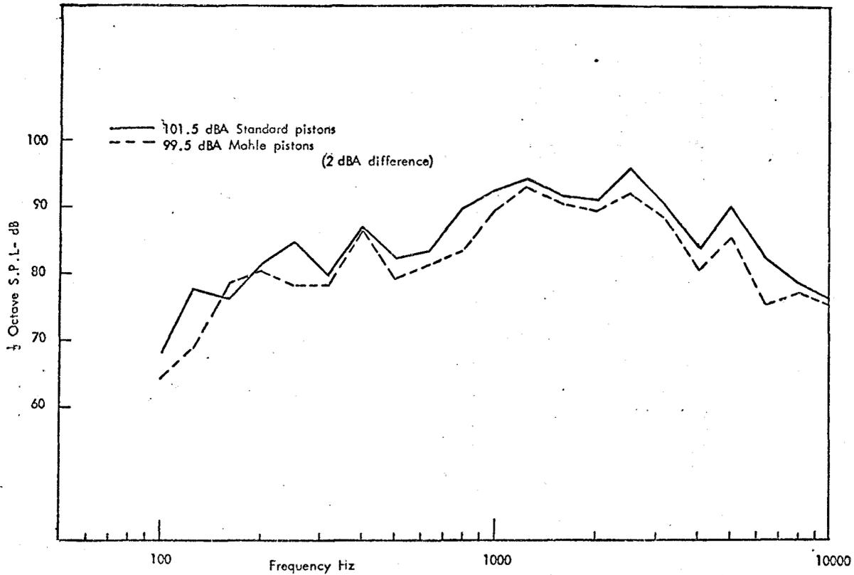
FIG. 4.4 RHS NOISE COMPARISON BETWEEN THE STANDARD AND MAHLE PISTONS FITTED ON THE ENGINE @ 2000 r.p.m. FULL LOAD. SA
