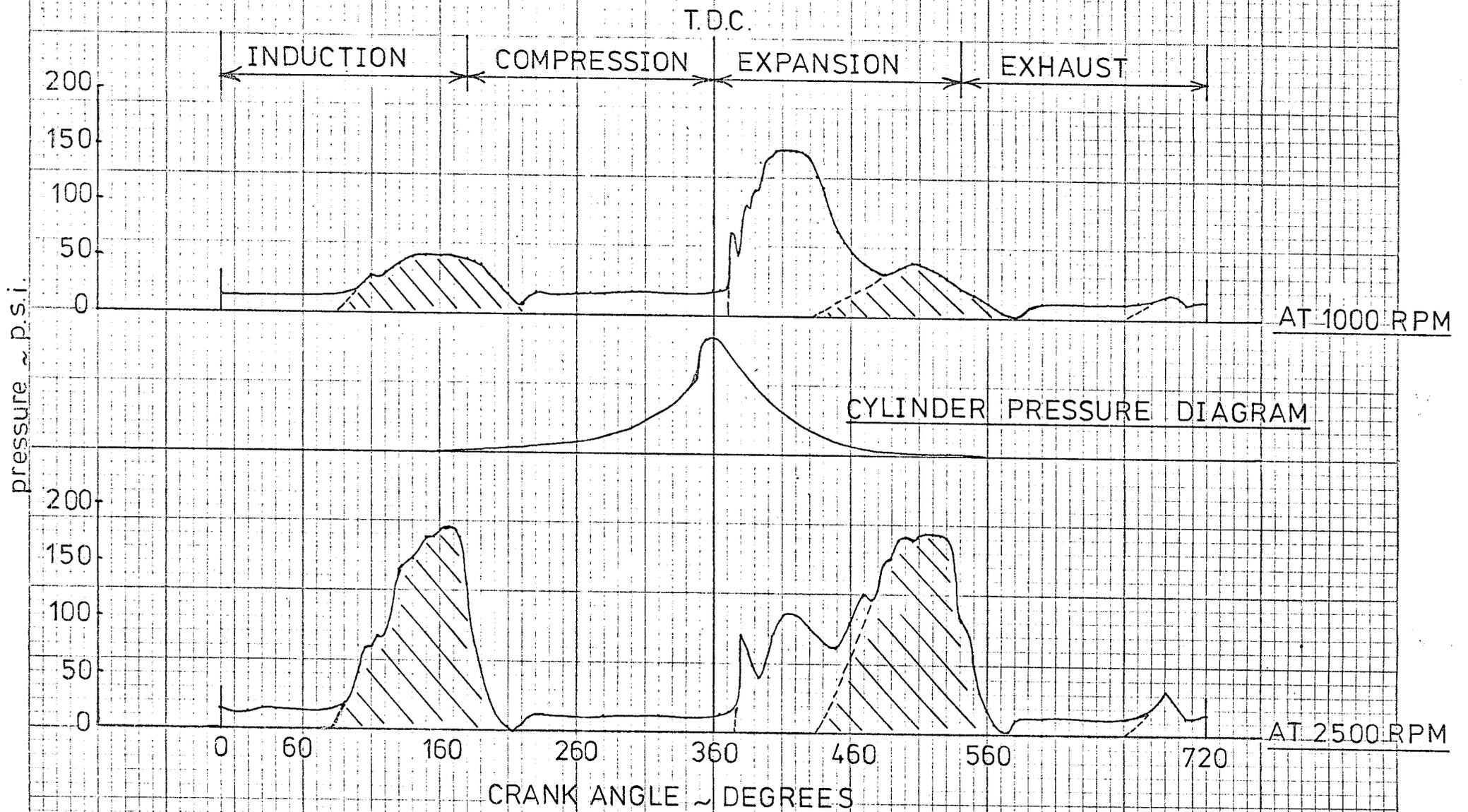
FIG. 7.14 VARIATION OF PISTON TO BORE OIL FILM PRESSURE (THRUST SIDE) WITH ENGINE SPEED AT NO LOAD FOR THE RUNNING V8 SA DIESEL ENGINE
