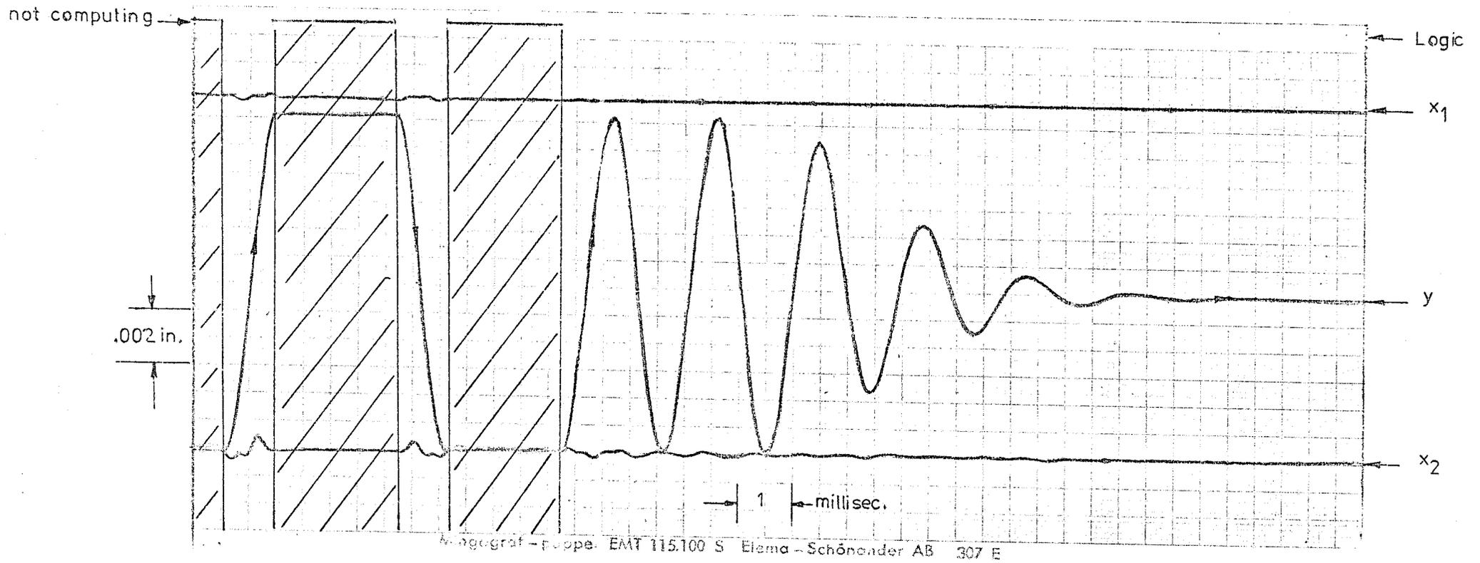
FIG. 6.7 Effect of introducing piston to block damping (artificial)
