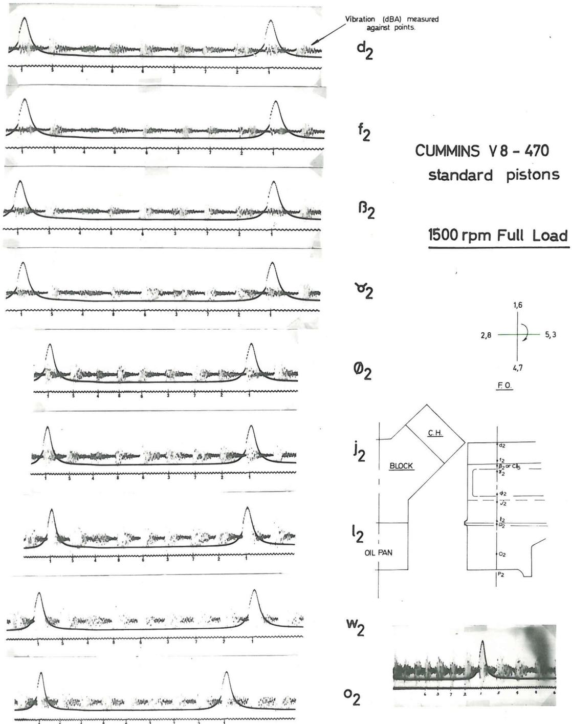
FIG. 4.11 VIBRATION CHARACTERISTICS DOWN ENGINE STRUCTURE (SA)
