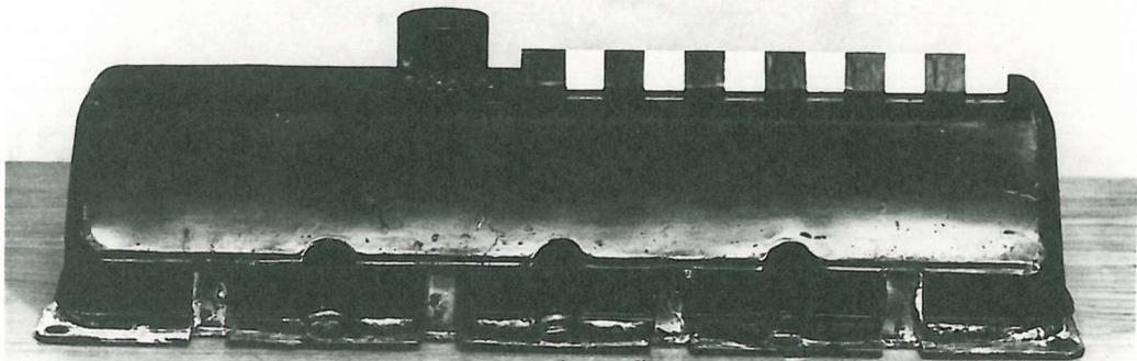
FIG. 3.21b A double skinned valve cover
