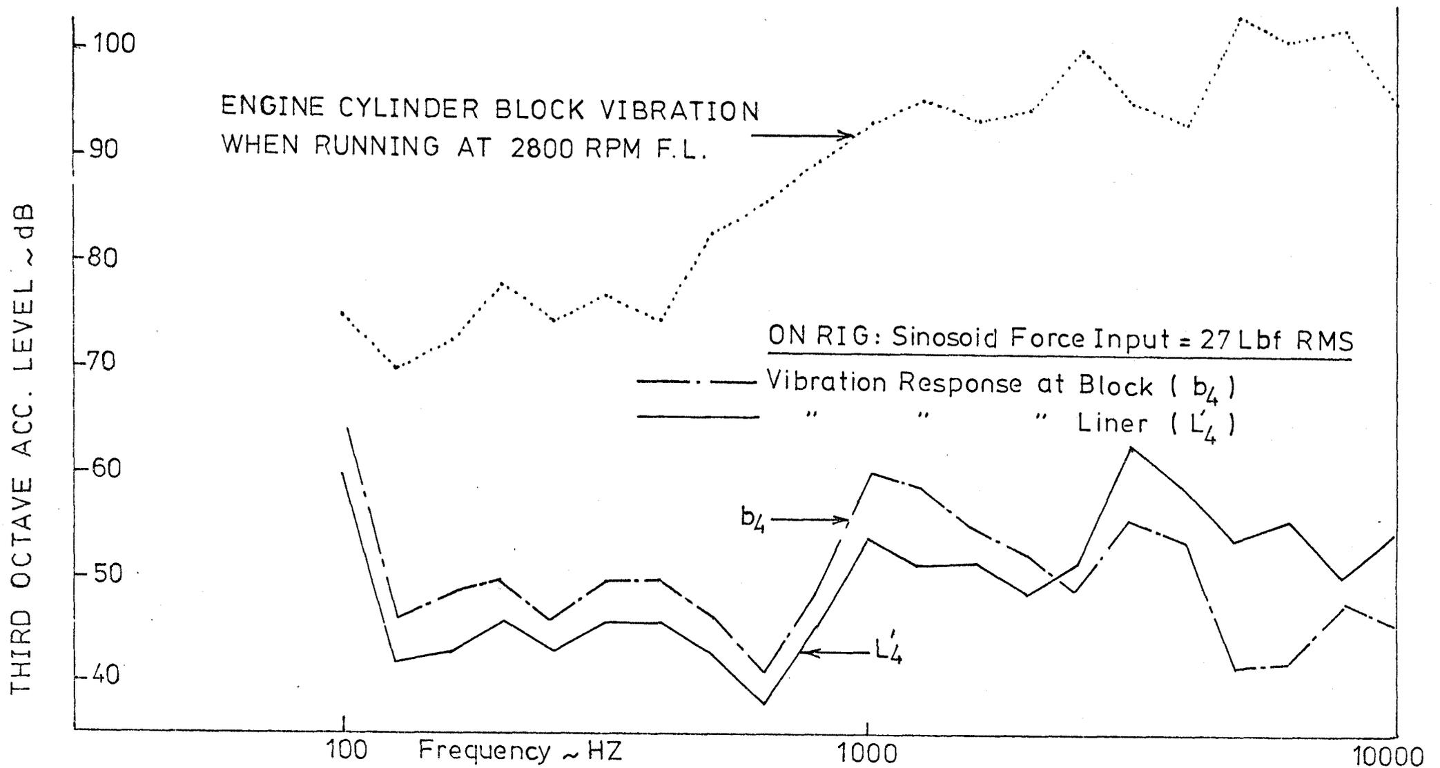
FIG. 5.6 COMPARISON OF CYLINDER BLOCK VIBRATION ON THE RUNNING ENGINE AND THE IN LINE RIG AT REPETITION RATE 46.7 per sec.  $\approx$  2800 RPM
