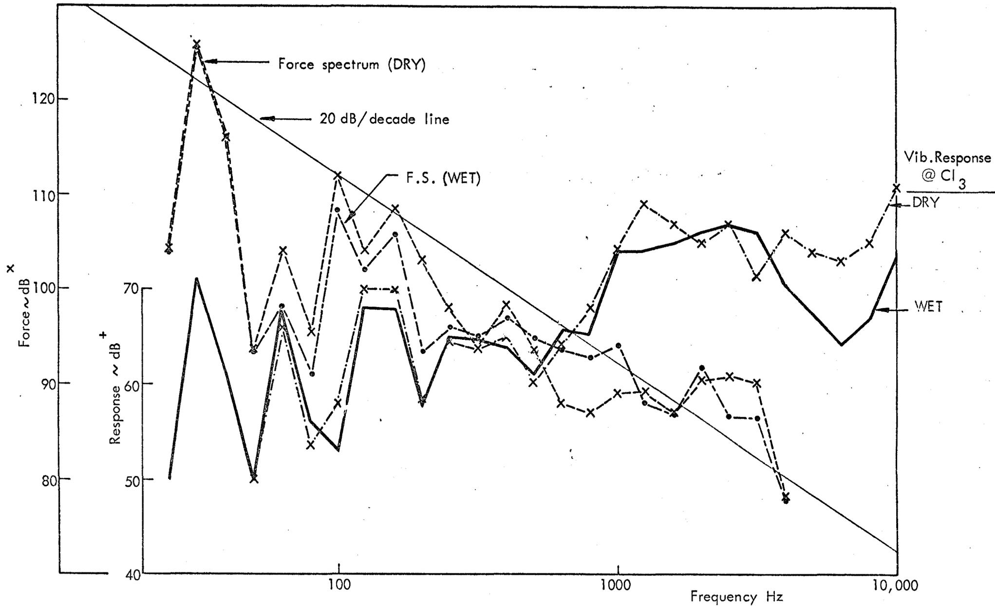
FIG. 5.30c TYPICAL EFFECT OF OIL FILM ON THE VEE RIG AT REPETITION RATE 33.3 per sec. — STANDARD PISTONS OF SA
