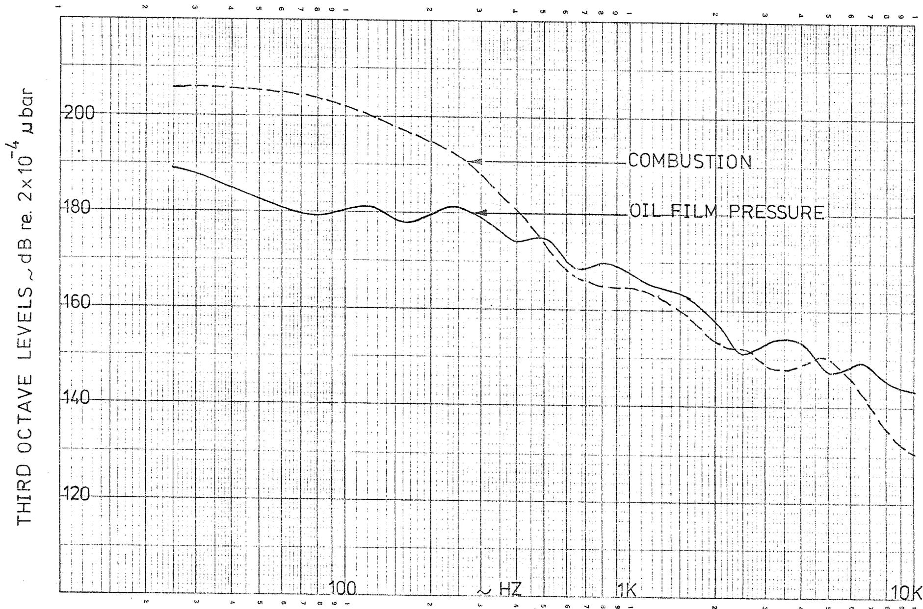
FIG. 7.22 SPECTRA OF PISTON TO BORE OIL FILM PRESSURE AND COMBUSTION FOR THE SA ENGINE AT 3000 RPM NO LOAD
