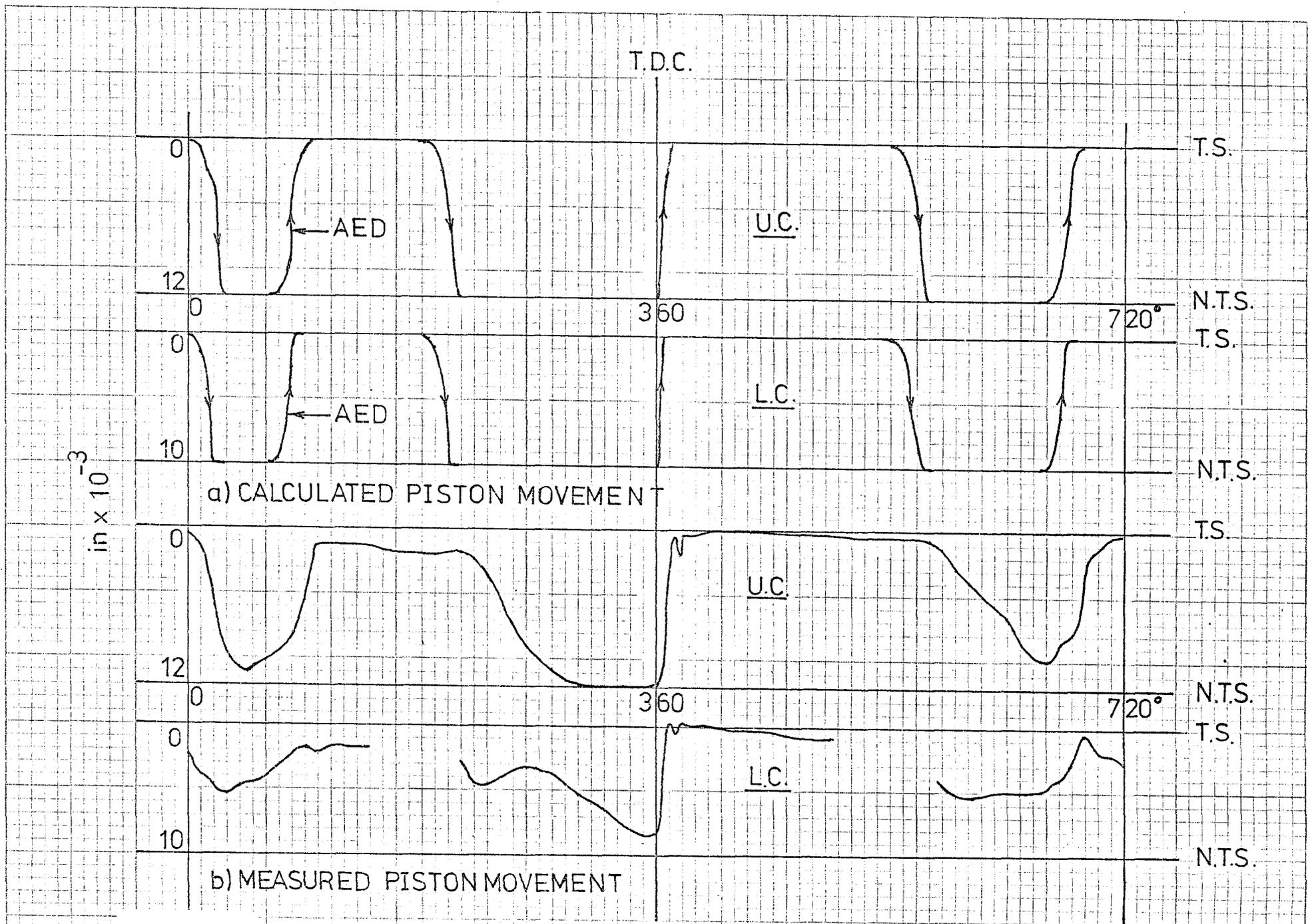
FIG. 7.35 COMPARISON OF CALCULATED AND MEASURED PISTON MOVEMENT PLOTS FOR ENGINE SA at 1000 RPM FULL LOAD
