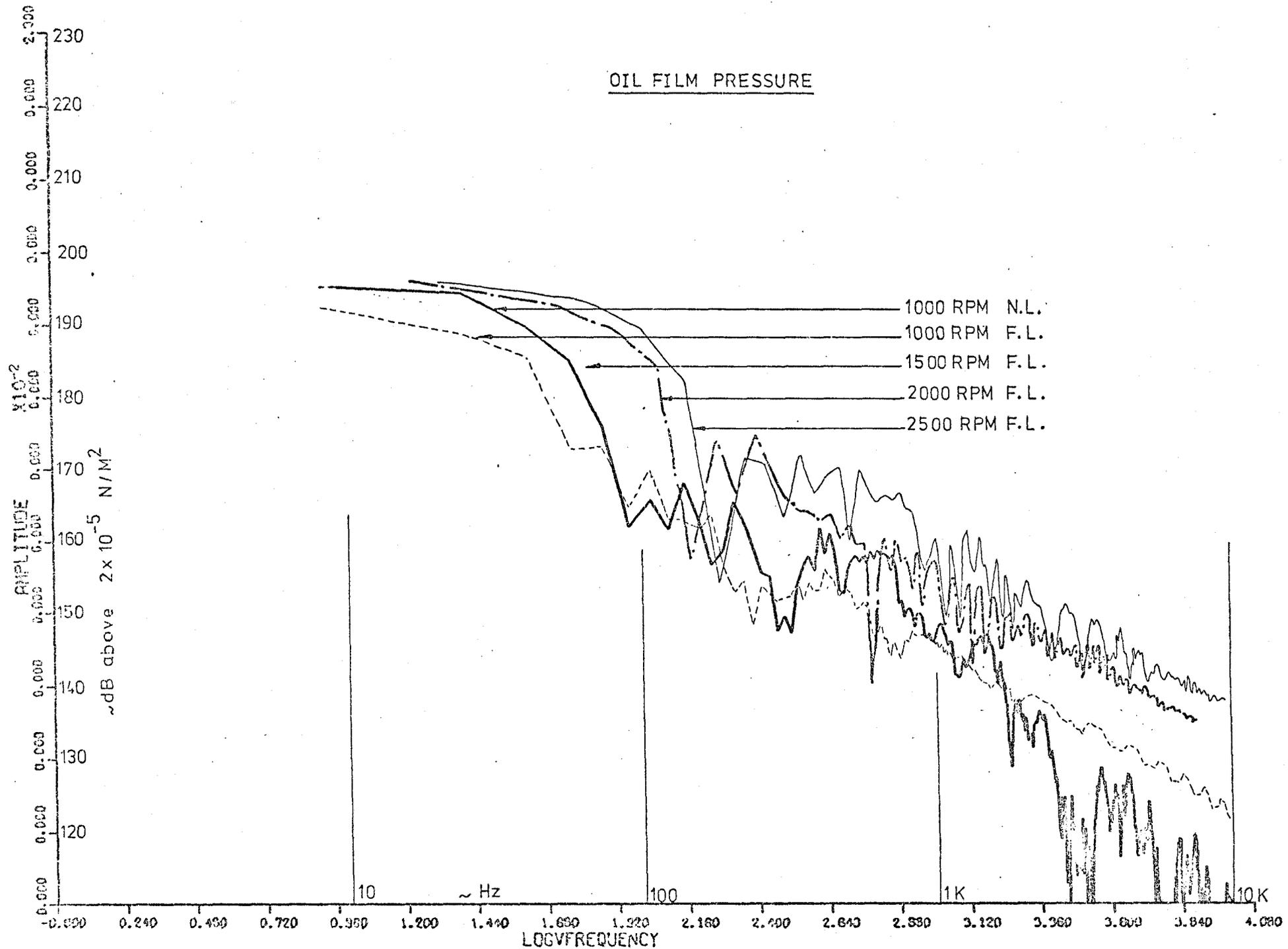
FIG. 7.19 NARROW BAND SPECTRA OF PISTON TO BORE OIL FILM PRESSURES - SA
