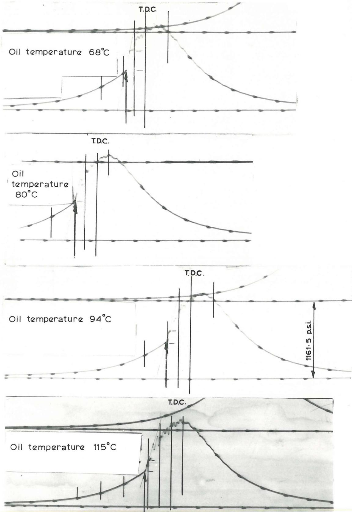
Fig. 3.6 Variation of cylinder pressure diagrams with oil temperature for the SA engine at 3000 r.p.m. full load.
