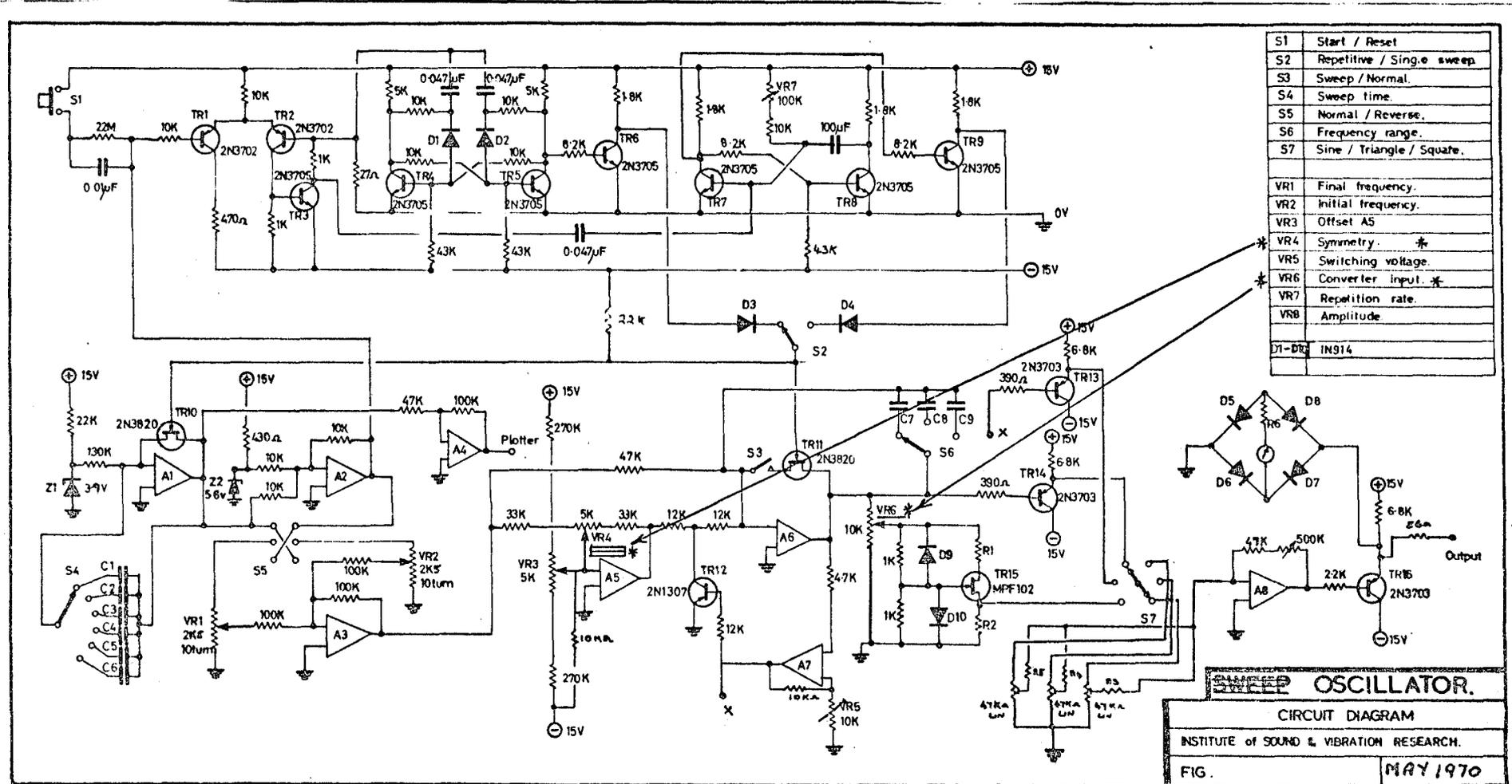
FIG. 5.14 CIRCUIT DIAGRAM OF THE SPECIAL OSCILLATOR USED TO SIMULATE PISTON SIDWAYS FORCE ON THE VEE PISTON SLAP RIG — ENGINE SA
