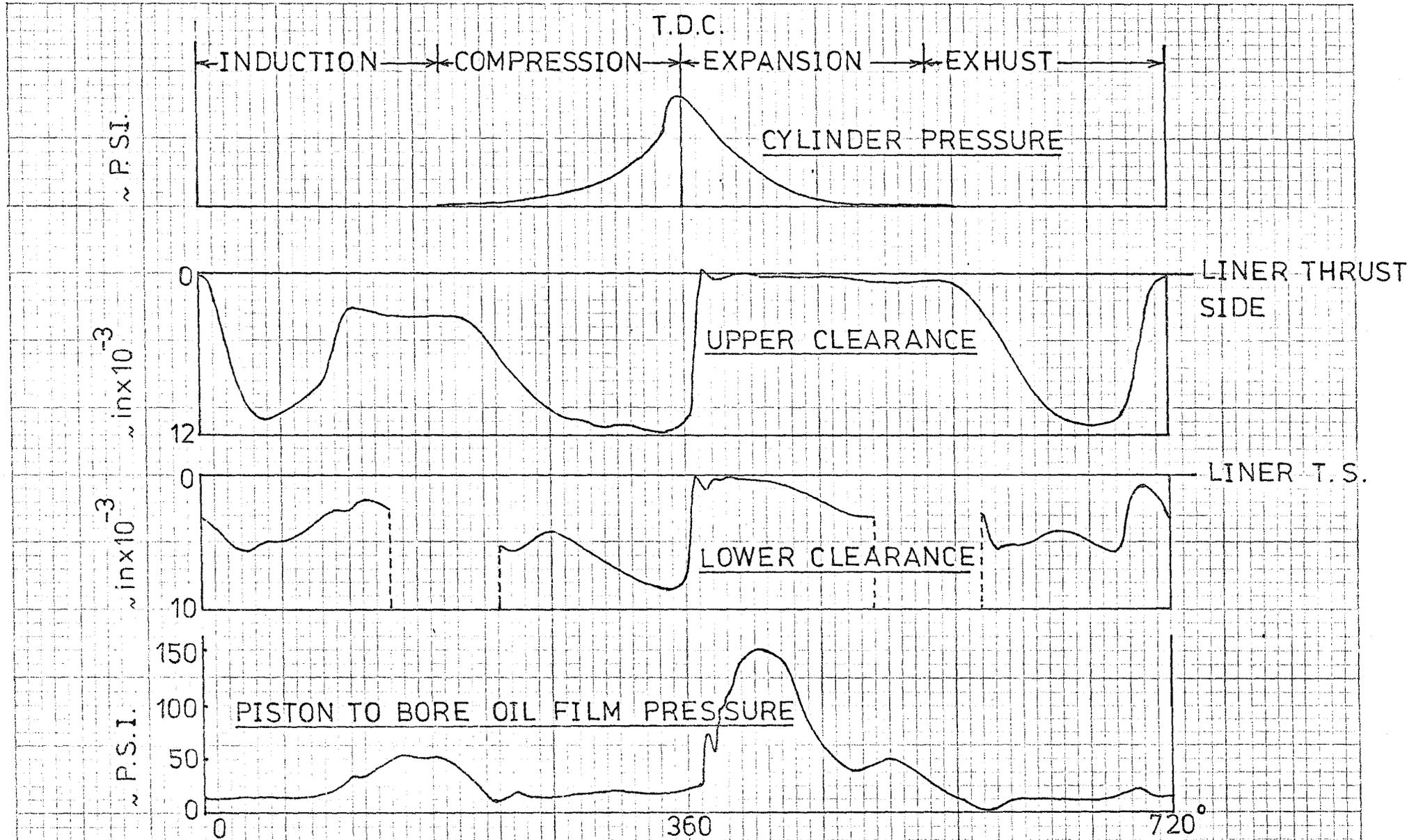
FIG. 7.30 RELATION BETWEEN CYLINDER PRESSURE, PISTON MOVEMENT AND PISTON TO BORE OIL FILM PRESSURE IN NO1 CYLINDER AT 1000 RPM NO LOAD. (ENGINE SA)
