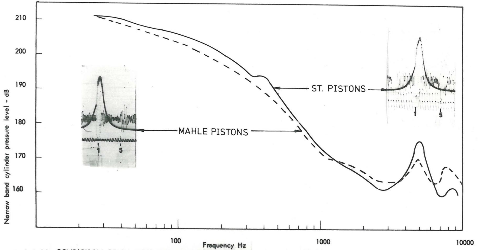
FIG. 4.21 COMPARISON OF CYLINDER PRESSURE SPECTRA FOR THE SA ENGINE FITTED WITH STANDARD AND MAHLE PISTONS @ 3000 r.p.m. FULL LOAD.
