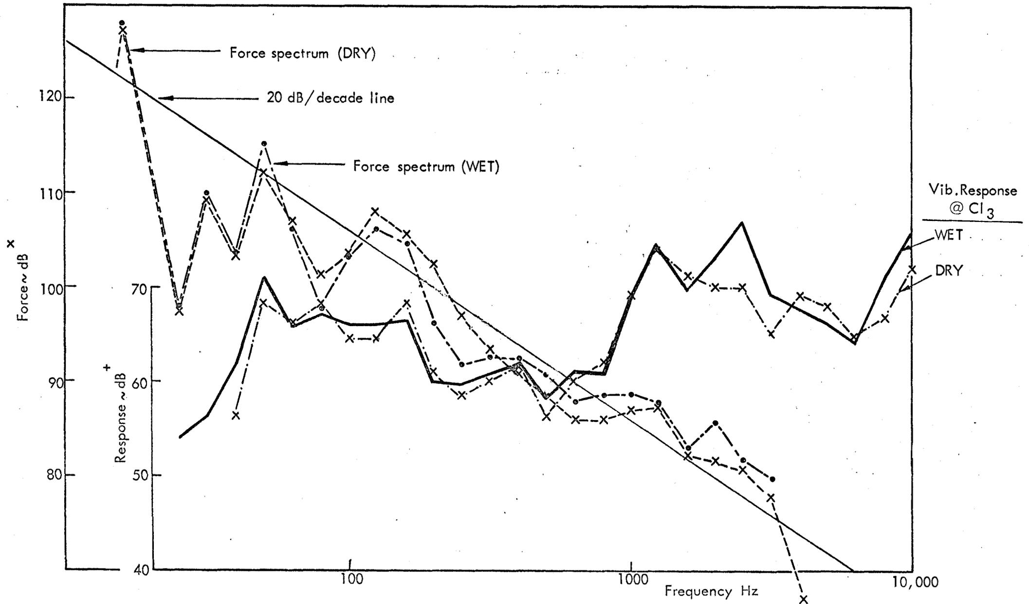
FIG. 5.30a TYPICAL EFFECT OF OF OIL FILM ON THE VEE RIG AT REPETITION RATE 16.7 per sec. - STANDARD PISTONS OF SA
