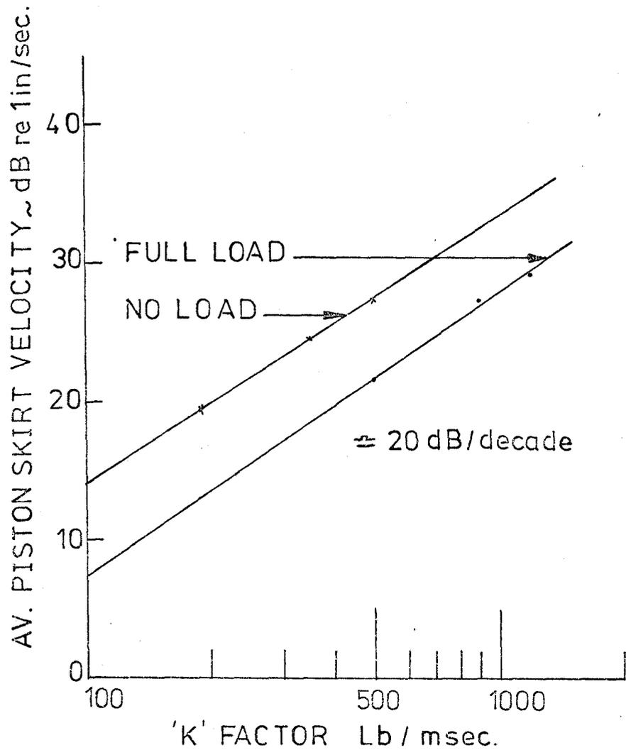
(a) RELATION BETWEEN AVERAGE PISTON IMPACT VELOCITY AND 'K' FACTOR — ENGINE SA
