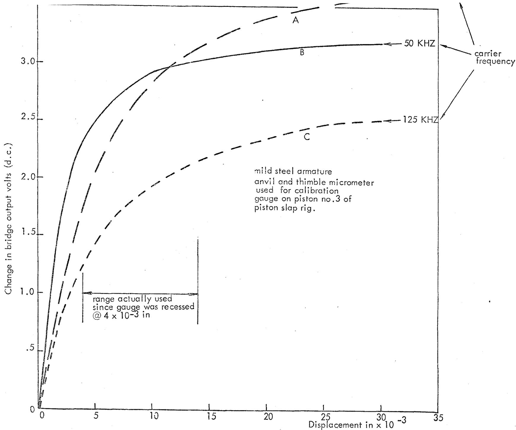
FIG. 2F CALIBRATION OF LOWER CLEARANCE AET 4 INDUCTIVE GAUGE
