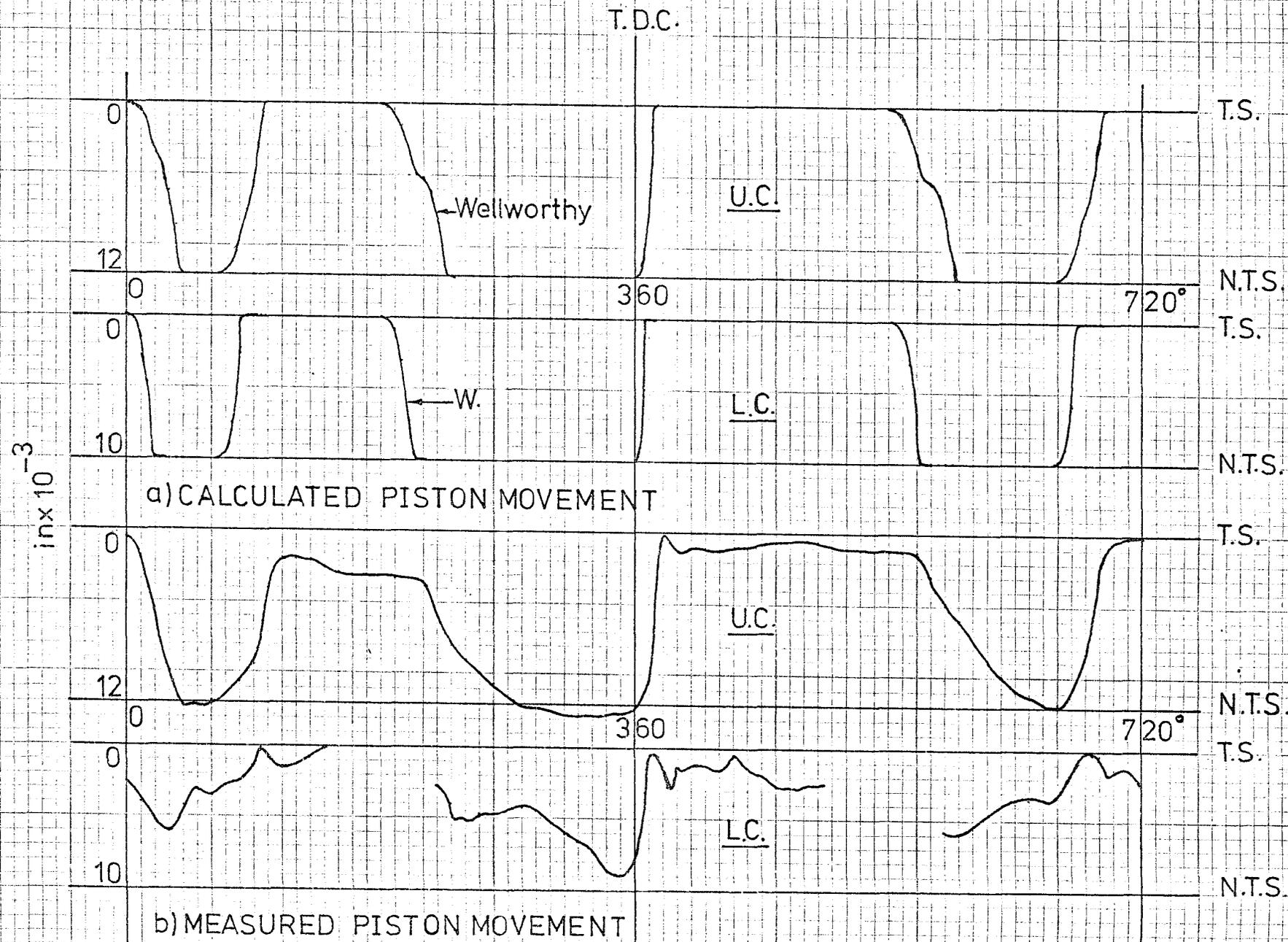
FIG. 7.32 COMPARISON OF CALCULATED AND MEASURED PISTON MOVEMENT PLOTS FOR ENGINE SA at 1500 RPM NO LOAD
