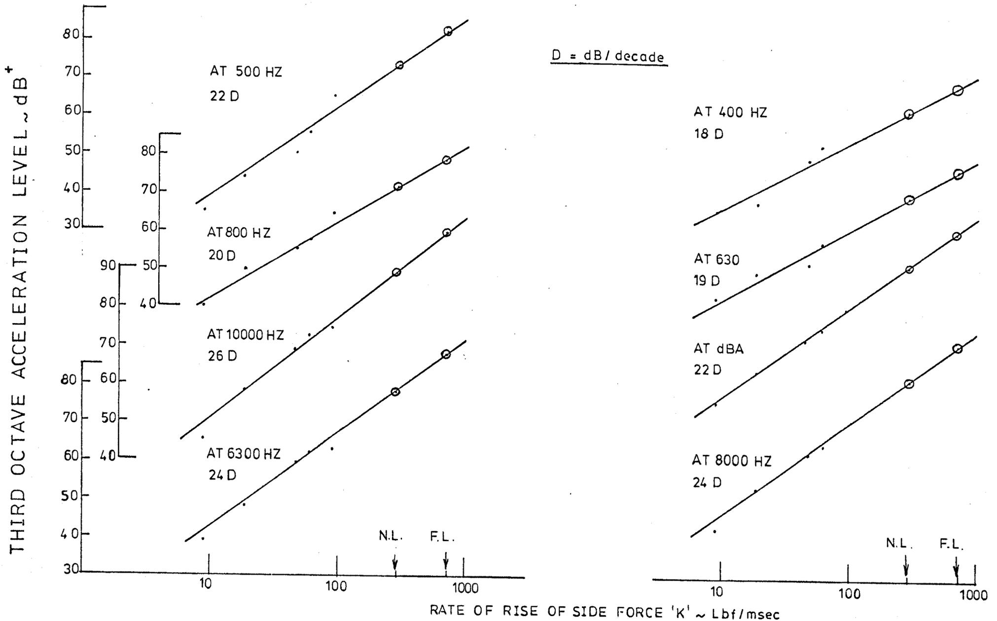
FIG. 5.22 RELATION BETWEEN VIBRATION RESPONSE AT  $Cl_3$  AND K FACTOR AT REPETITION RATE 25 per sec.  $\cong$  1500 RPM ENGINE SPEED (SA)
