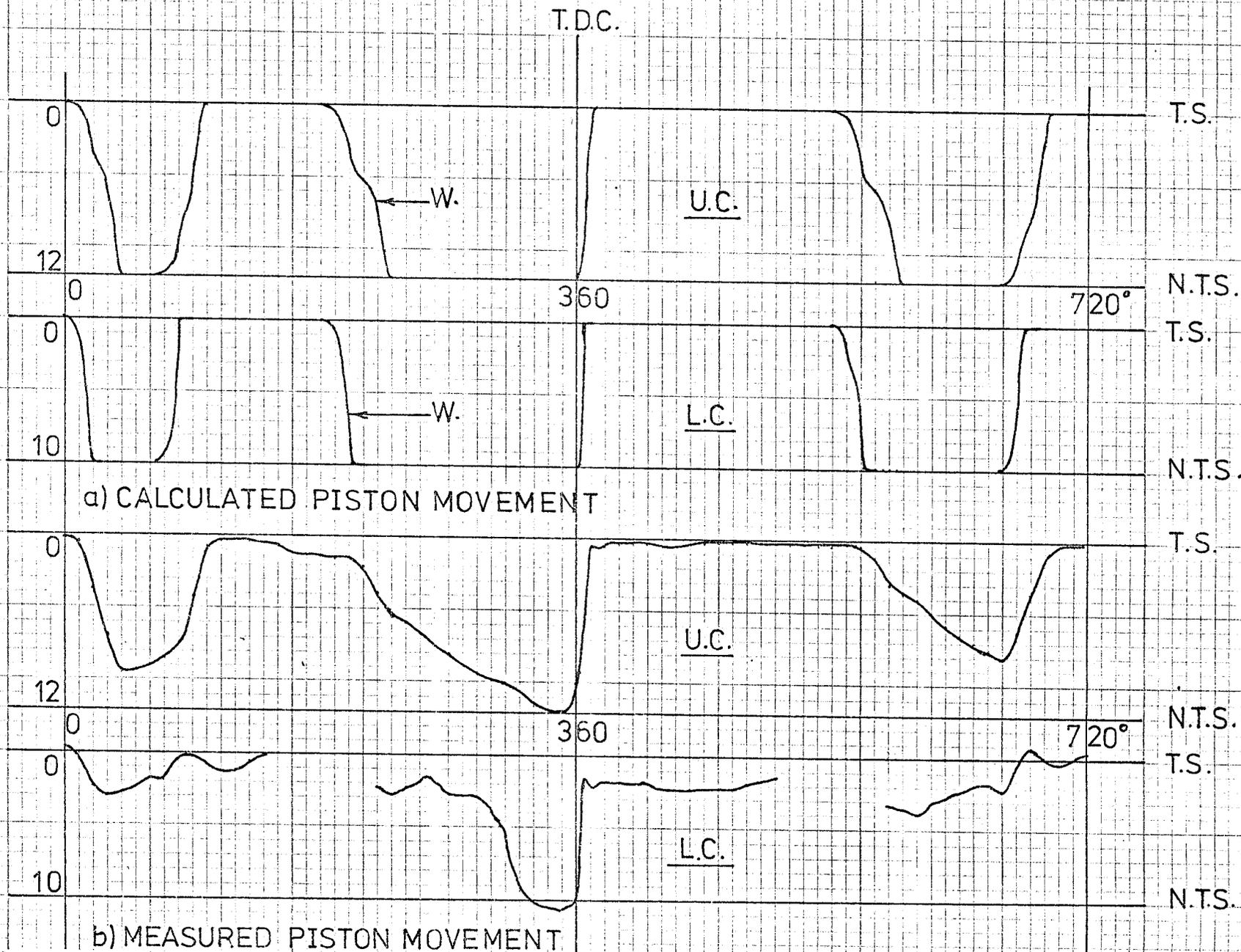
FIG. 7.36 COMPARISON OF CALCULATED AND MEASURED PISTON MOVEMENT PLOTS FOR ENGINE SA at 1500 RPM FULL LOAD
