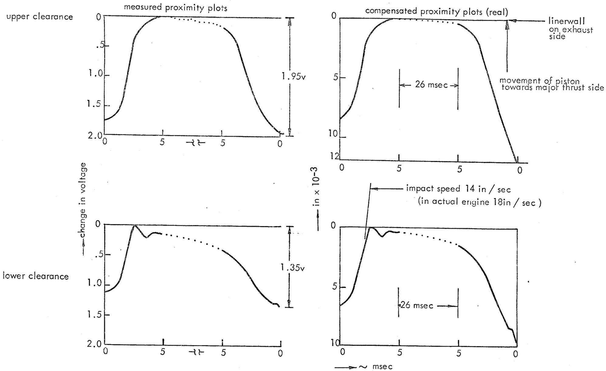
FIG. 3F PISTON MOVEMENT @ 16.7 HZ  $\approx$  1000 rpm DRY CASE — PISTON SLAP RIG —
