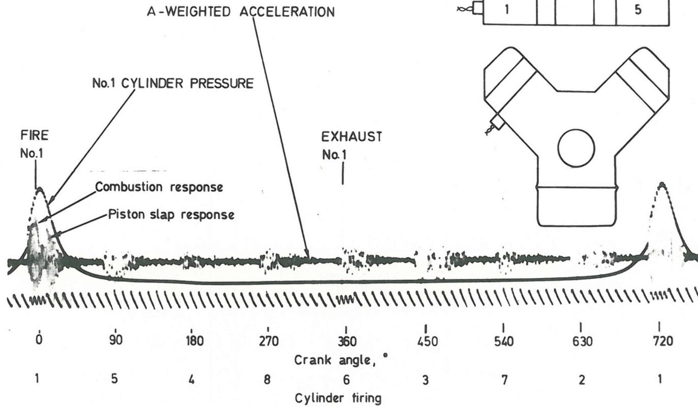
FIG. 4.9 Piston Slap Contribution to Cylinder Block Vibration IN a Running Engine
