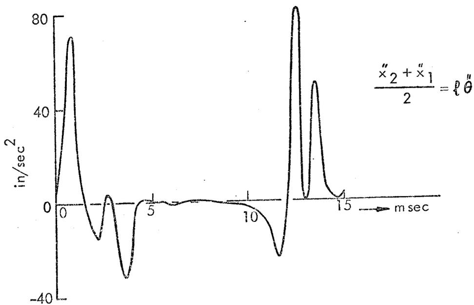
FIG 4A GRAPHICAL DERIVATION OF  $l\theta''$  FROM PLOTS OF 3A DUE TO A CERTAIN FORCE AT 50 Hz  $\equiv$  3000 RPM .
