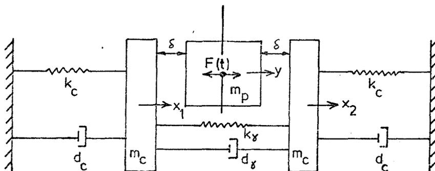
SKETCH (1). Simple Model of Piston-liner Movement Around TDC.
