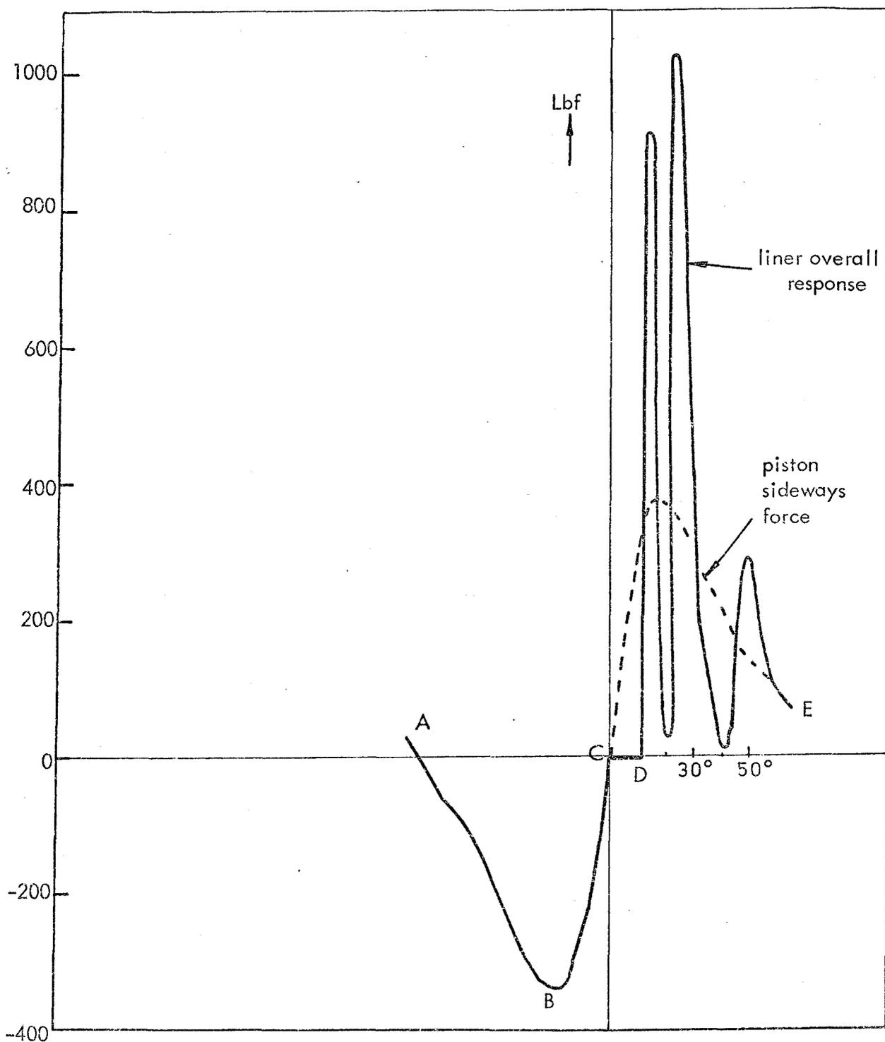
FIG. 2H RESULTANT LINER OVERALL RESPONSE DUE TO PISTON IMPACT
