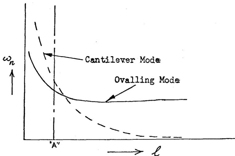
For short cylinders as at "A",  $\omega_n$  cantilever mode  $>$   $\omega_n$  ovalling mode
