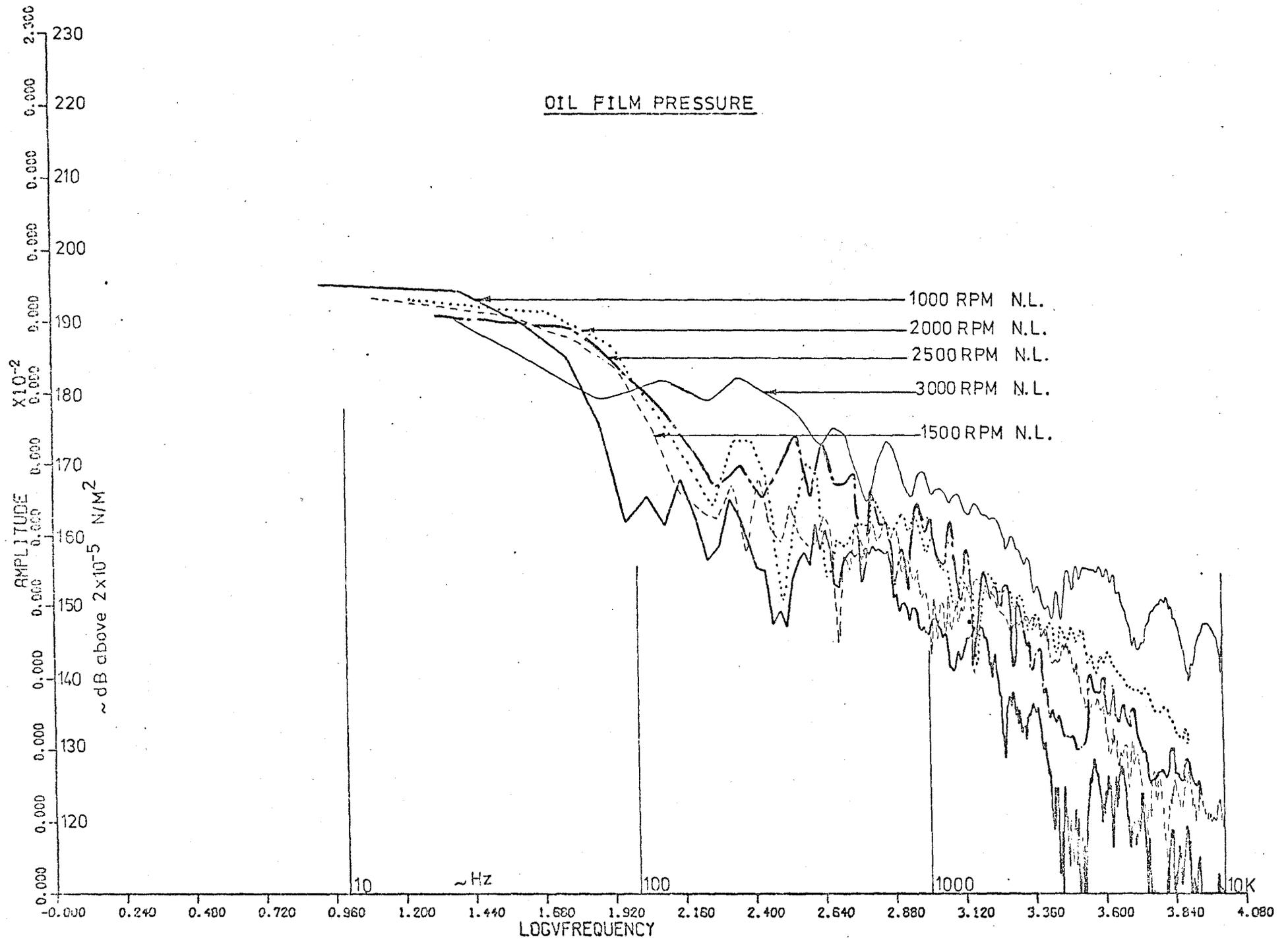
FIG. 7.18 NARROW BAND SPECTRA OF PISTON TO BORE OIL FILM PRESSURES - SA
