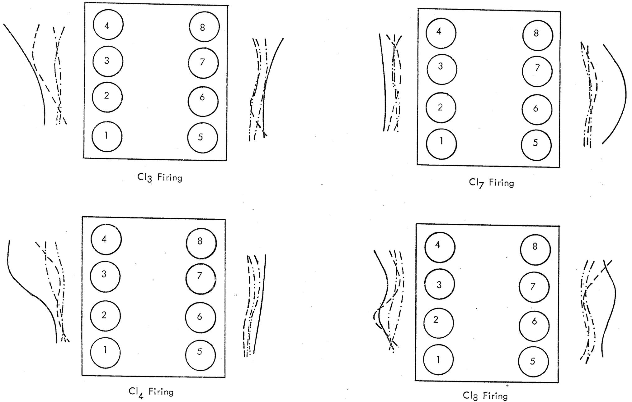
FIG. 4.20 MAXIMUM VIBRATION AMPLITUDES FOR SA ENGINE MAHLE @ 3000 r.p.m.
