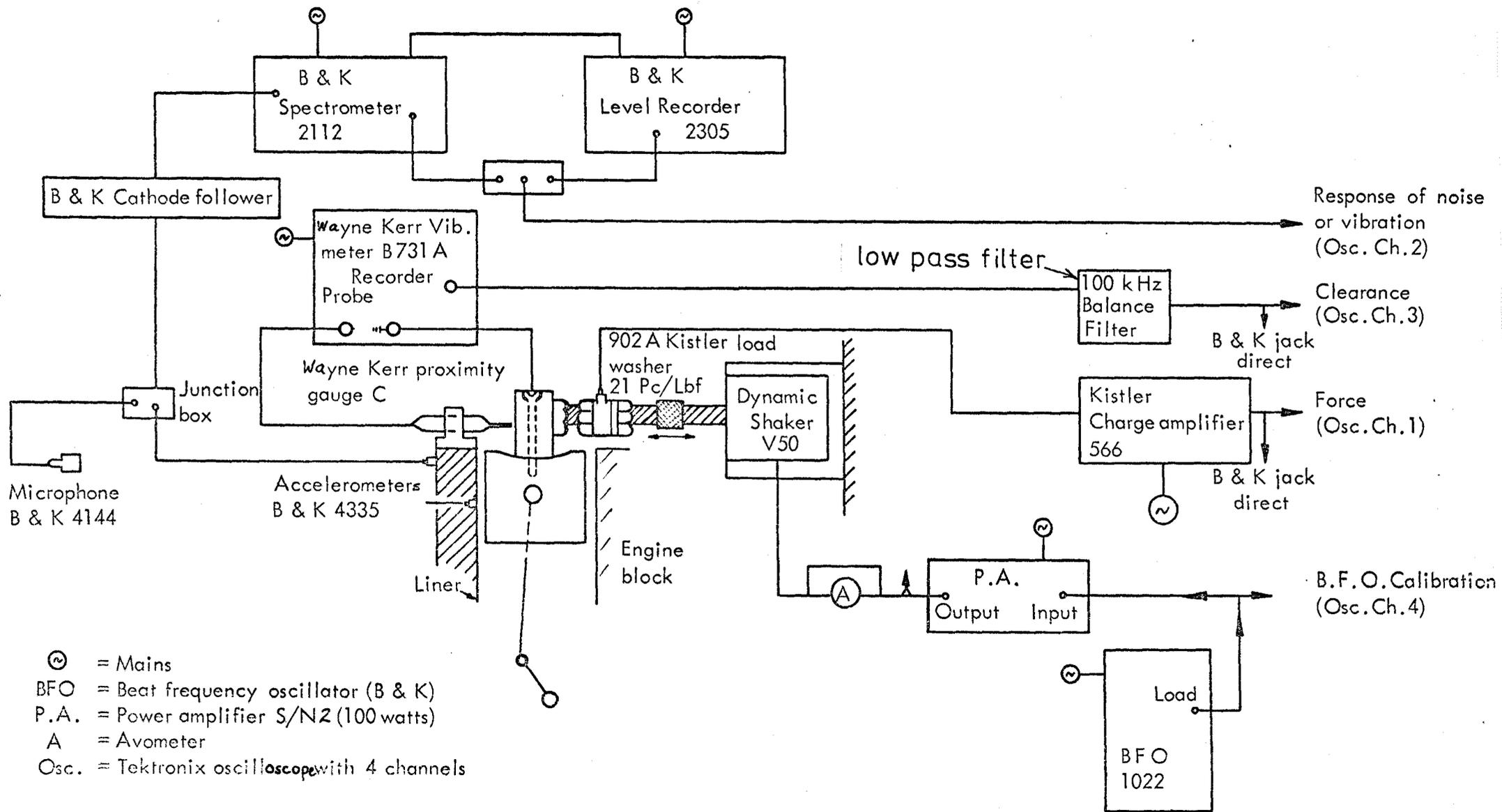
FIG. 5.2 LAYOUT OF INSTRUMENTATION AND CIRCUIT DIAGRAM FOR THE STUDY OF PISTON SLAP SIMULATION ON A SIX CYLINDER IN-LINE DIESEL ENGINE
