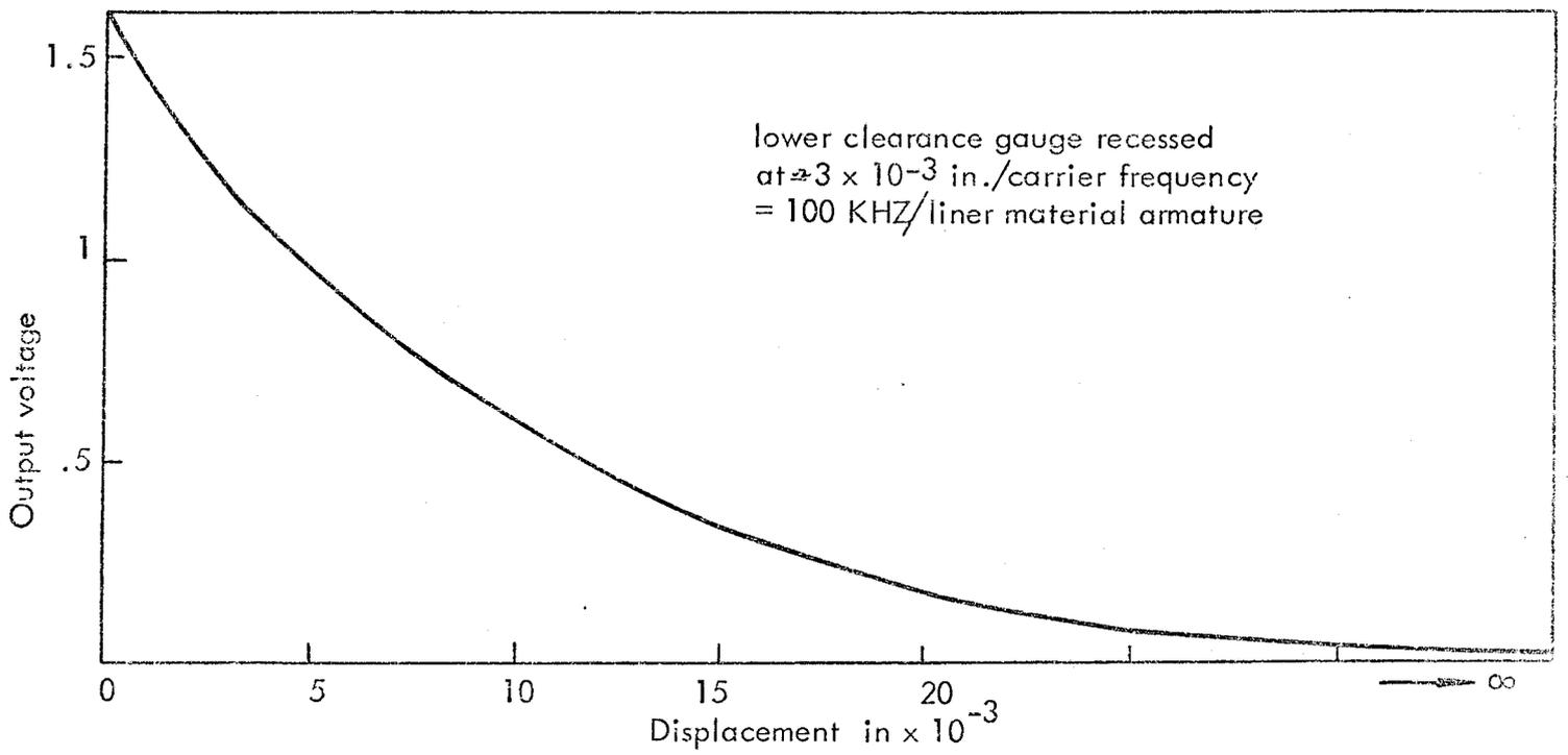
FIG. 5F CALIBRATION CURVES OF THE TWO AET 4 PROXIMITY GAUGES INSTALLED IN PISTON 1 OF V8 - 7.7 LITRE RUNNING ENGINE "WITH LINKAGE"
