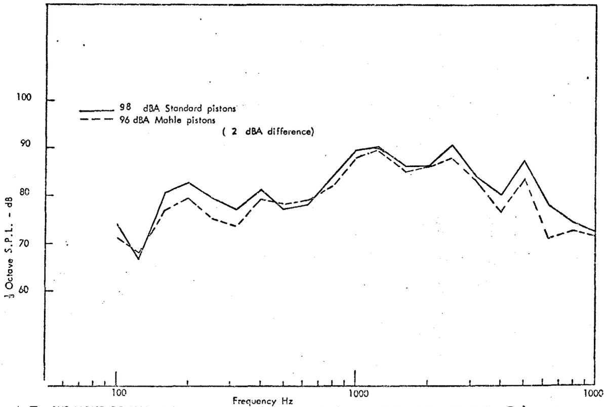
FIG. 4.5 RHS NOISE COMPARISON BETWEEN THE STANDARD AND MAHLE PISTONS FITTED ON THE ENGINE @ 1500 r.p.m. FULL LOAD. SA
