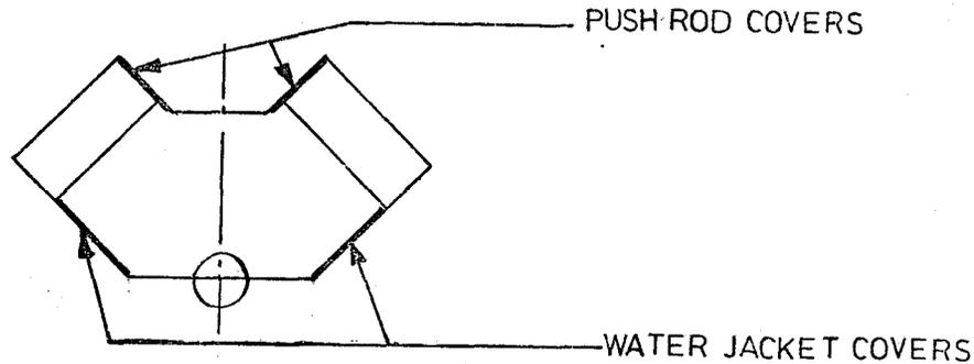
(e) Water jacket covers (see sketch). These were made of double skin damped panels bonded together at the fixing flange, thus also providing vibration isolation.
