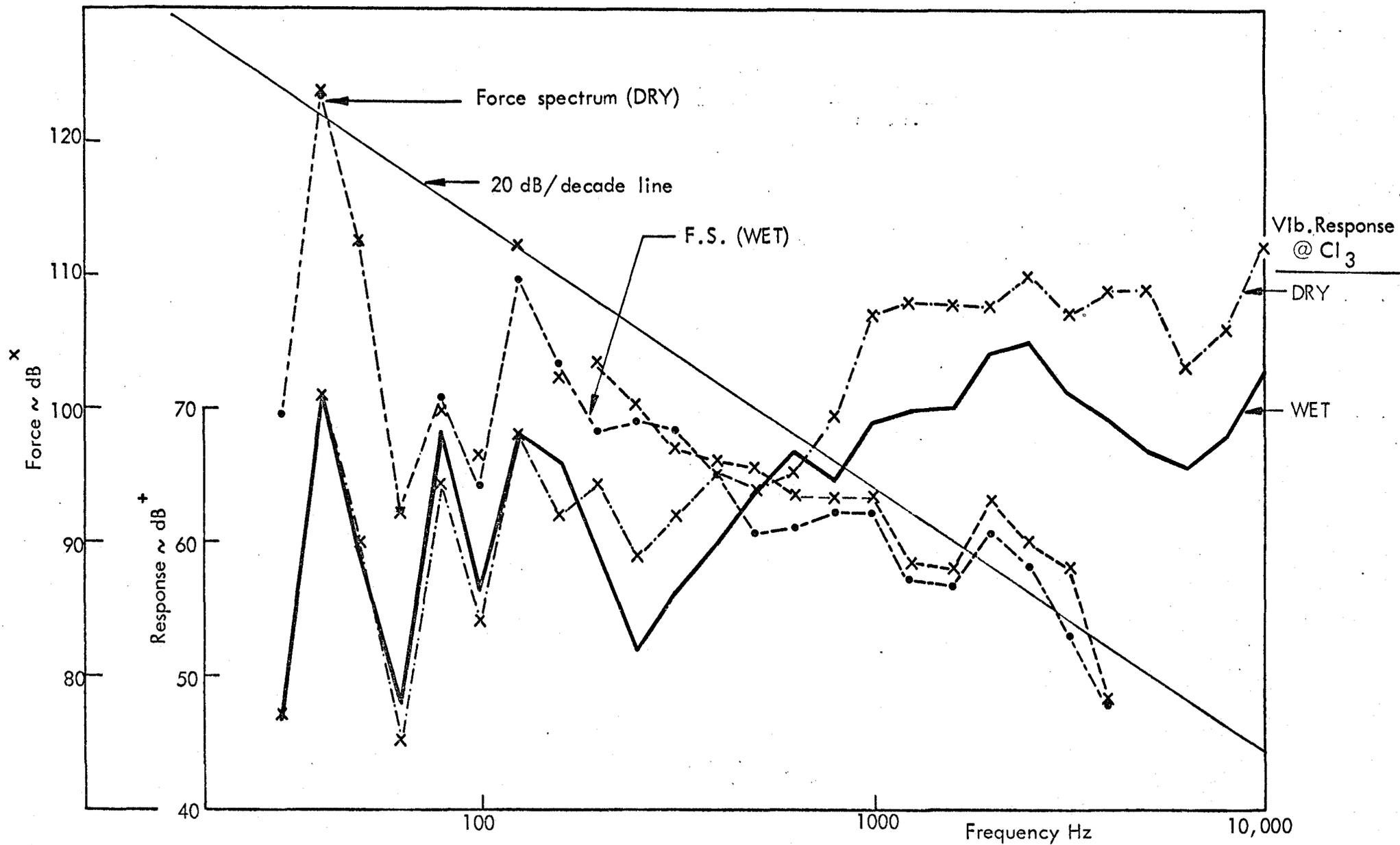
FIG. 5.30d TYPICAL EFFECT OF OIL FILM ON THE VEE RIG AT REPETITION RATE 41.7 per sec.—STANDARD PISTONS OF SA
