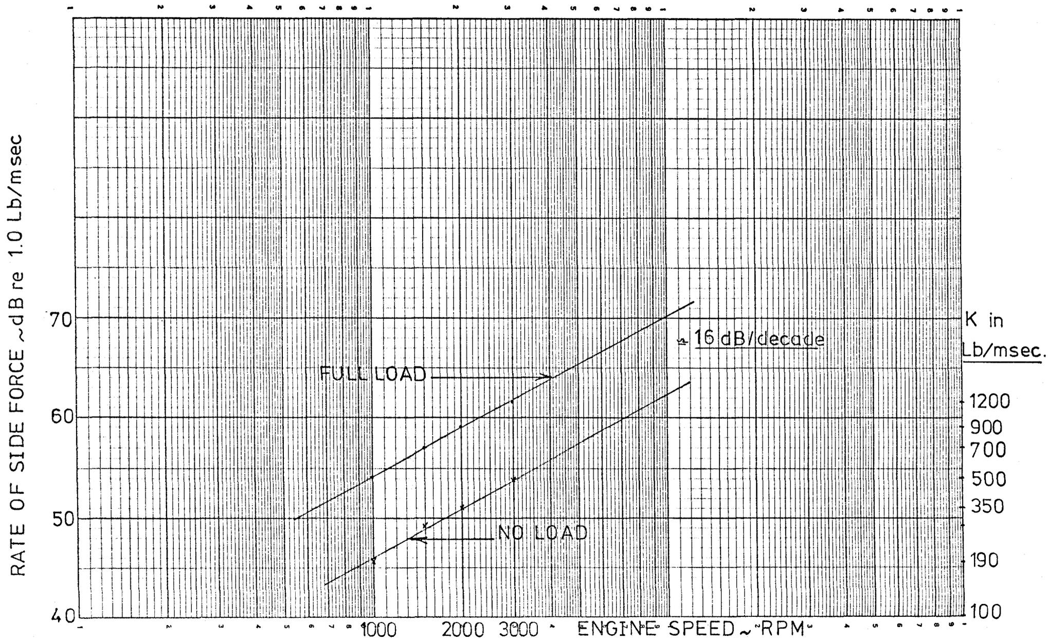
FIG. 5.28 RELATION BETWEEN 'K' FACTOR AND ENGINE SPEED - ENGINE SA
