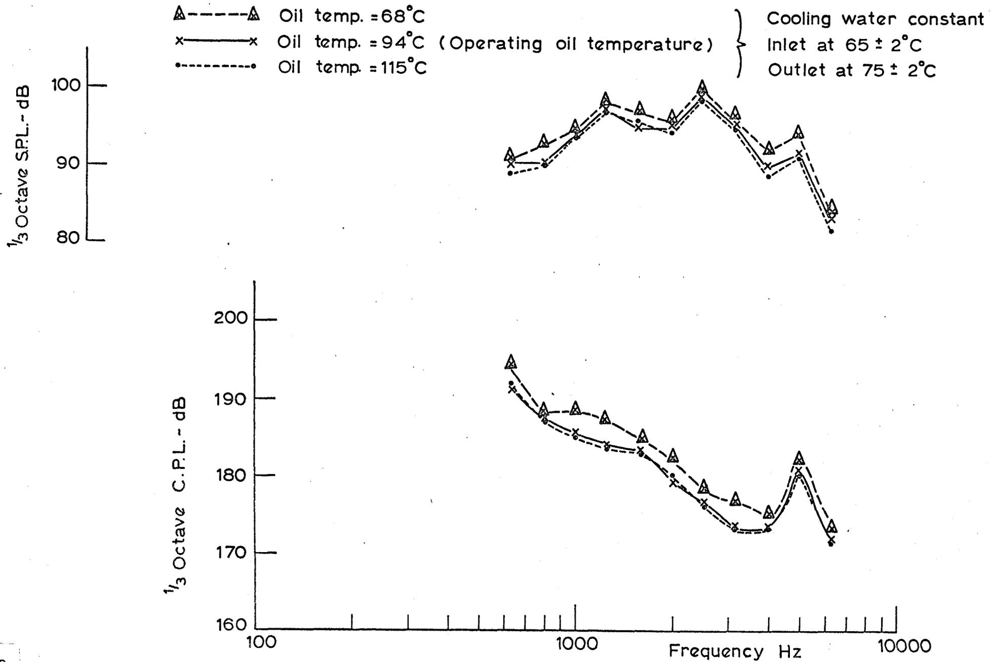
Fig. 3.8 Variation of cylinder pressure and noise spectra with change of oil temperature for the SA engine at 3000 r.p.m. full load.
