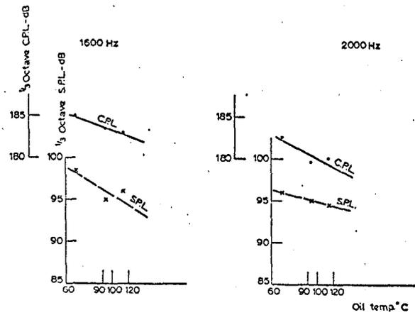
FIG. 3.9b Variation of cylinder pressure and noise with oil temperature for the standard engine at 3000 r.p.m. full load - 1600 and 2000 Hz.
