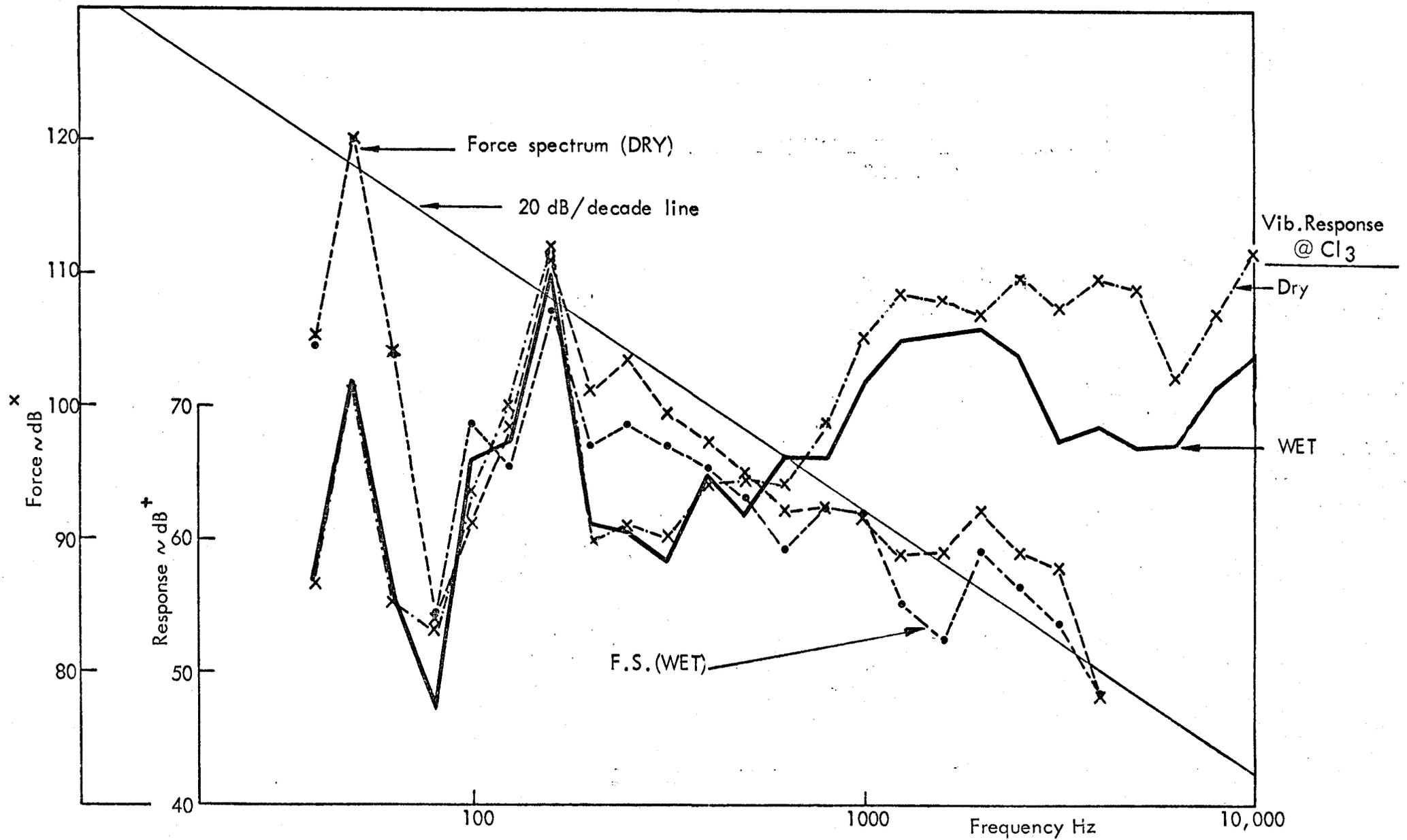
FIG. 5.30 e TYPICAL EFFECT OF OIL FILM ON THE RIG AT REPETITION RATE 50 per sec. — STANDARD PISTONS OF SA
