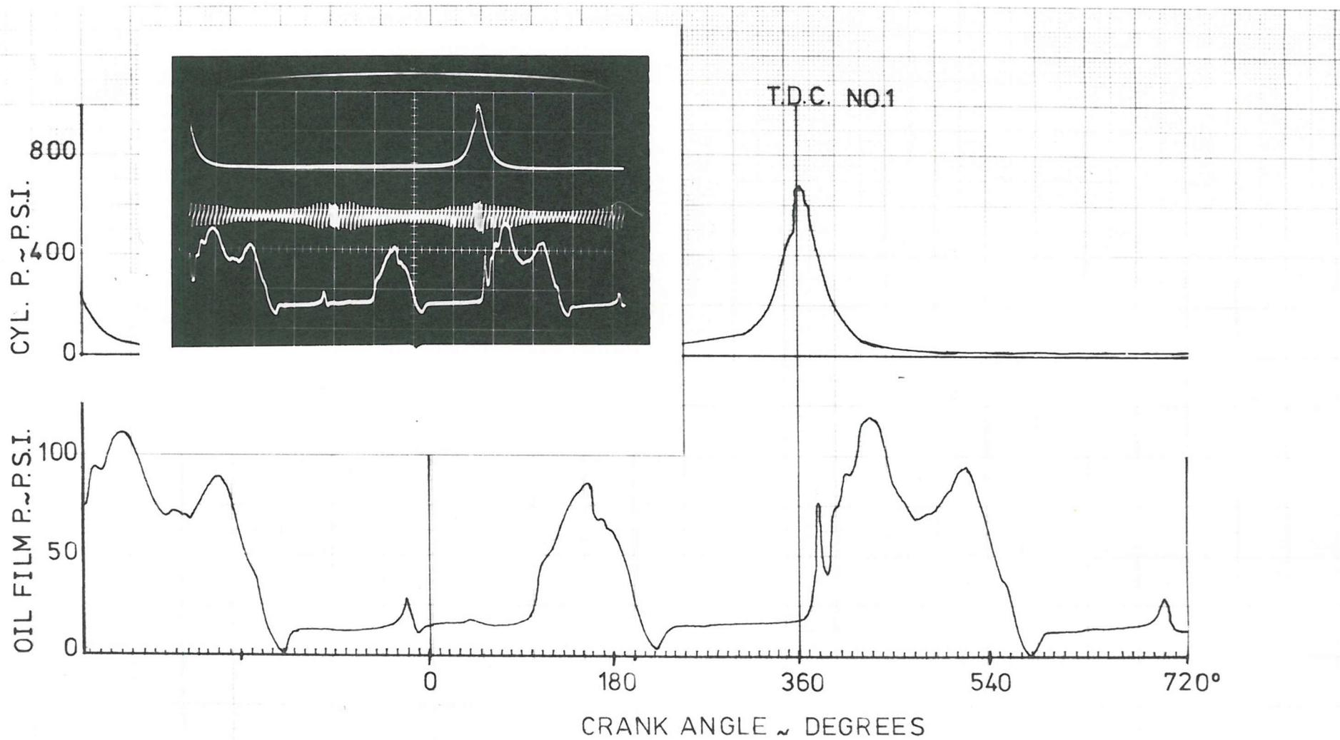
FIG. 7.5 CYLINDER PRESSURE AND PISTON TO BORE OIL FILM PRESSURE (THRUST SIDE) AT 1500 RPM NO LOAD - SA ENGINE
