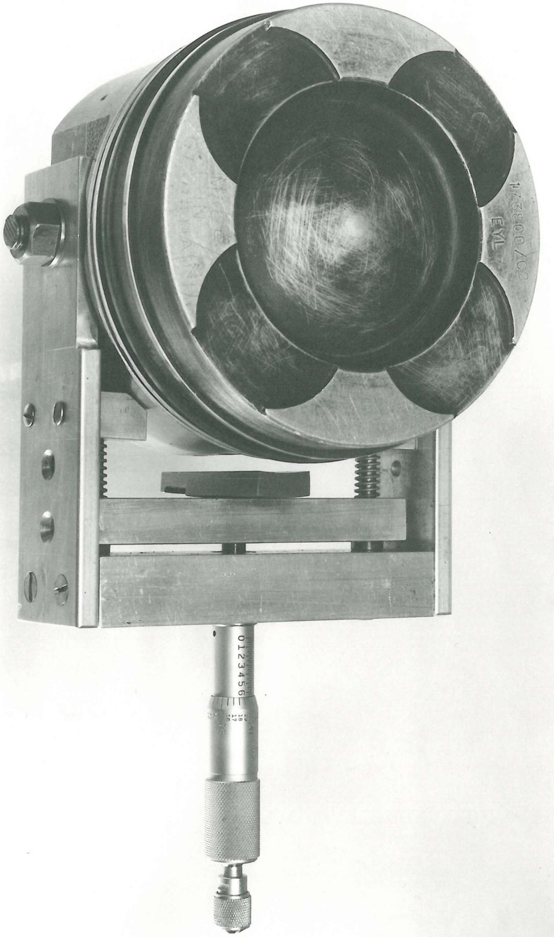
FIG. 4F RIG FOR CALIBRATING T4 GAUGES IN SITU
