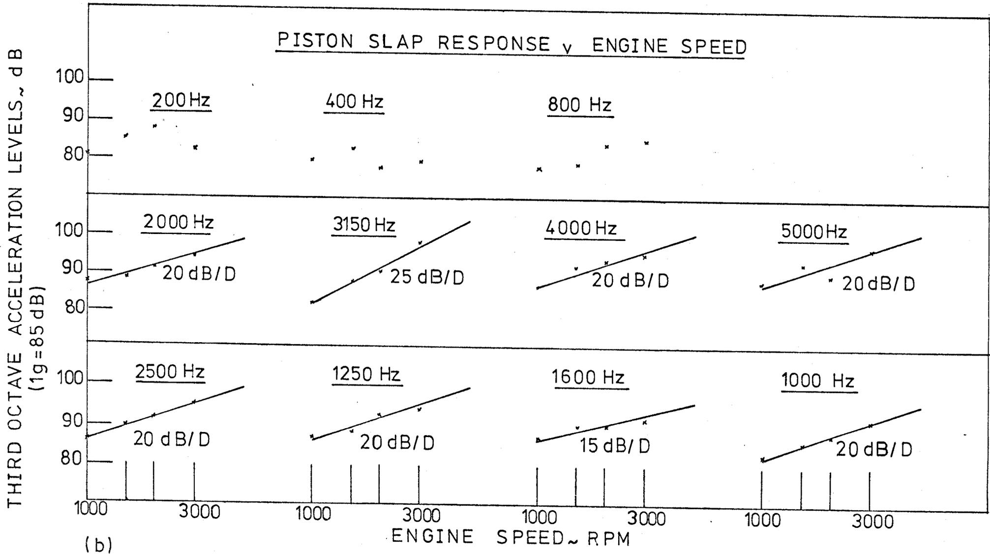
FIG. 5.27 CHARACTERISTICS OF PISTON SLAP INDUCED VIBRATION AND ITS RELATION WITH ENGINE SPEED — FULL LOAD
