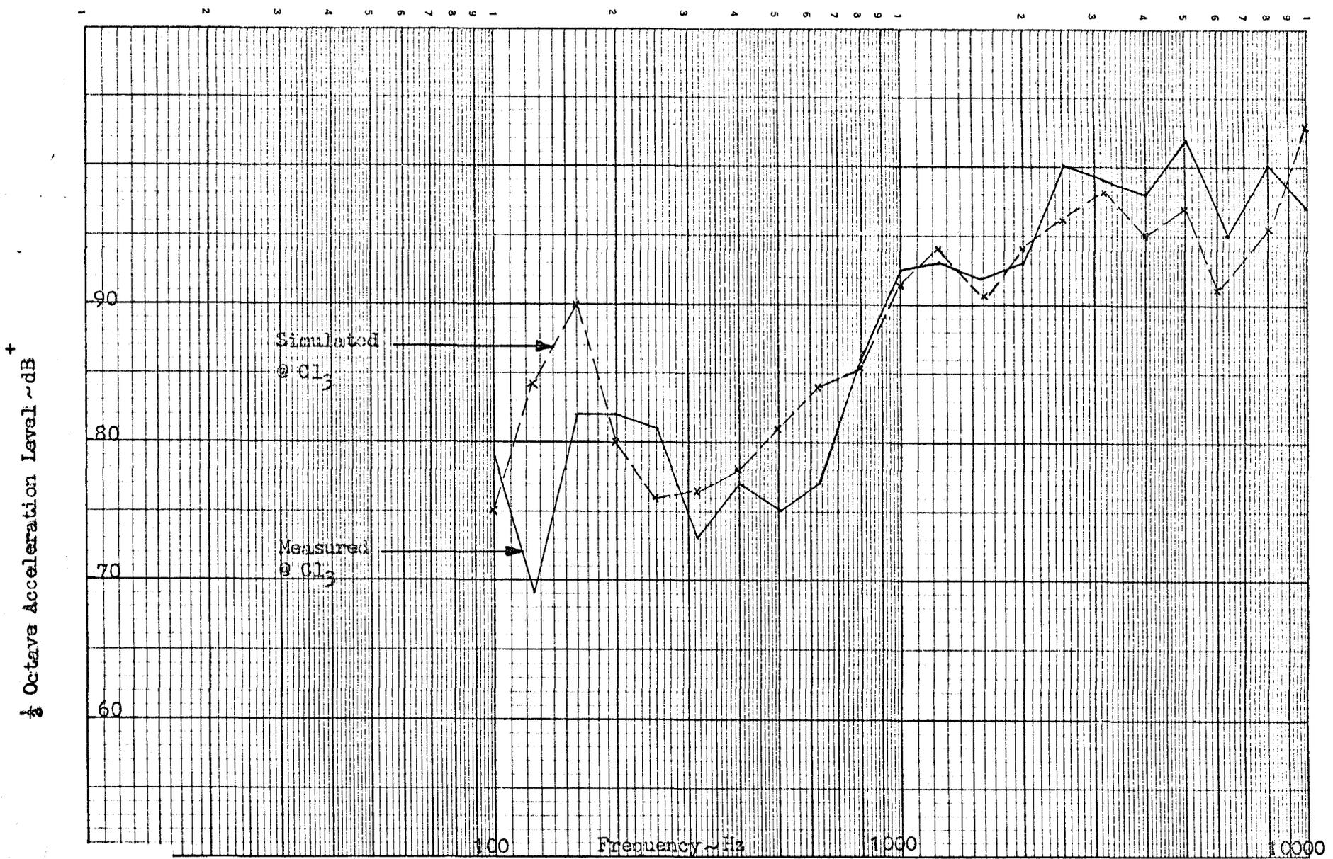
FIG. 5.26 Comparison of measured vibration @ Cl<sub>3</sub> and that simulated through the piston slap rig at Full Load
