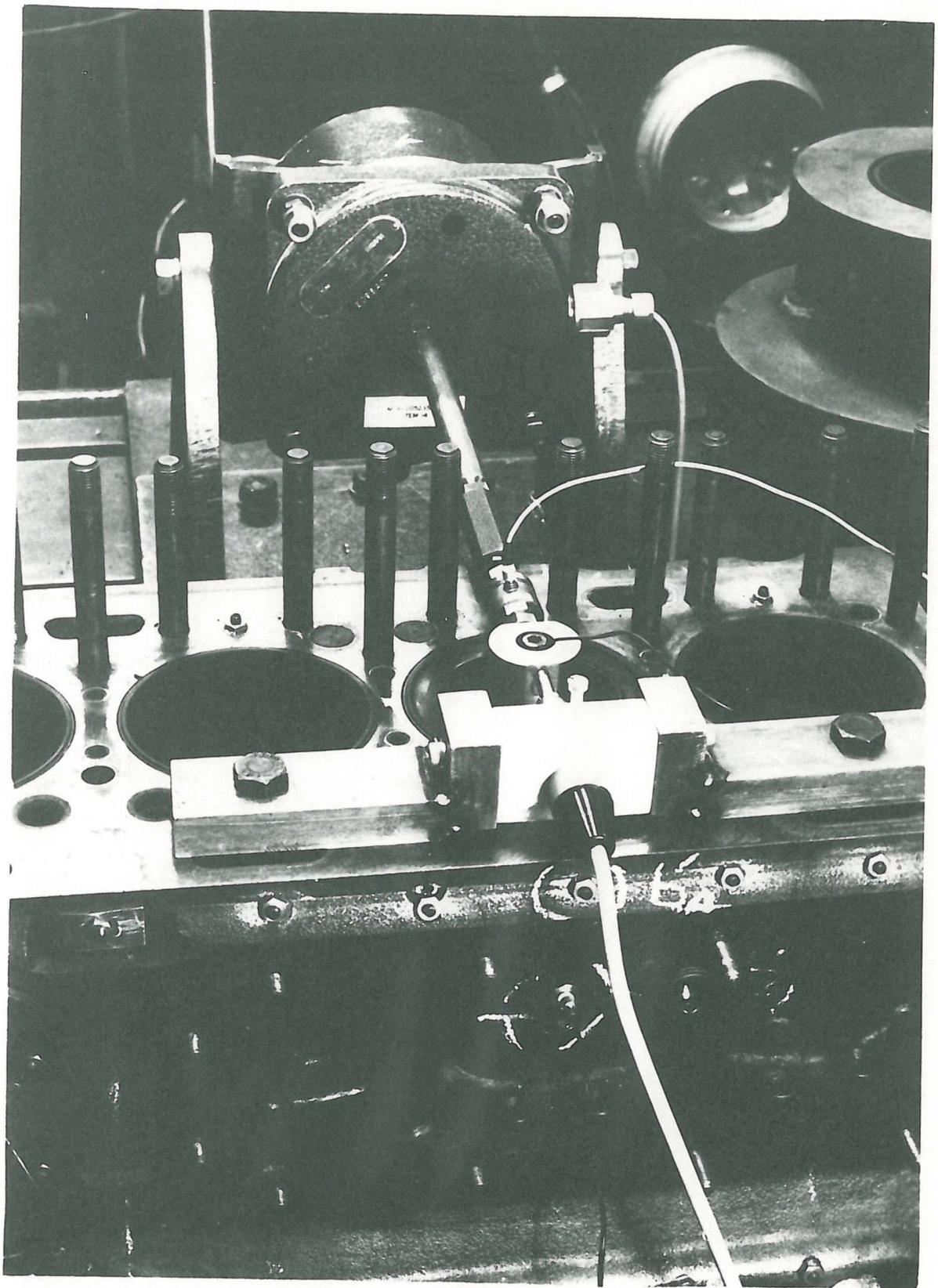
Close up of the InLine 6 Piston Slap Rig.
