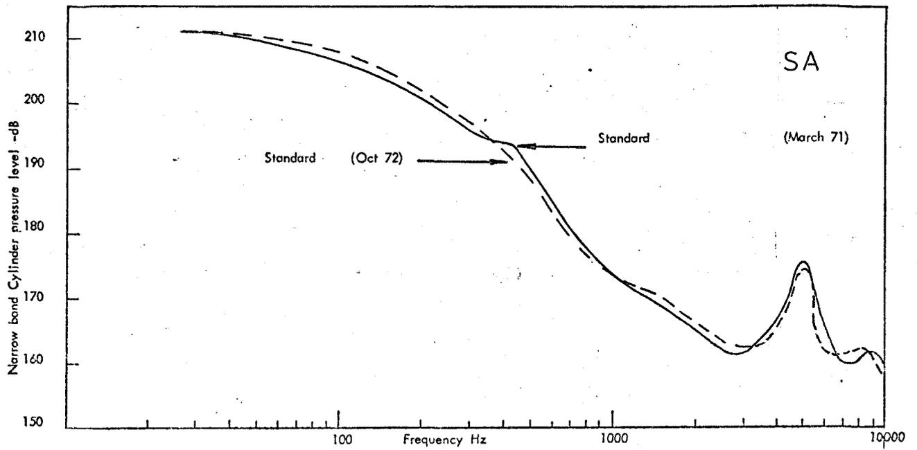
FIG. 4.24 COMPARISON OF CYLINDER PRESSURE SPECTRA FOR THE SAME MAKE AND TYPE OF ENGINE TESTED UNDER NEARLY IDENTICAL CONDITIONS @ 3000 r.p.m. FULL LOAD.
