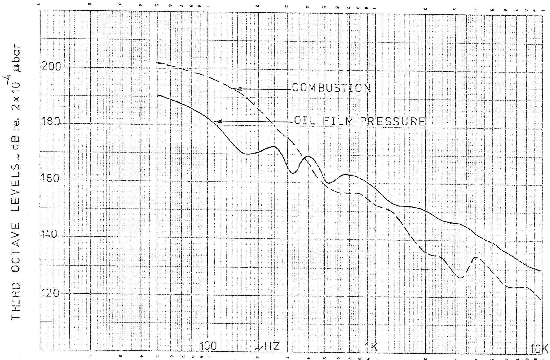
FIG. 7.21 SPECTRA OF PISTON TO BORE OIL FILM PRESSURE AND COMBUSTION FOR SA ENGINE AT 2000 RPM NO LOAD
