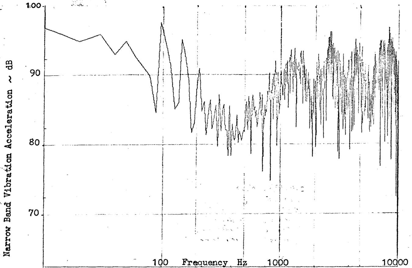
FIG. 2C Vibration Acceleration Response at  $Cl_3$  due to Slapping Pulses in a running V8-470 Diesel Engine at 2000 r.p.m. Full Load.
