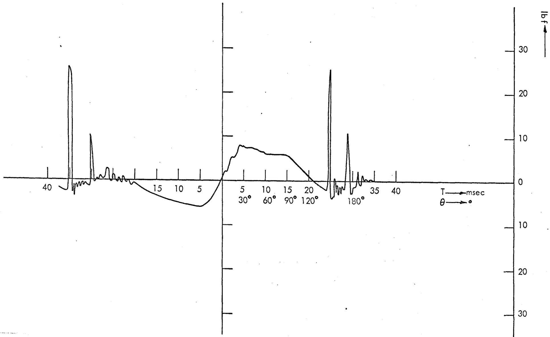
FIG. 5.4 ACTUAL PISTON SIDE FORCE USED TO SIMULATE PISTON SLAP AT 16.7 Hz.
