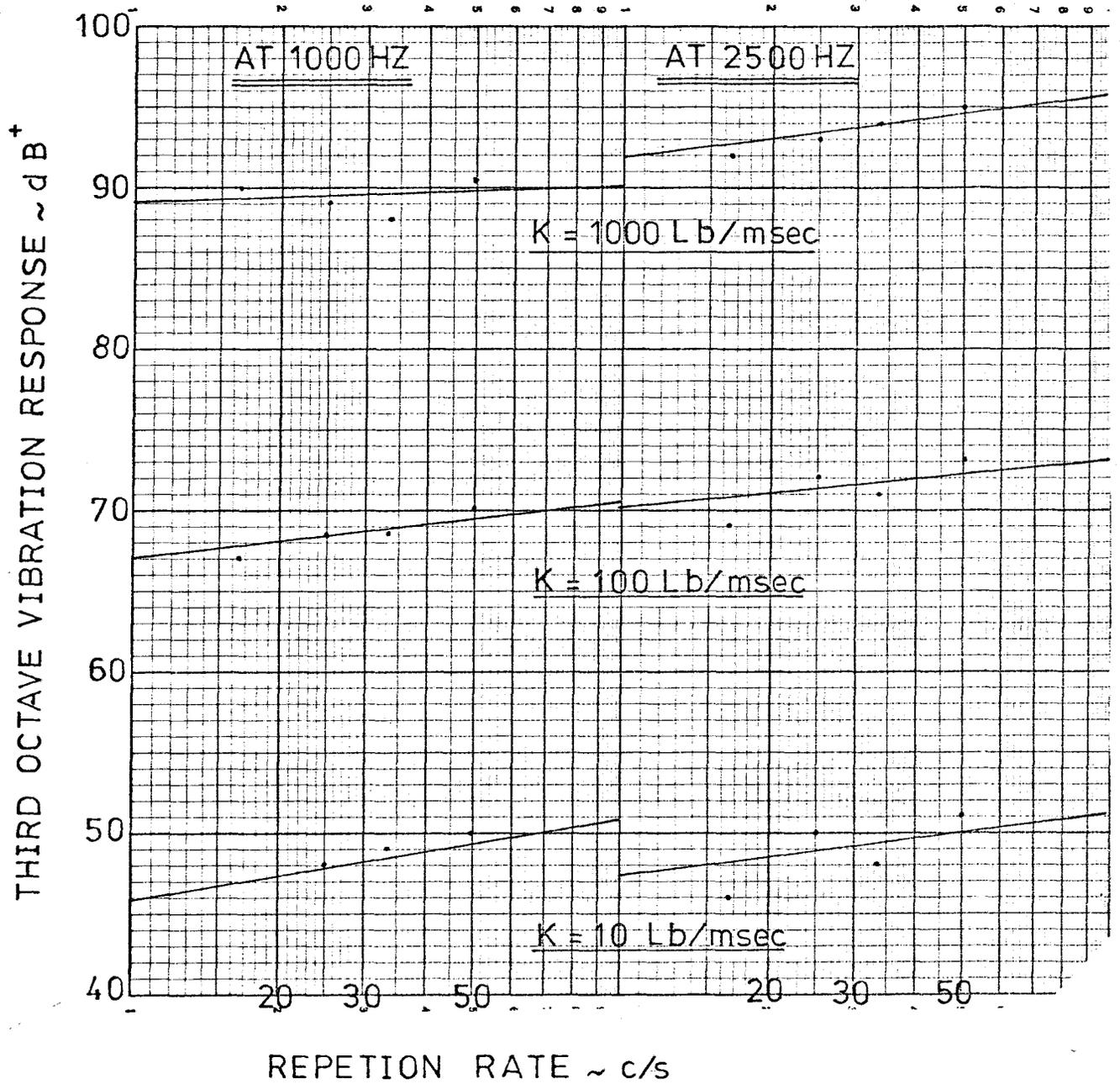
FIG. 5.29 RELATION BETWEEN VIBRATION RESPONSE AT  $Cl_3$  AND PISTON SLAPPING RATE FOR CONSTANT K FACTORS AT TWO TYPICAL THIRD OCTAVE FREQUENCY BANDS
