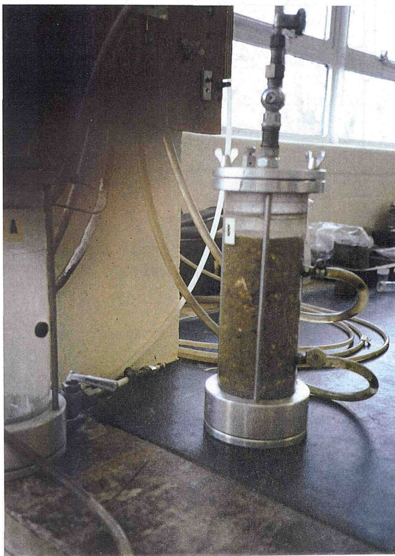
Plate 4.5 Equipment used for hydraulic conductivity tests
