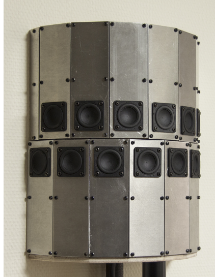
FIGURE 7.12: Prototype of a HCA with r_S = 14.2 cm and L = 15 Tang Band W1-1070SG full-range drivers.
