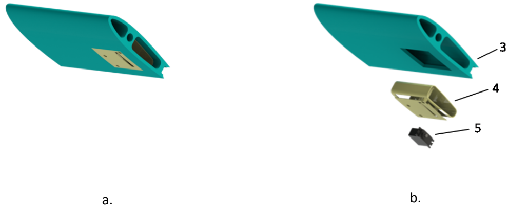
Figure 5-20 – Part of the subassembly of the tailplane of DECODE-2. a. Collapsed view b. Exploded view.
