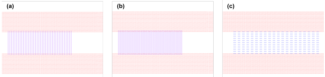
FIGURE 4.8: Implementation of the grating couplers over 10 \mu\text{m} -wide waveguides, for (a) \lambda = 1.55 \mu\text{m} , (b) \lambda = 1.95 \mu\text{m} and (c) \lambda = 3.80 \mu\text{m} . The red features show the ESM grating cladding, the purple features show the 250 nm etched gratings and the blue features show the 500 nm etched gratings.
