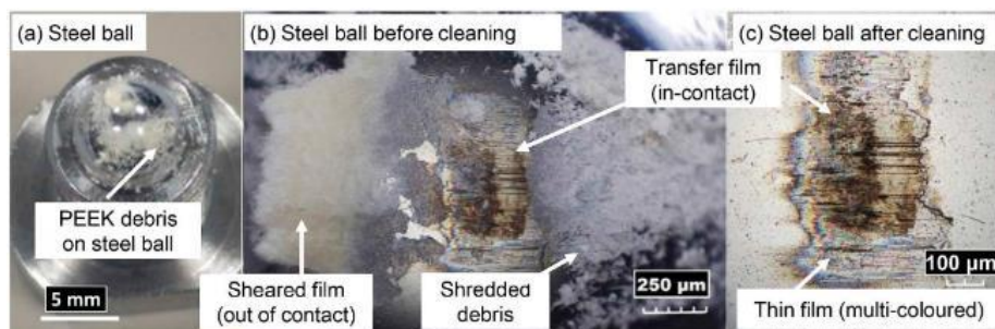
Figure 2.21. Appearance of PEEK transfer film formed on the steel ball (adapted from [90])
