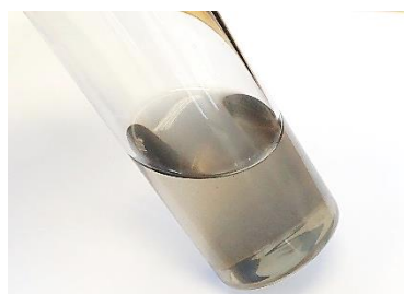
Figure 6.12. PAO4 oil containing CFR PEEK wear debris
