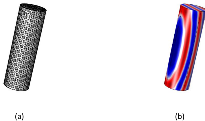
Figure 4-26 The meshed BE model (a) and the surface pressure distribution (b) at the frequency of 1000 Hz.
