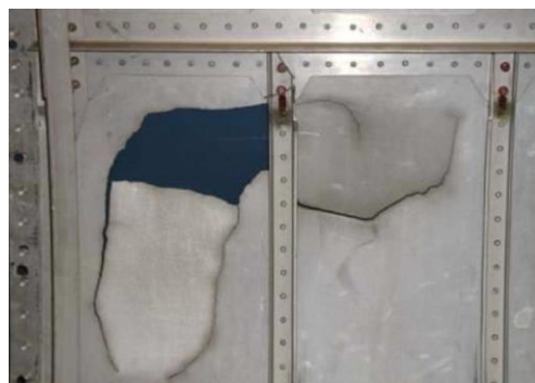
Figure 1-1 A cracked panel due to acoustic fatigue [1].
