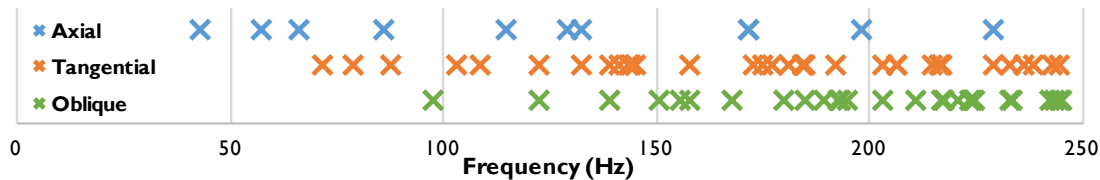
Figure 2-11. Example room natural frequencies (cuboid shaped room, 4 x 3 x 2.6 m)
