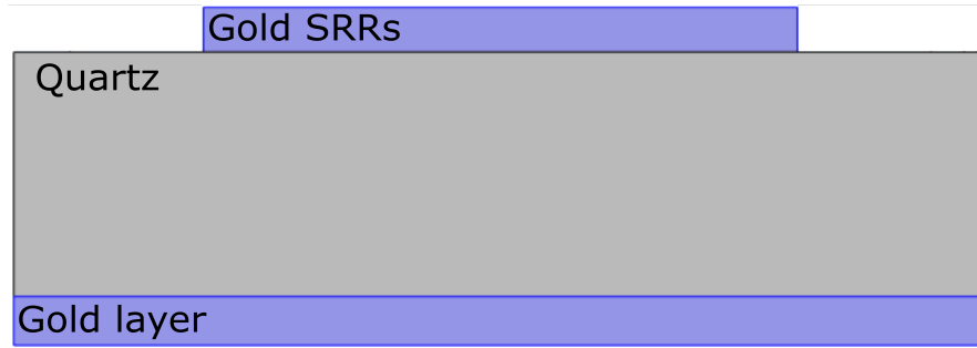
FIGURE 2.4: The structure on which the SRRs will be deposited via thermal deposition . The SRRs sit atop a substrate which separates the SRRs and the Gold layer.
