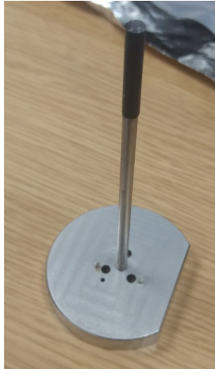
Figure 4.7: Experimental setup for mounting the lithium iron phosphate electrode sample.
