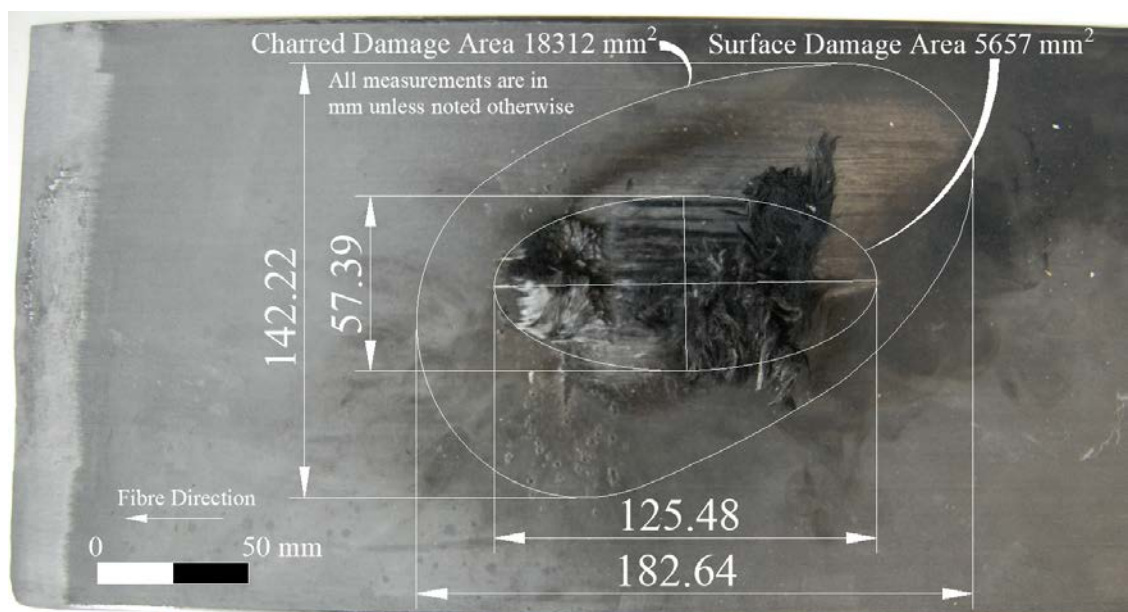
Figure A.20: Visual inspection of damaged specimen AE3-4 struck
