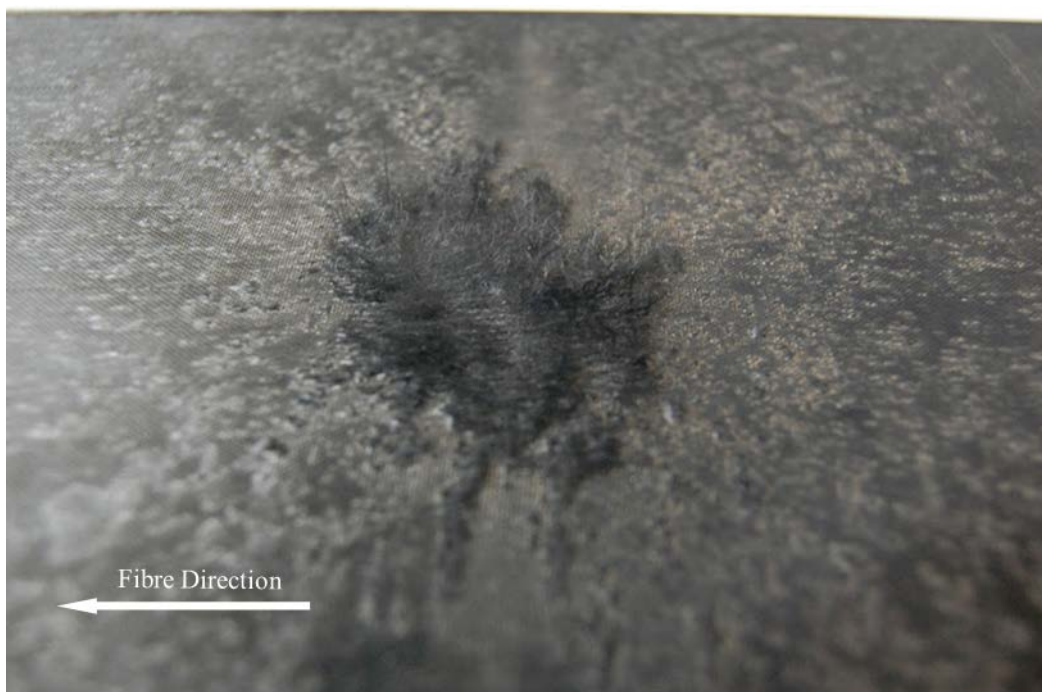
Figure 4.40: Close-up image of charring damage from specimen AE2-4 taken using Nikon DSLR with 50 mm lens
