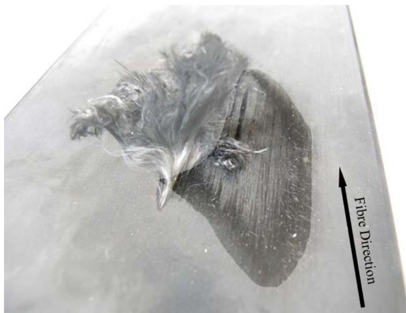
Figure 4.39: Close-up image of the area with resin burn off in specimen AE3-4 taken using Nikon DSLR with 50 mm lens. Undamaged area is shaded.
