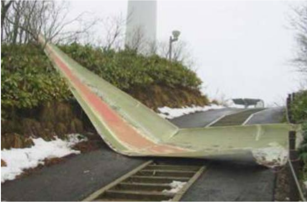
Figure 2.22: The remainder of a blade detached from a wind turbine due to lightning damage [75]
