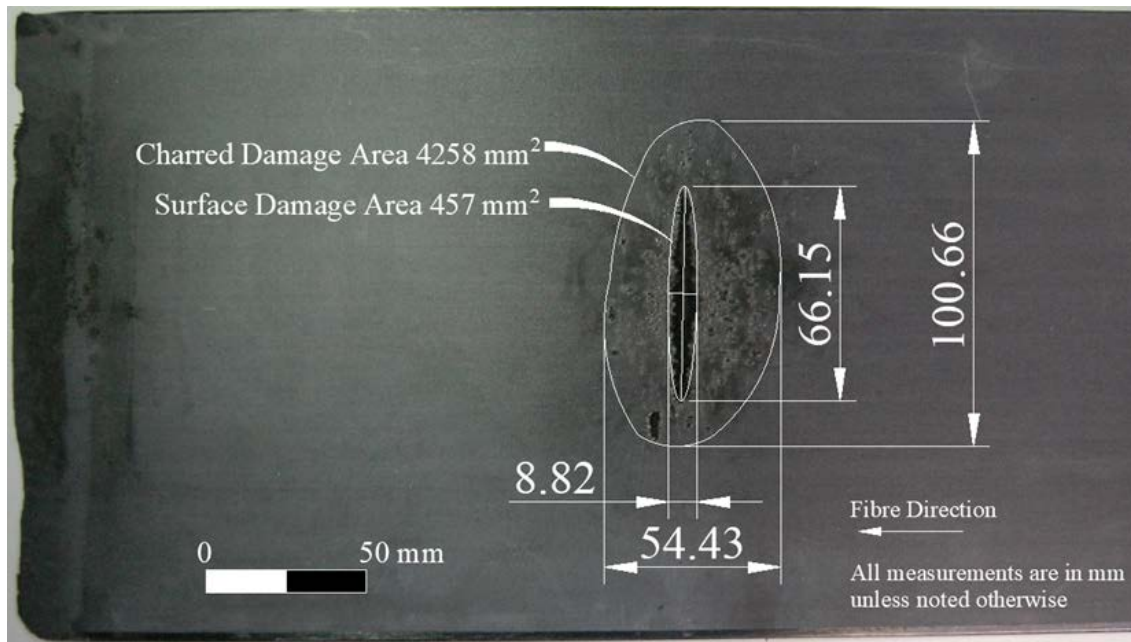
Figure A.12: Visual inspection of damaged specimen from AE2-4 struck with oscillating waveform
