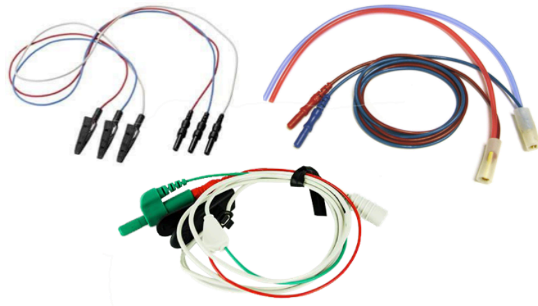
Figure 5.2: Three types of leads used during experiments: alligator clip for mastoid pad (top left), tiptrode lead combined with delivery tube (top right), wick electrode leads (bottom)
