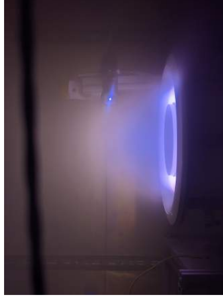
(b) The BN500 Hall thruster during krypton testing in the large vacuum chamber.
