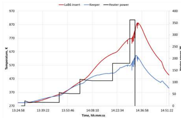
Fig. 7 Thermocouple data for preliminary heater tests of the G100 without the internal BN heat shield. Minor noise can be seen on the thermocouple readings, this occurred when slight arcing occurred within the chamber and effected the thermocouple reading.
