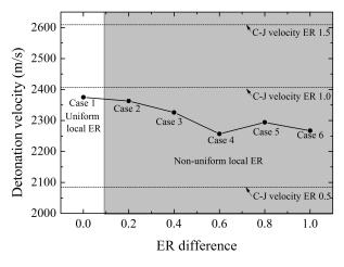
Figure 6: Average detonation velocity computed from the pressure profiles from 0.6 ms to 0.9 ms.
