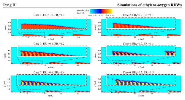
Figure 3: Pseudo-color images of local equivalence ratio (ER) under different injections.
