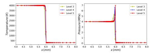
Figure 2: Temperature and pressure profiles of 1-D ethylene/oxygen detonation front.
