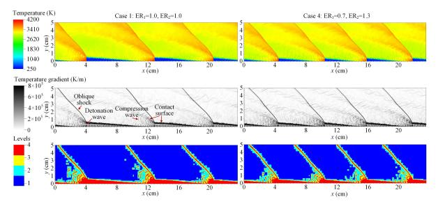
Figure 4: Pseudo-color images of temperature, temperature gradient and refinement level distribution under different injections.
