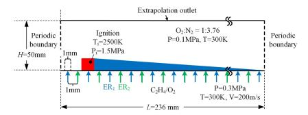
Figure 1: 2-D computational domain of the ethylene/oxygen RDE simulations.
