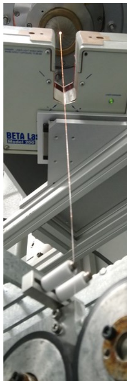
Figure 64. Fibre drawing process of the 3D printed silica preforms.
