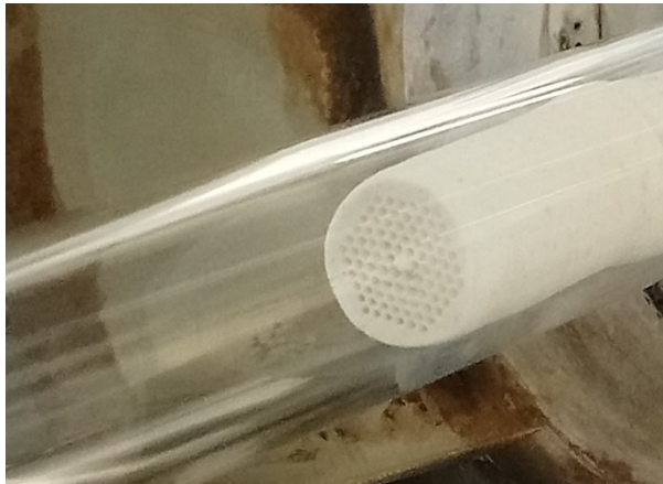
Figure 61. Fibre drawing conditioning of 3D printed silica preforms.
