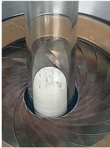
Figure 63. 3D printing preform set in fibre drawing furnace.
