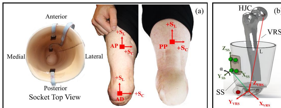
11 Figure 2: (a) Sensor placement on the inner socket wall and the corresponding locations on the 12 residuum (b) An illustration to define virtual residuum segment (VRS), socket segment (SS), angular 13 coupling (α) and pistoning (L).
