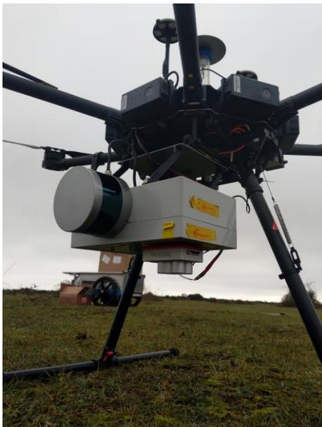
Figure 3-2 The components of the sensor package assembled within a lightweight plastic box for testing, here mounted on a DJI M600 multirotor platform.
