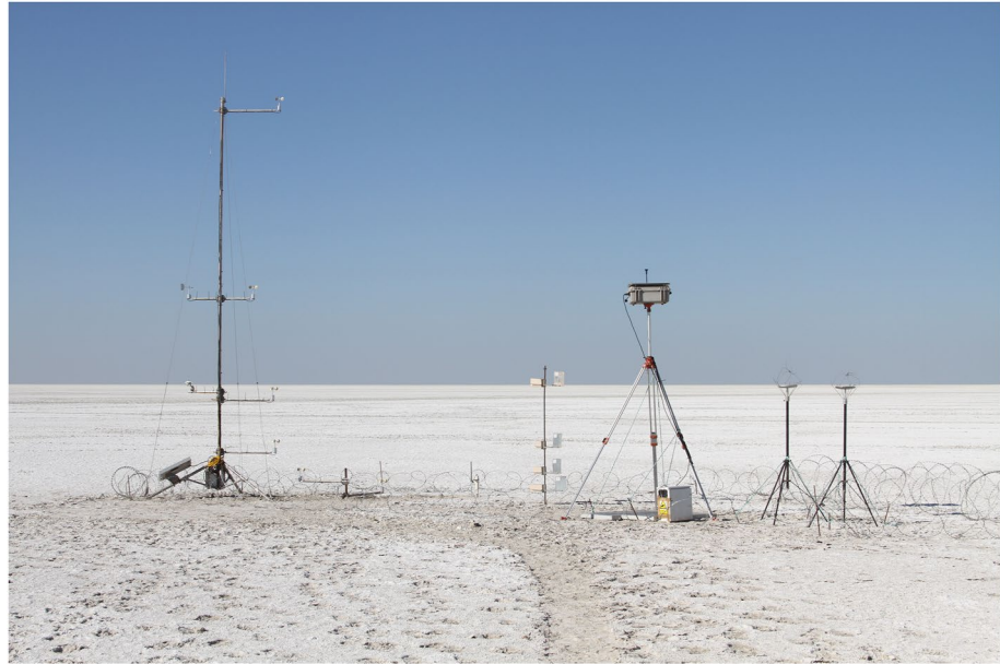
Figure 2. A typical monitoring station (Pan Road) showing a 6 m anemometer tower on the left and a TSI DustTrak DRX aerosol monitor on the tripod in the center-right. All instrument data were logged at an interval of 10 min.
