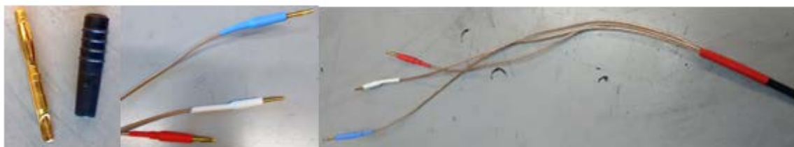
Figure 2-4 Photographs of the specially designed cables showing the banana plug (left), FEP coated coaxial cables with banana plugs connected (middle) and the completed cable assembly (right).
