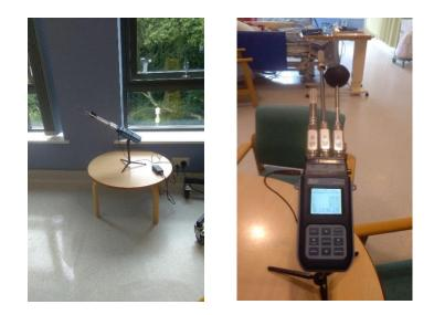
**Figure 21.** Location of Delta OHM WBGT monitor used to measure thermal comfort in the study wards over a pre-intervention (22<sup>nd</sup> August 2017) and a post intervention (2<sup>nd</sup> April 2018) period during the study
