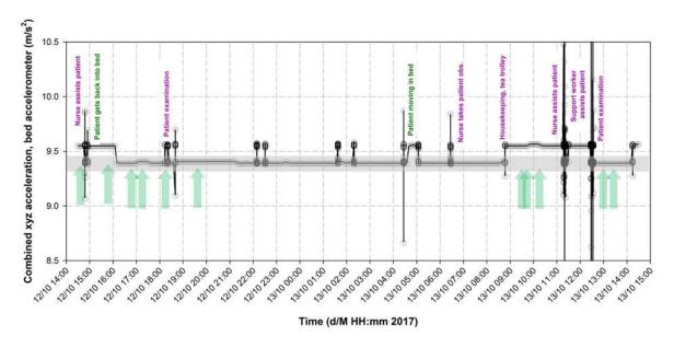
**Figure 38.** Quantitative bed movement data on Bed 3 with combined acceleration (xyz) forces (m/s<sup>2</sup>) shown against qualitative observed bed events for Bed 3 in an older-persons' community hospital ward during a 24-hour study pilot from 14:30:00 12<sup>th</sup> October 2017 until 14:30:00 13<sup>th</sup>
