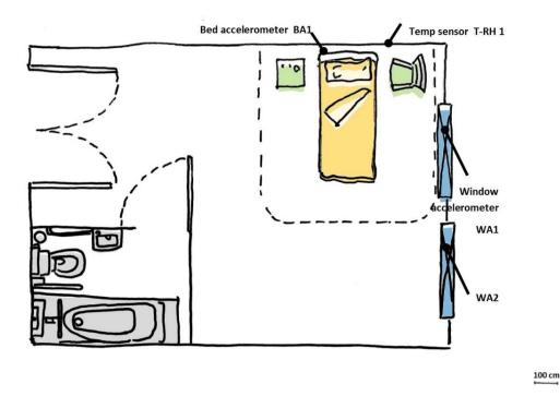
Figure 25. Single room layout and location of the monitoring equipment used during the study
