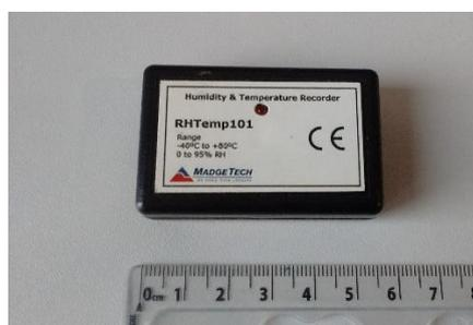
**Figure 19.** MadgeTech RHTemp101 logger used to measure air temperature and relative humidity in the control and intervention study wards during the study (1<sup>st</sup> August 2017 - 30<sup>th</sup> April 2018)
