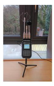
**Figure 20.** Delta OHM WBGT monitor used to measure thermal comfort in the control and intervention study wards over a pre-intervention (22<sup>nd</sup> August 2017) and a post intervention (2<sup>nd</sup> April 2018) period during the study
