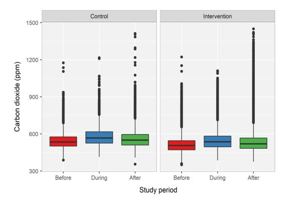
**Figure 69.** Boxplot of minutely CO<sub>2</sub> values (ppm), comparing the control and intervention study groups for the study periods before (1<sup>st</sup> August - 31<sup>st</sup> October 2017), during (1<sup>st</sup> November 2017 - 31<sup>st</sup> January 2018) and after (1<sup>st</sup> February - 30<sup>th</sup> April 2018) the behaviour change intervention
