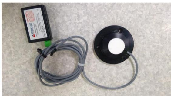
**Figure 17.** Unbranded silicon photodiodes and data logger used to measure light in the control and intervention study wards during the study (1<sup>st</sup> August 2017 - 30<sup>th</sup> April 2018)
