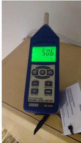
**Figure 18.** Reed SD4023 sound monitor used to measure noise levels (dB) in the control and intervention study wards during the study (1<sup>st</sup> August 2017 - 30<sup>th</sup> April 2018)
