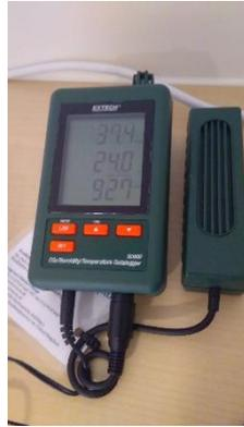
**Figure 22.** Extech SD800 CO<sub>2</sub> monitor used to measure carbon dioxide (CO<sub>2</sub>) in the study wards during the study (1<sup>st</sup> August 2017 - 30<sup>th</sup> April 2018)
