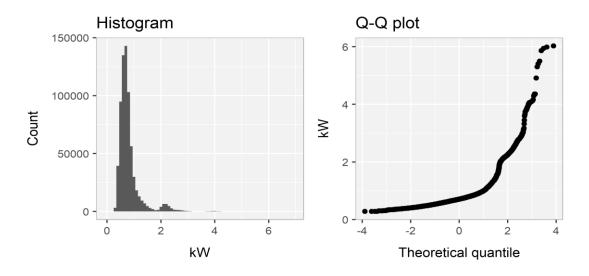
**Figure 47.** Histogram and Q-Q plot showing the total power demand values for small power for the combined control and intervention study groups for the study period of 1<sup>st</sup> September 2017 to 30<sup>th</sup> April 2018
