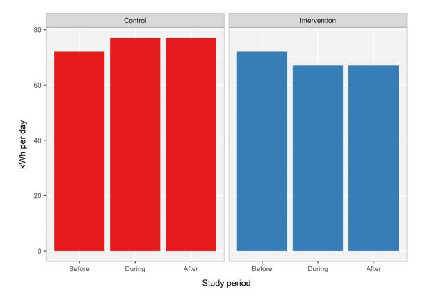
Figure 87. Total energy consumption per day (kWh/day) for lighting and small power, comparing the control and intervention study groups for the study periods before (1<sup>st</sup> September - 31<sup>st</sup>
