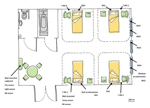
**Figure 26.** Four-bed multi-occupancy room layout and location of the monitoring equipment used during the study
