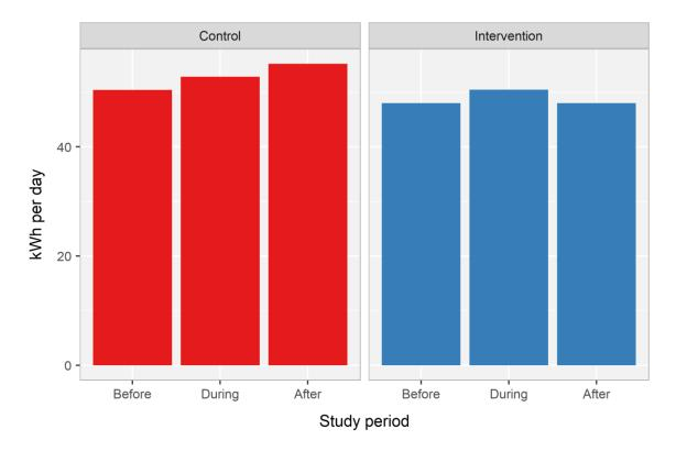
**Figure 52.** Energy consumption per day (kWh/day) for small power, comparing the control and intervention study groups for the study periods before (1<sup>st</sup> September - 31<sup>st</sup> October 2017), during (1<sup>st</sup> November 2017 - 31<sup>st</sup> January 2018) and after (1<sup>st</sup> February - 30<sup>th</sup> April 2018) the behaviour change intervention
