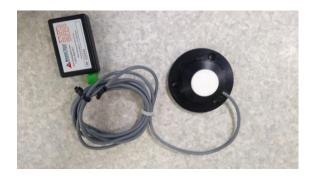
**Figure 17.** Unbranded silicon photodiodes and data logger used to measure light in the control and intervention study wards during the study (1<sup>st</sup> August 2017 - 30<sup>th</sup> April 2018)
