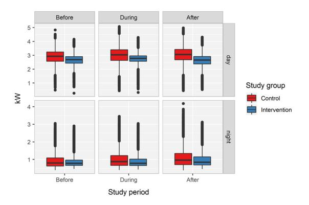
**Figure 42.** Box plot of day and night time minutely power demand values (kW) for lighting, comparing the control and intervention study groups for the study periods before (1<sup>st</sup> September -31<sup>st</sup> October 2017), during (1<sup>st</sup> November 2017 - 31<sup>st</sup> January 2018) and after (1<sup>st</sup> February - 30<sup>th</sup> April 2018) the behaviour change intervention
