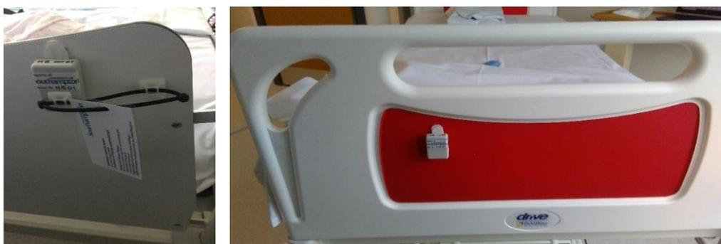
**Figure 24.** 3-axis accelerometer shown on (1) a standard bed (left) and (2) a falls bed (right) used to measure patient bed movements in the control and intervention study wards during the study (1<sup>st</sup> August 2017 - 30<sup>th</sup> April 2018)
