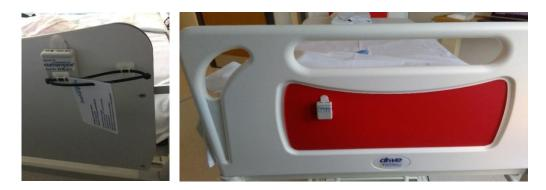
**Figure 24.** 3-axis accelerometer shown on (1) a standard bed (left) and (2) a falls bed (right) used to measure patient bed movements in the control and intervention study wards during the study (1<sup>st</sup> August 2017 - 30<sup>th</sup> April 2018)
