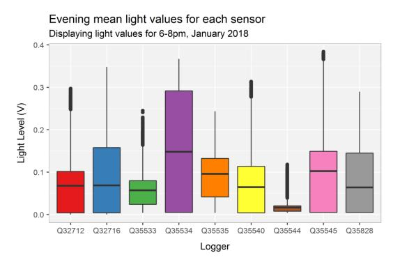
Figure 2: Mean light voltage level for each sensor
