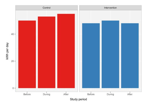
**Figure 46.** Energy consumption per day (kWh/day) for lighting, comparing the control and intervention study groups for the study periods before (1<sup>st</sup> September - 31<sup>st</sup> October 2017), during (1<sup>st</sup> November 2017 - 31<sup>st</sup> January 2018) and after (1<sup>st</sup> February - 30<sup>th</sup> April 2018) the behaviour change intervention
