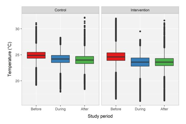
**Figure 59.** Boxplot of 5 minutely air temperature values (<sup>o</sup>C), comparing the control and intervention study groups for the study periods before (1<sup>st</sup> August - 31<sup>st</sup> October 2017), during (1<sup>st</sup> November 2017 - 31<sup>st</sup> January 2018) and after (1<sup>st</sup> February - 30<sup>th</sup> April 2018) the behaviour change intervention
