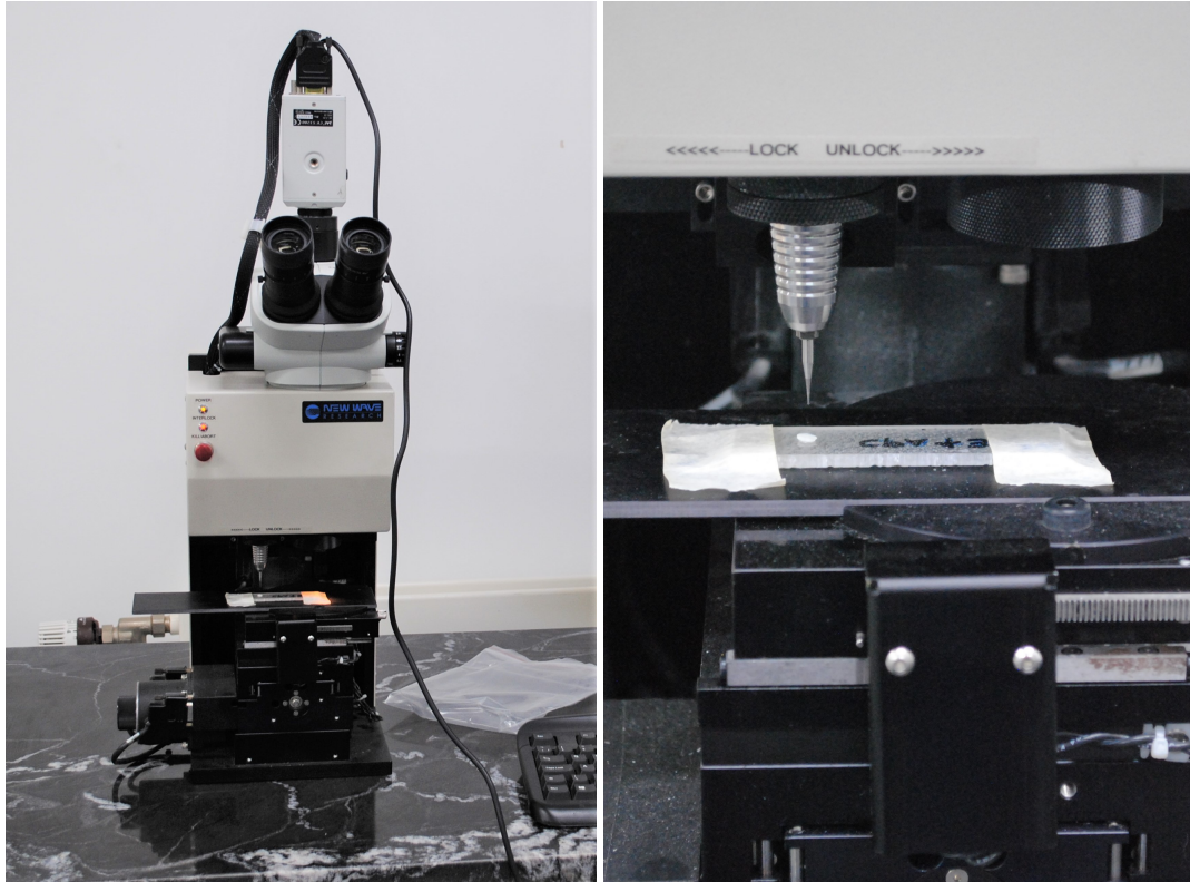
FIGURE 2.5: Top left shows the otolith milling setup, using an ESI New Wave Micromill. Top right shows how mounted otoliths were affixed to the Micromill stage, using masking tape. The drill bit mounted is flat edged with a cut width of 900\ \mu\text{m} .
