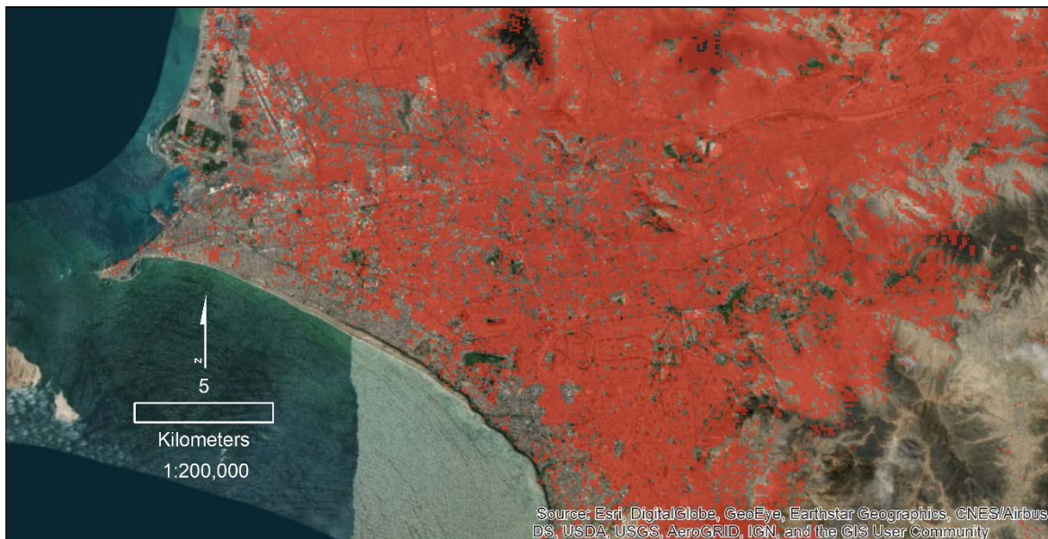
Figure 2 Example of GHSL built-settlement extent data (red) in Lima, Peru where a part of the city pre-existing 1975 was not captured (south west coast). The artefact of the image tile extents where there were issues (e.g. atmospheric, sensor, etc.) is also apparent.
