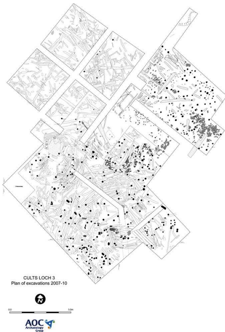
Figure A.1.1 Plan of the piles (dark spots) and timbers (elongate outlines) indicating the structure of the promontory crannog in Cults Loch. Courtesy of AOC Archaeology.
